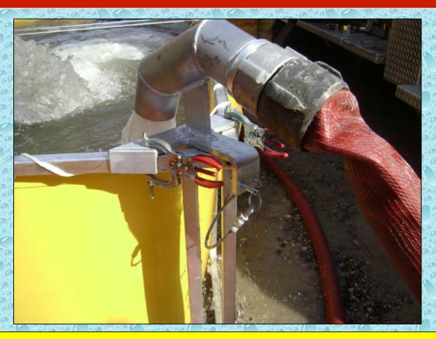
The floating portable pump discharges water into the primary drafting tank using the attachment shown above.
