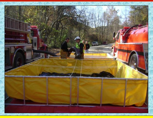
A second dump tank is deployed around the 9:27-minute mark and crews work to set a water transfer device.
