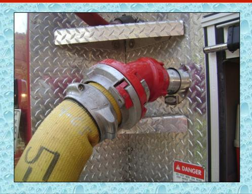
The 1,250 gpm draft pumper could not support a flow much above 1,000 gpm for a couple of reasons. Perhaps the main reason was the flow capability of the rear discharge. Had two discharges been used to feed the 5-inch LDH line to the Hose Monster, then the pumper most likely could have discharged a higher volume.
