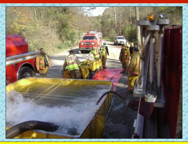
With more tankers arriving, crews prepare to set-up a third dump tank in hopes of moving to a 1,000 gpm flow.
