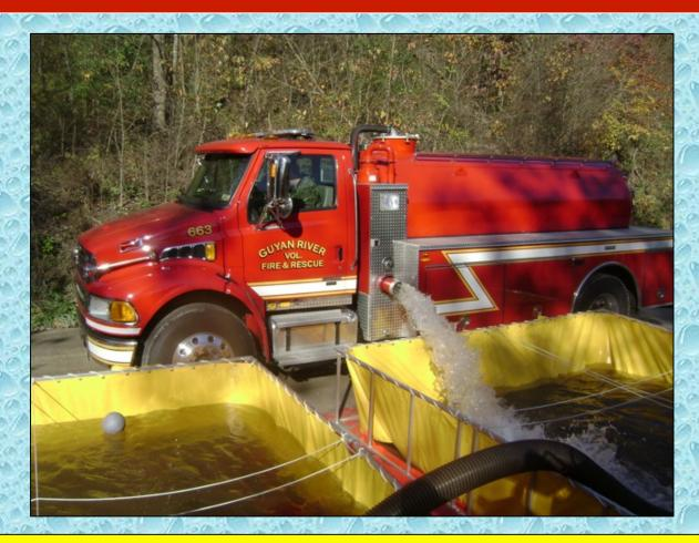
Guyan River Tanker 663 dumps is 2,000 gallons of water while crews work to expand the dump site.
