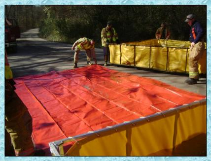
Crews change the location of the 3<sup>rd</sup> dump tank prior to it being filled with water. The decision was based on using a 3-tank arrangement and drafting out of the center tank as opposed to drafting out of the end tank. It is important to make these changes early because once a tank is filled with water, it normally does not get moved.
