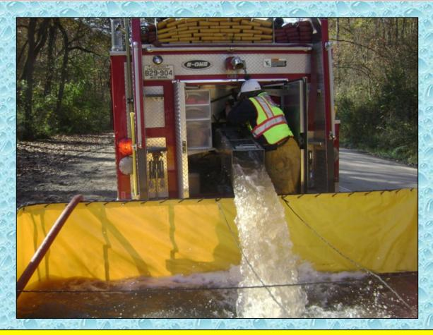
As additional tankers arrive, they have to be positioned so that they don't impede the operation of other tankers.
