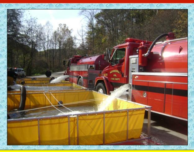
At the 87:00 minute mark, with four dump tanks in operation, the flow was moved to 1,000 gpm where it was sustained for the remainder of the drill.
