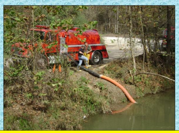
This 2,000-gallon vacuum tanker loads very quickly and will soon be on its way back to the dump site.
