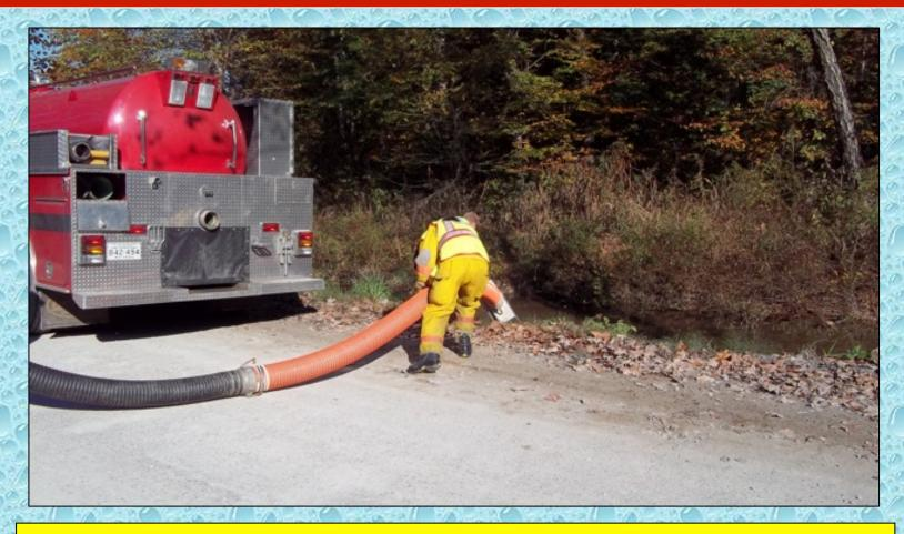
The suction hose is deployed into the stream and will remain in place for the duration of the drill.
