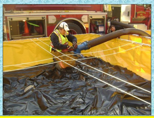
A jet siphon is set-up to transfer water from the second tank into the primary dump tank.
