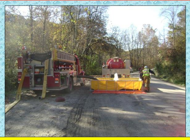
In just 3:55 minutes, the two crews have the dump site set up and the first tanker off loads its 2,000 gallons of water – pretty impressive!
