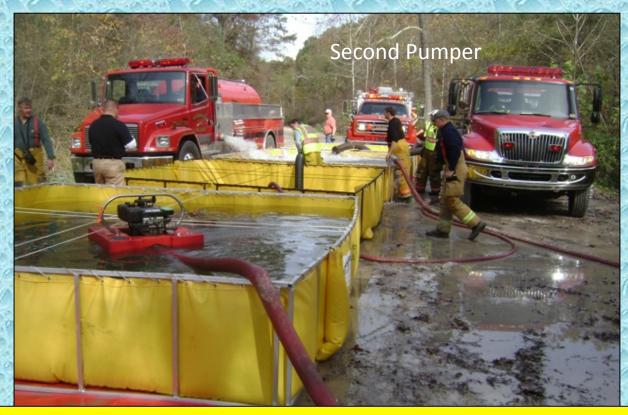
In an effort to improve jet siphon operations, a second pumper was put into operation at the dump site to run jet siphons. The pumper had been hauling water in the shuttle, so the decision to remove it as a water hauler had to be made carefully.
