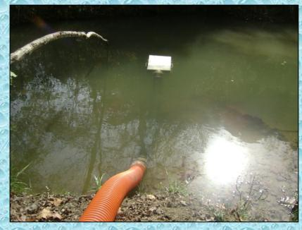
At the second fill site, a similar set-up is used. The first arriving vacuum tanker sets up the suction hose and strainer arrangement and leaves it in place for return trips and for other vacuum tankers to use.
