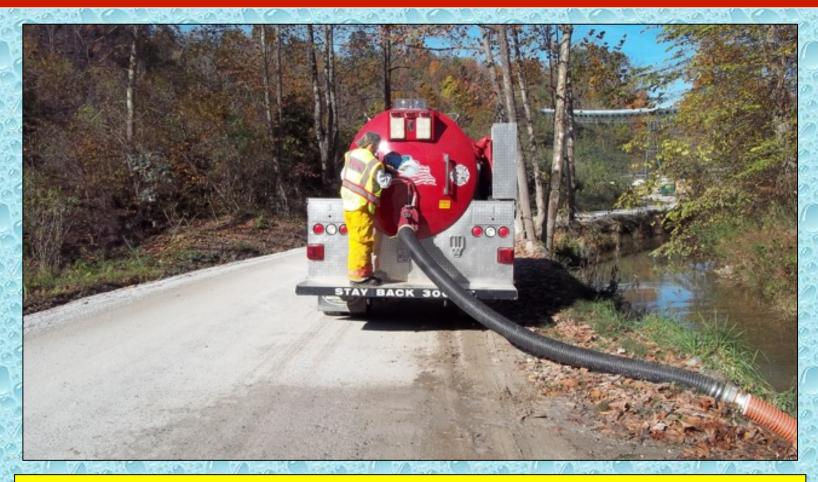
With everything connected, loading commences at over 1,000 gpm without the need for a fill site pumper.
