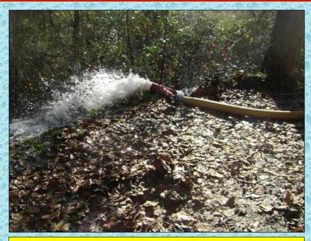
At the 50:00 minute mark, flow is moved to 800 gpm.
