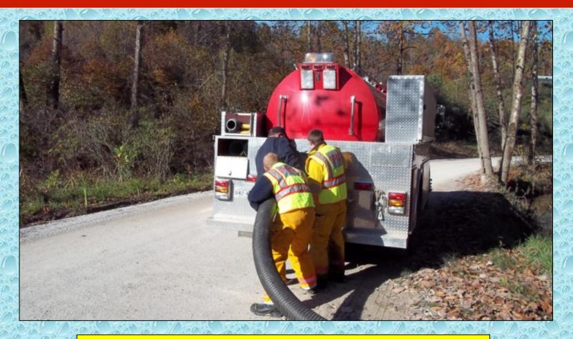
With the strainer in position, the final connection is made.
