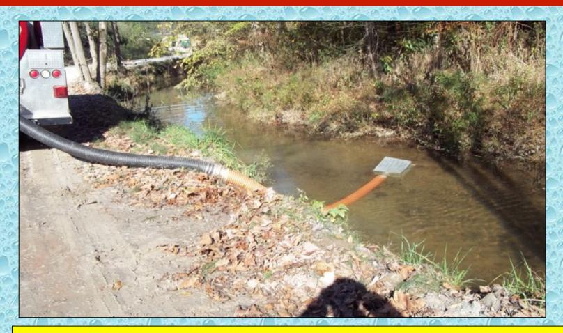
The specially designed strainer has high-flow capability and can operate in shallow as well as deep water.
