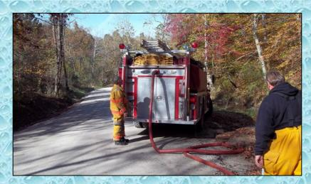
Because there were two conventional style tankers hauling water in the drill, a traditional fill site was needed – thus, a pumper was needed to draft and fill those tankers.
