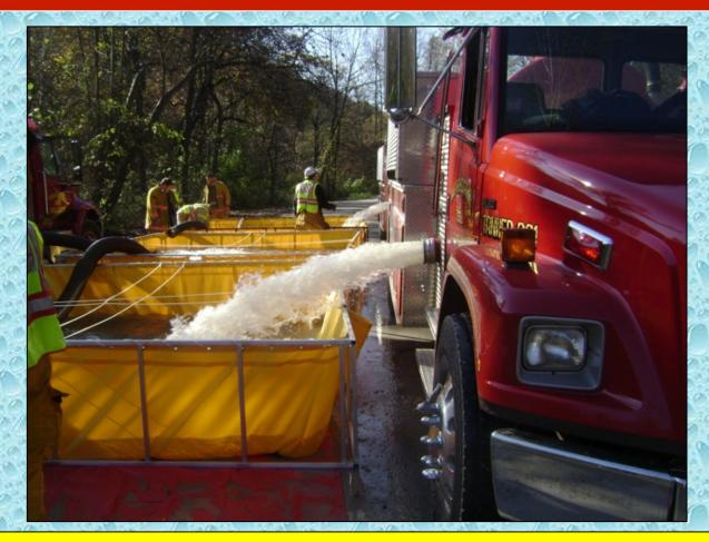
With the third dump tank now in position, two tankers can offload at the same time – a feature that will be needed in order to increase the flow.
