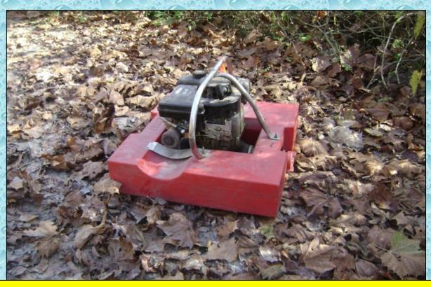
With the fourth tank in operation, a problem arose – the the dump site pumper was nearing its maximum capacity and could not run another jet siphon or support a higher flow. So a 250 gpm portable pump was located to help transfer water.
