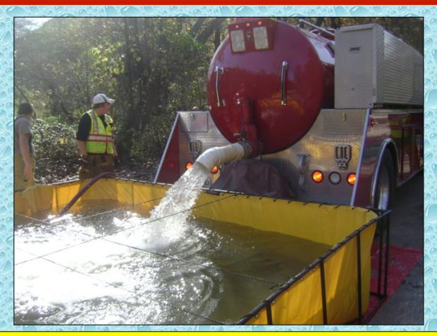
Because of the limited road width, some of the tankers were directed to the end tanks where they could back up and dump and still allow tankers to pass them.
