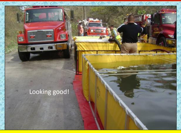
An important note, when setting up dump tanks in the "parallel" arrangement, be sure to keep them aligned as best as possible – otherwise, tanker drivers will have some difficulty positioning their units for offloading water.
