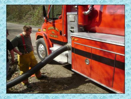
Cam lock style fittings make suction hose fittings easy to connect and disconnect on a vacuum tanker.
