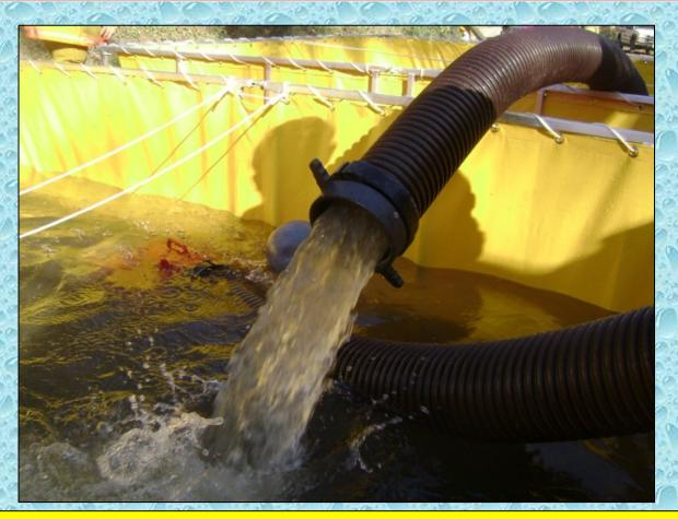
With two dump tanks in operation, water transfer becomes important. This 6-inch jet siphon is moving water very effectively.
