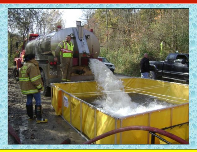
Around the 60:00-minute mark, a fourth, 2,500-gallon dump tank is placed into operation.
