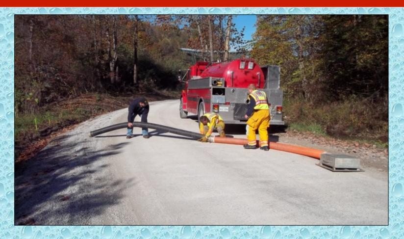
Two lengths of suction hose are needed to reach the stream.
