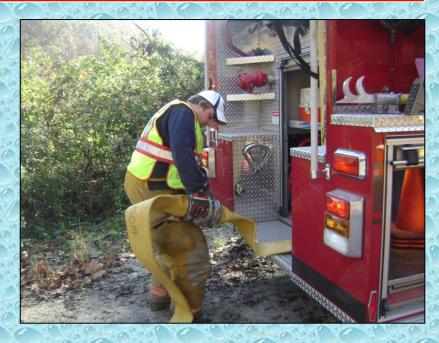
While three personnel work to get a dump tank set-up, the fourth person stretches 100-ft of 5-inch LDH to a flow monitoring device in preparation for starting water flow operations.
