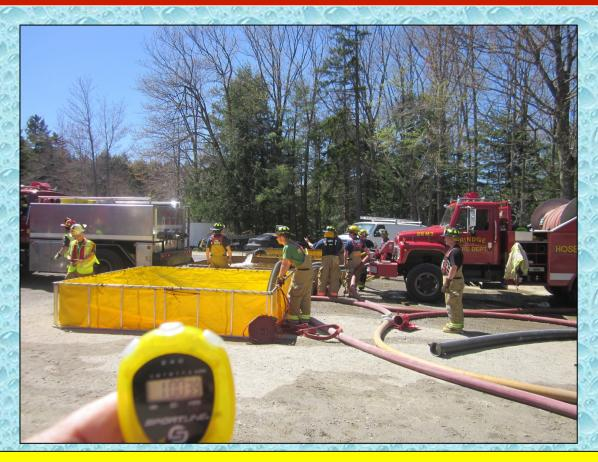
At the 1-hr mark, the 500-gpm flow rate was clearly obtainable using the three-dump tank set up and the 1,000 gpm pumper.
