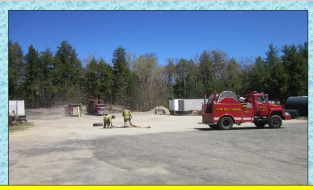
Milford Engine 1 arrived on the scene first and laid a 300-ft, 4-inch supply line. Rindge's Hose Reel Pumper (1,000 gpm) was the next unit to arrive and positioned to operate as the dump site pumper because the other pumpers were on the barn fire. The stopwatch was started when the Milford engine engaged its parking break.
