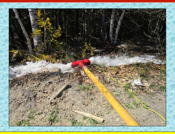
At the 5-minute mark, water flow was started by the Milford pumper. A Hose Monster flow diffuser with built-in pitot was used to measure flow.
