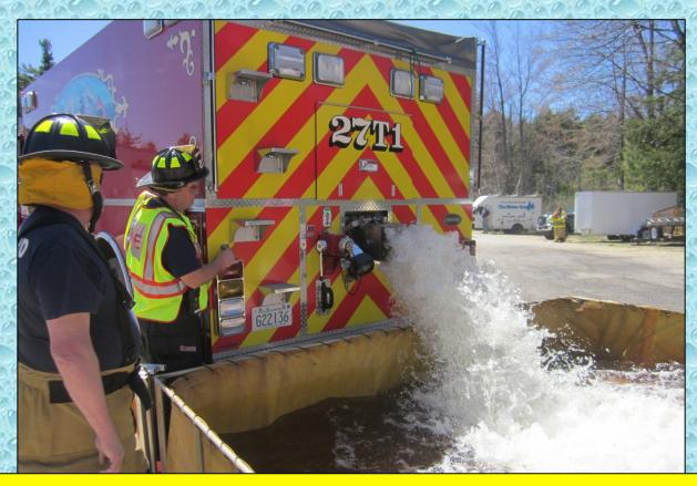
Dump tank operations were now underway and the nurse tanker was returned to water hauling operations. 27-Tanker-1 was the next arriving tanker and dumped its water.
