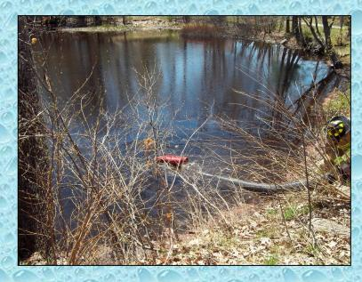
The crew elected to use a traditional drafting operation in lieu of using the dry fire hydrant. They used several lengths of 6" suction hose plus a barrel strainer.
