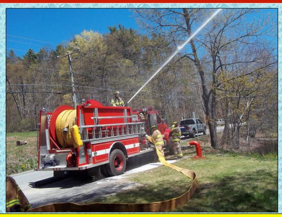
The LDH supply line to the manifold was supplied via the pumper's high-flow discharge. The pumper's deck gun was used as a circulating line in between loading tankers.
