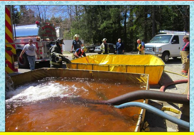
At around the 15-minute mark, a second dump tank was set up and made ready for operation. Meanwhile, the flow was moved to 533 gpm.
