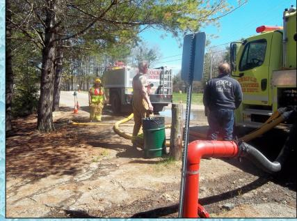
The third fill site was located at Crowcroft Pond which provided a 1.2-mile roundtrip for tankers hauling water. Temple's tanker was relocated from the dump site to this pond with the instruction to set-up to draft and fill tankers. The crew used a 6-inch dry fire hydrant at the pond.
