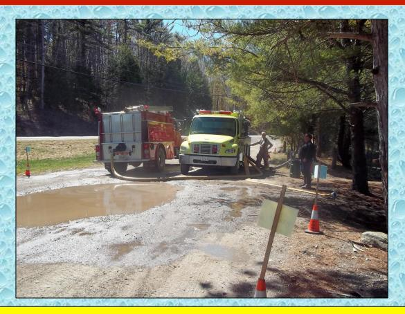
Temple 50-Tanker-1 with its 1,000 gpm pump did a respectable job of drafting and filling tankers. Its two-person crew did a good job of making and breaking connections and getting tankers loaded as quickly as possible.
