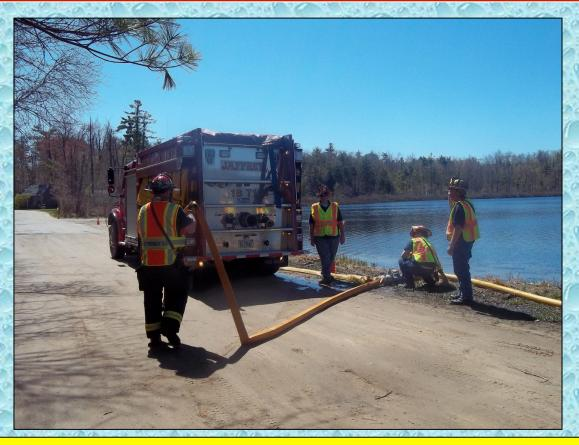
The loading crew used 4-inch hose and an LDH manifold to load tankers. The crew is shown here loading Jaffrey's tanker.
