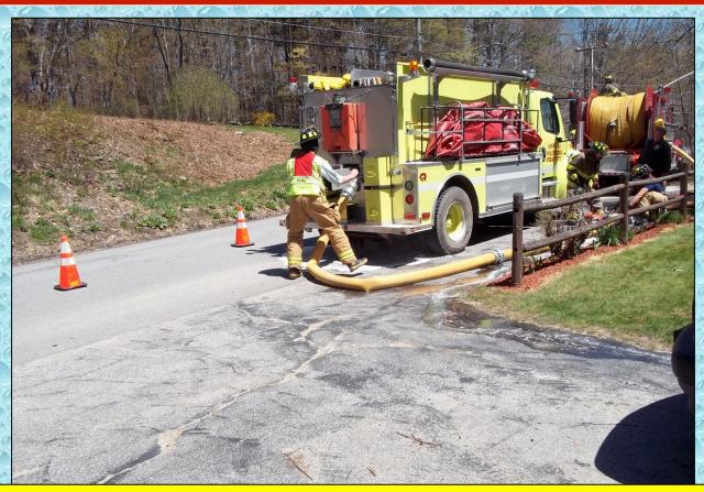
The fill site crew worked hard to fill tankers at a rate of at least 1,000 gpm. Temple's tanker is shown here being filled using its rear direct fill inlet.
