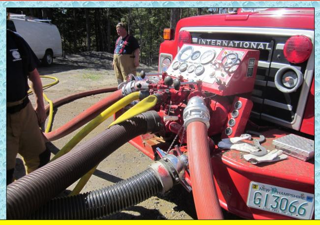
In a final step to maximize flow, dual suctions were used on the front mount pump and the flow was moved to 1,000 gpm plus jet siphons.
