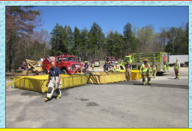
Around the 30:00-minute mark, three dump tanks were in operation – however, the number of tankers was limited and flow was restricted. Note the photo shown here – there are no tankers dumping water or waiting to dump water.
