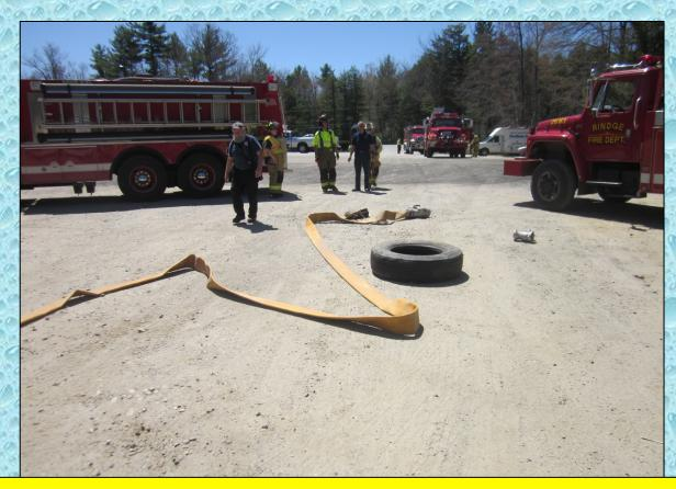
The rural hitch operation is an easy way to allow a tanker to pump off its water and support the fire attack during the early phase of a rural water supply operation.
