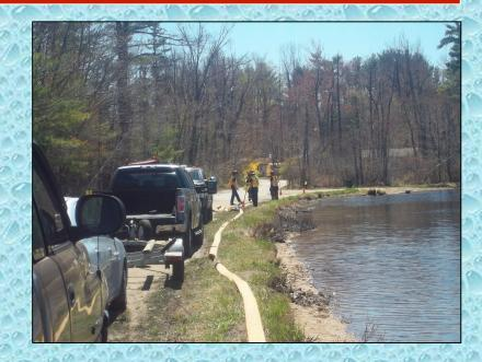
The second fill site was located at Grassy Pond and provided a 2.8-mile round trip for tankers hauling water. Jaffrey FD's hose reel pumper was used as the source pumper for this operation. Its front mount pump made for easy access to the water.
