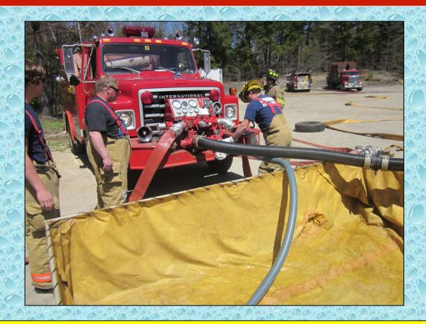
The dump site pumper positioned so that the front-mounted pump could be used as efficiently as possible.
