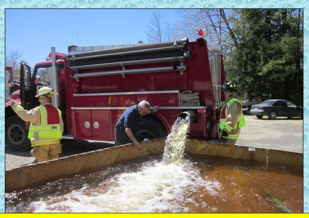
With the first dump tank all set up and ready, the first load of water was offloaded. Meanwhile, nurse tanker operations continued until the dump site pumper obtained a draft.
