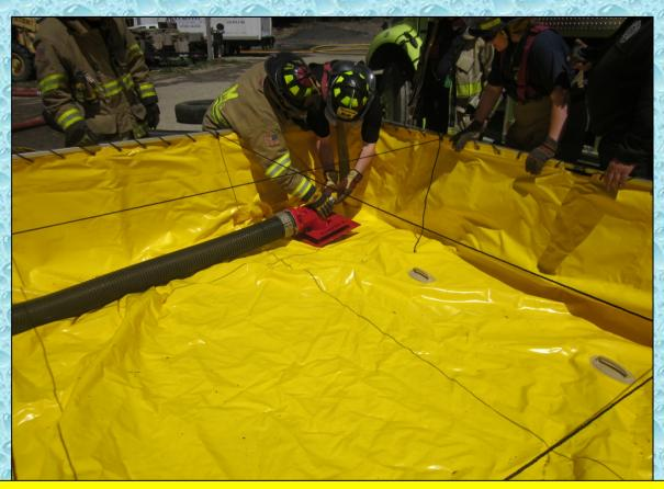
Water transfer operations are critical in all dump site operations. The crews are shown here setting up a low level suction strainer as a water transfer device.
