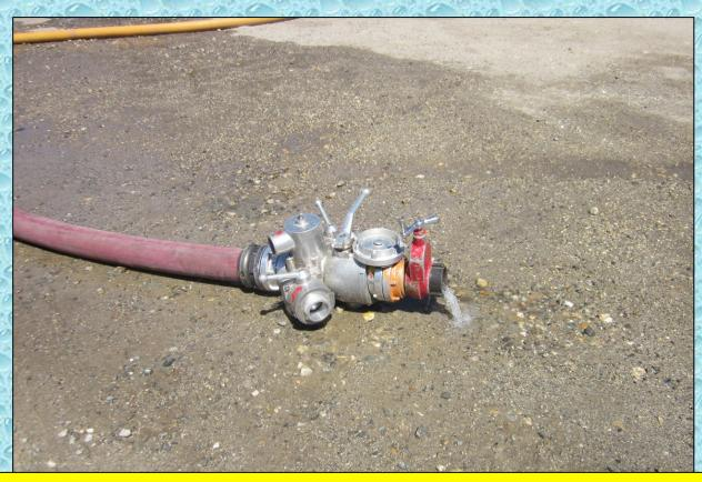
There were a couple of leaky LDH appliances found at this drill. Most of the leaks dealt with sand and grit preventing the complete closure of a valve. It is important to thoroughly clean and rinse these devices after each use.
