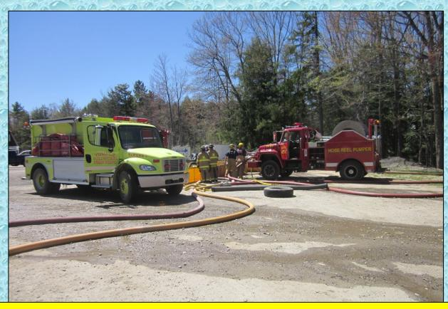
One of the challenges of the drill was the 1,000 gpm pump capacity on the Rindge hose reel pumper. At one point, plans included the use of Temple Tanker 1 as a pumper so that jet siphons could be supplied without using the Rindge unit.
