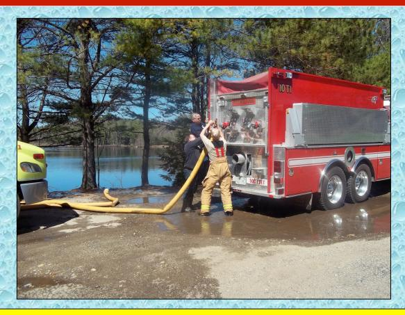
This photo is a good example of why it is important to design tankers with low, direct fill lines. Valuable time was lost making and breaking this connection.
