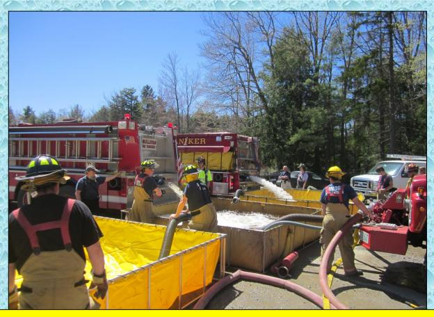
As tankers cleared the barn fire, they joined the shuttle operation. The additional tankers brought stabilization to the water flow.
