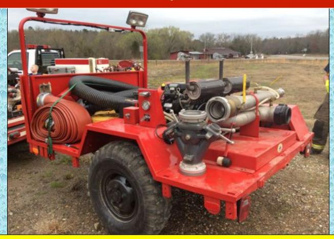
Ringold's trailer pump, outfitted with two, 550-gpm pumps connected in parallel was used to load tankers at Tucker Lake. Ringold's Truck 1 (1500 gpm pumper) was used as well – drafting through a dry fire hydrant.
