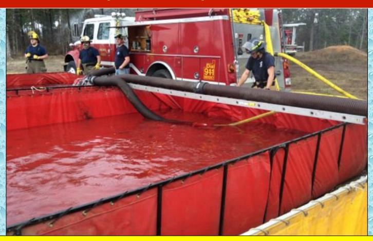
Water transfer operations quickly became important as a third dump tank was deployed. Several jet siphons were used to move water between tanks.
