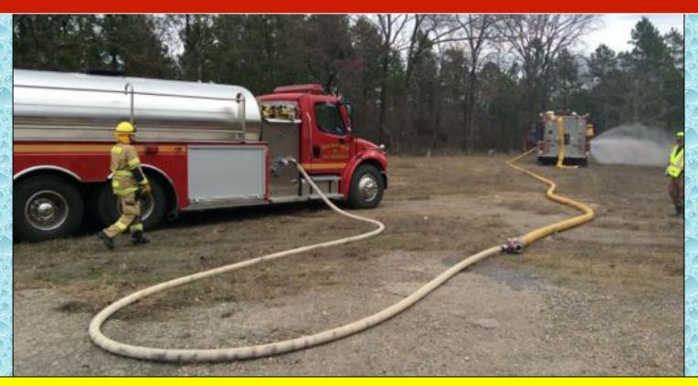
Hochatown Tanker 30 (3,000 gal) was the next unit to arrive on the scene. The crew used a pre-connected length of 2-1/2" hose line to quickly connect to the siamese and supply the attack engine. A 250 gpm flow was started at the 5-minute mark.
