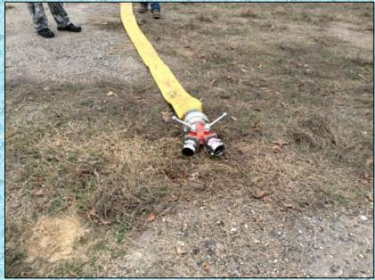
Hochatown Engine 65 was the first-arriving engine and laid a 200-ft, 5-inch supply line and set up as an attack engine. A clappered siamese was not available, so a 2-1/2"x2-1/2"x5" gated wye was used (reversed) so that nurse tanker operations could be used to support the initial attack.
