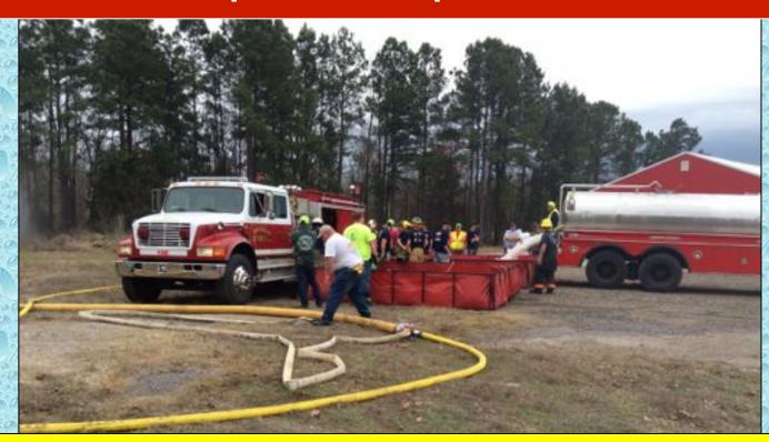
Transition to dump site operations occurred around the 12-minute mark (yellow hose) and the nurse tanker dumped the remainder of its water into the dump tanks and left to reload. Flow had been moved to 350 gpm at the 8-minute mark.
