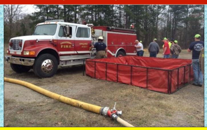
Eagletown Engine 4022 (1250 gpm) was the next arriving engine and went to work setting up as the dump site engine. The first dump tank (3500 gal) was taken from the nurse tanker.
