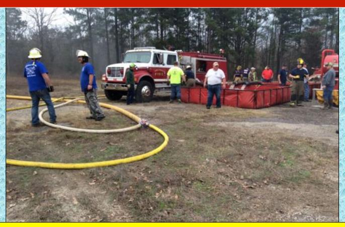
The dump site engine charged the second supply line feeding the gated wye and the dump site was now ready to increase flow to the attack engine.
