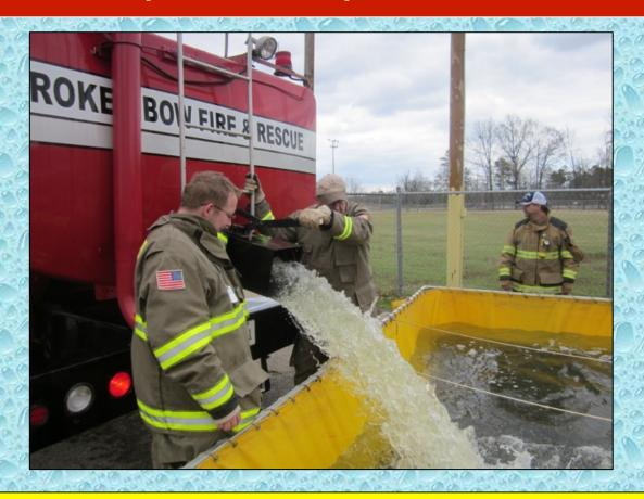
With the third dump tank now in operation, there was plenty of water in storage on site at any given time and water flow was never interrupted.
