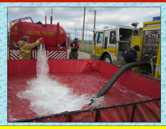
At the 2:52-minute mark, Truck 7 dumps its 2,500 gallons of water and the dump site pumper obtains a draft.
