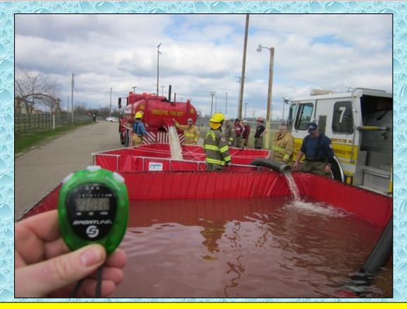
At 23-minutes, the first tanker has returned from the fill site – which is pretty good timing. However, it is important to note that the fill site was only within a 2-mile round trip.
