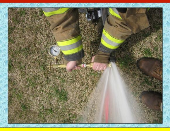
Flow measurement for the drill used a hand-held pitot tube along with smooth bore nozzle tips.
