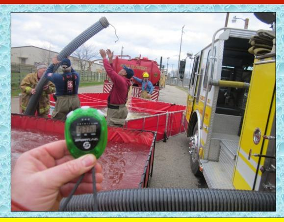
Ringold Truck 5 dumps its 2,500-gallon of water as effort is underway to place the second dump tank into operation.
