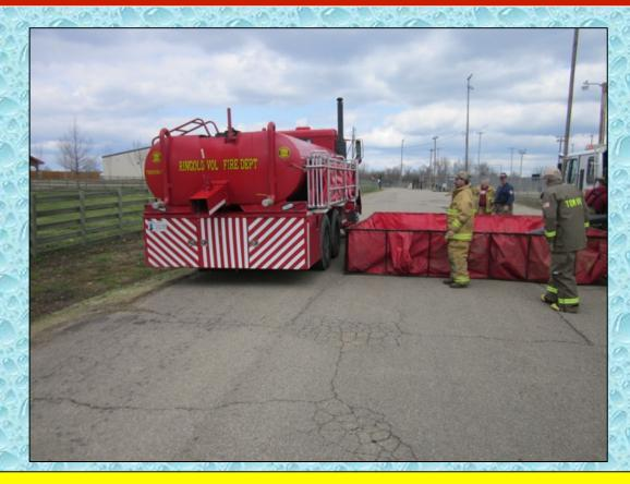
As noted already, dump tank placement is critical. This 3,500-gallon dump tank had to be carefully positioned so that tankers could drive past the site.
