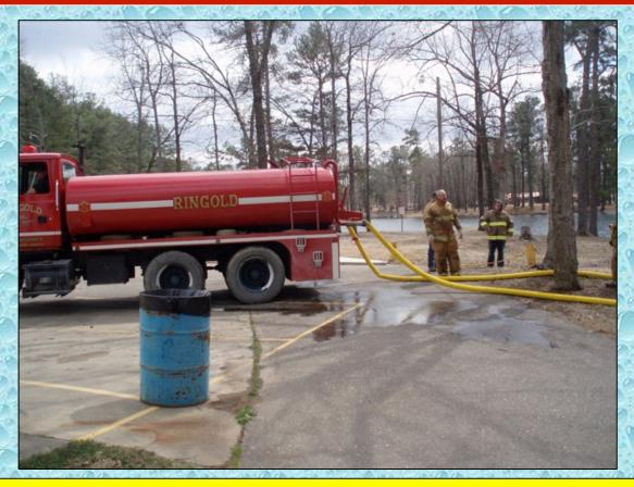
Two, 3-inch fill lines were used to load some of the tankers at this fill site. Later in the drill, a change-over to LDH helped to speed up the operation.
