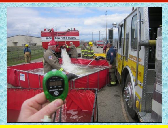
The third dump tank was not placed into operation until the correct water transfer equipment was available.
