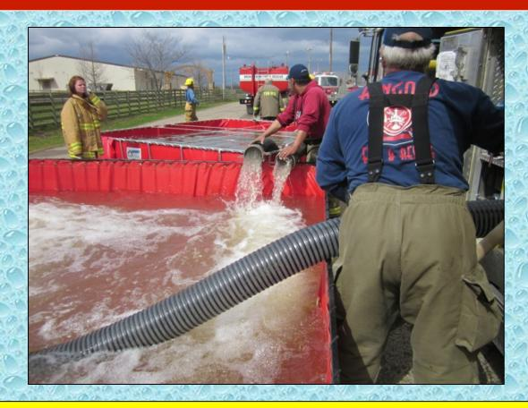
With two jet siphons now in use, the flow was moved to 800 gpm at around the 83:00-minute mark.
