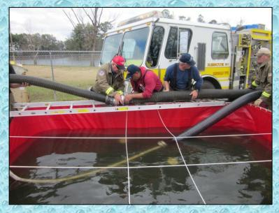
The plan was to transfer water from the 3<sup>rd</sup> dump tank directly into the 1<sup>st</sup> dump tank by "jumping" the second tank. To make this work, extra suction hose was needed. The problem that arose was that one section of hose was 5" and the other 6" in diameter. Thus – folks had to be a bit creative on adaptor use.
