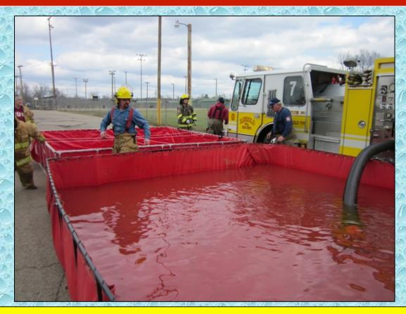
Knowing that the goal is to increase flow, a second dump tank is deployed as soon as possible. Truck 7's 3,000-gallon dump tank is shown being set up after the tanker dumped its water into the first dump tank.
