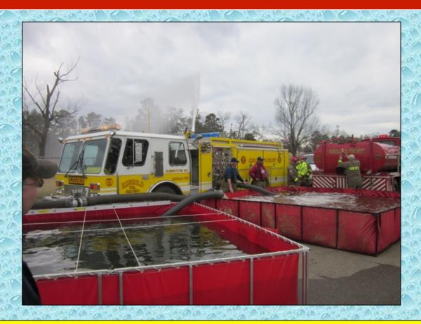
Jumping the 2<sup>nd</sup> dump tank really made a big difference in managing the water transfer operations at this drill.
