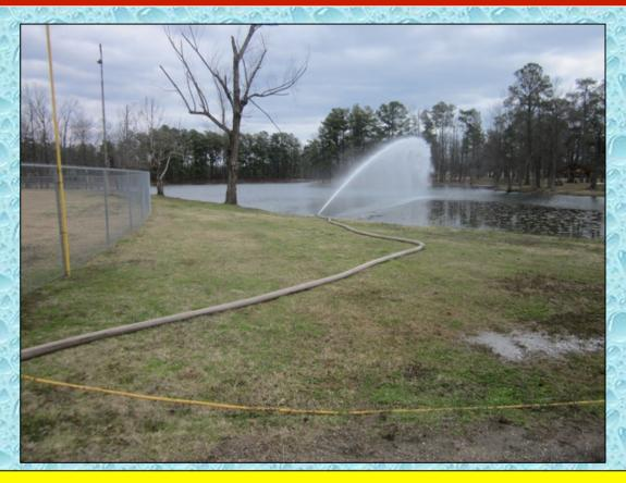
At 19:00 minutes, the water flow was increased to 500 gpm where it was maintained for over one-hour before being increased.
