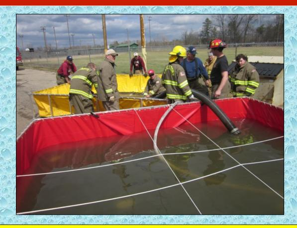
Around the 27:00-minute mark, a third dump tank is placed in preparation for expanding the flow.
