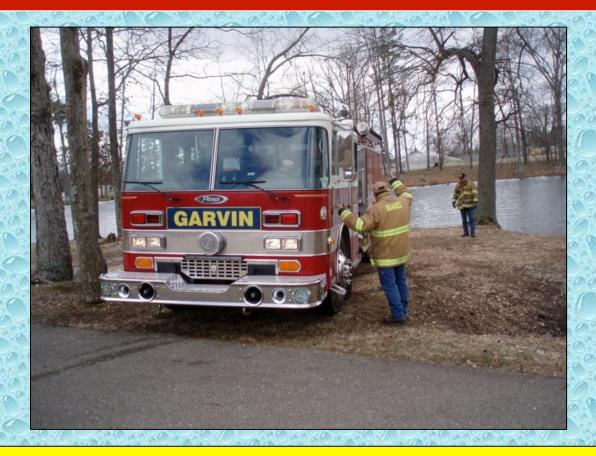
With limited suction hose onboard the pumper needed to be positioned close to the shoreline.
