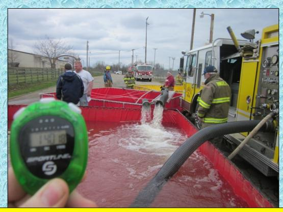
A critical point was reached about 20-minutes from the end of the drill. The flow was 800 gpm and there were no tankers dumping water or waiting to dump water. However, about two minutes later, a tanker arrived and flow continued interrupted.
