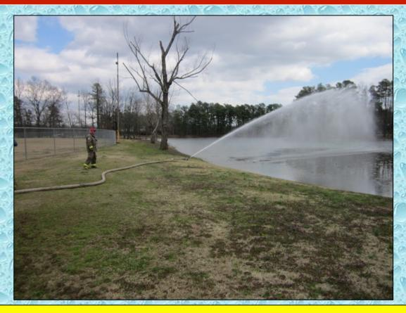
Water flow is started at 250 gpm at the 4:27-minute mark and now the goal is not to interrupt the flow.
