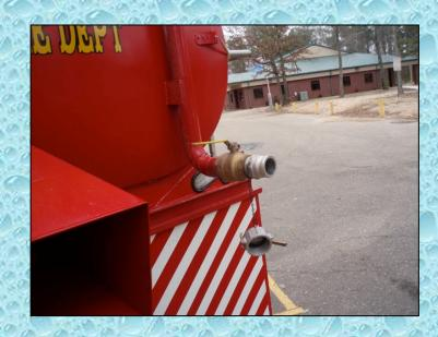
One issue that can arise at a loading site is the need for adaptors because of the different types of tanker fill connections. A good tanker fill site has an entire allotment of adaptors ready for use by the loading staff.
