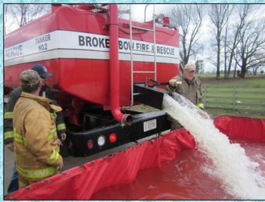
Around the 9-minute mark, Broken Bow Tanker 2 arrives and begins to offload its 5,000 gallons of water. Meanwhile, the dump site crew begins to assemble the items needed to transfer water between dump tanks.
