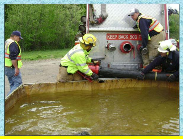
With the arrival of other apparatus, a 6-inch low level strainer replaces the 2-1/2-inch strainer and the drafting operation is ready to begin.
