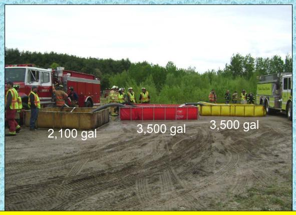
The crews used a three-dump tank set-up to supply the water needed by the attack engine. The tanks were set in a diamond shape and jet siphons were used to transfer water.
