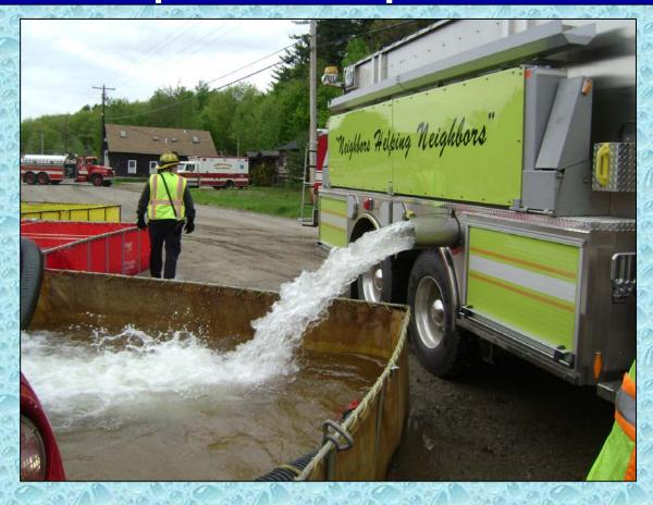
The advantage of side dumps is illustrated above. Strafford 25E3 offloads its 3,000 gallons through one of its 8-inch side dumps.
