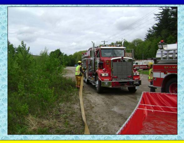
Holderness 12E5 (2,500 gallons) is the first tanker to return from the fill site and is shown above getting ready to pump to the clappered siamese (rural hitch).
