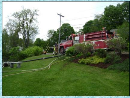
While the lift was not that high, the access was a bit far, so additional lengths of suction hose were needed to reach the water. In addition, the crew used a 500 gpm portable pump to help boost the output of the operation.
