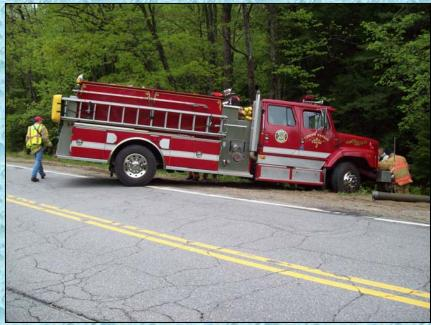
The stream that was used at this fill site had about a 15-ft lift and difficult access. The crews had to be careful in positioning the pumper and used 30-ft of hard suction to reach the water.
