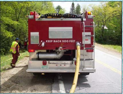
Without an LDH manifold handy, a traditional gated-wye was adapted to fit the LDH which was then used as the control valve for filling tankers.
