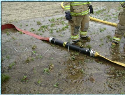
An electronic flow meter was used to monitor the flow on the 4-inch line that fed the portable monitor.
