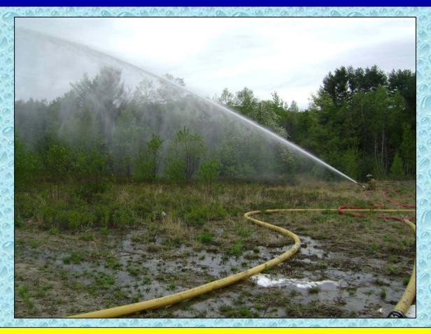
At the 65-minute mark, the flow is moved to 750 gpm while still using the portable monitor fed by a 4-inch supply line.
