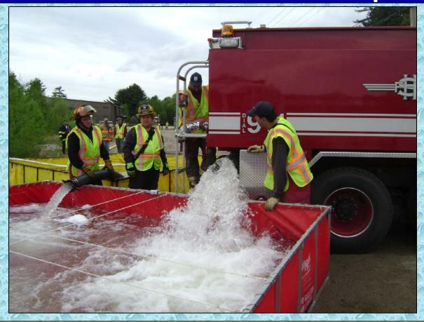
Stratford Hollow 40W1 can really offload its 3,000 gallons when it uses its 12-inch rear dump that can pivot to either side of the rig.
