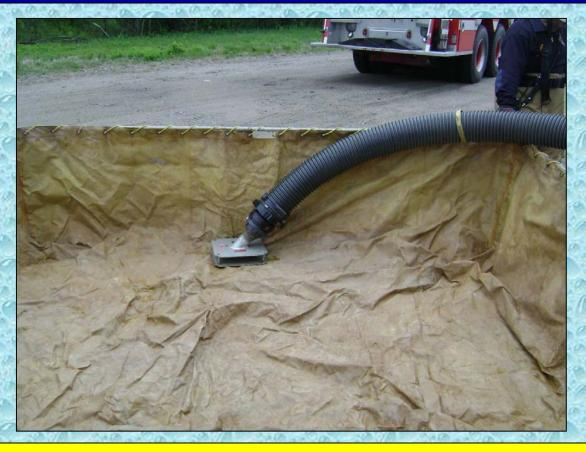
As units from the Water Supply Task Force began to arrive, the dump site was set-up. Here, the only strainer available was a small, 2-1/2-inch forestry-style strainer. Fortunately – it was changed out when a bigger strainer arrived.
