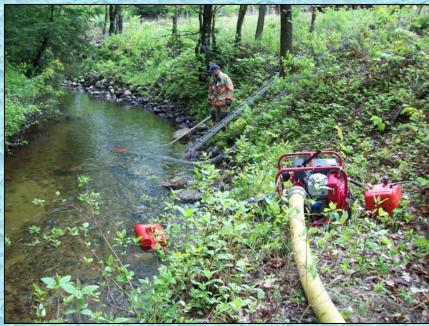
To help improve the operation, a 500 gpm portable pump was put into operation. The crews did a good job of reducing the lift by putting the portable pump as close to the water's edge as possible.
