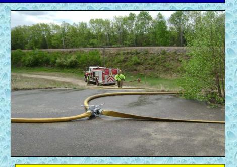
Gilford's 8E1, a 2,000 gpm pumper connected to the hydrant and provided the pumper support for the LDH manifold. Note the additional valves on the hydrant – excellent work for expanding water supply operations if needed.
