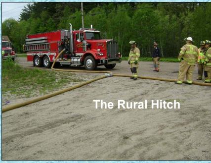
Campton Thornton 35E1 and Holderness 12E5 arrive and begin pumping off their water to support the fire attack operations. A clappered LDH siamese is used so that both engine/tankers can be connected at the same time to the attack engine's supply line.
