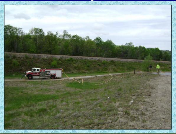
This fill site was a hydrant located just off of Route 3 near Interstate 93. The hydrant was on a large main and provided plenty of flow and operating pressure for tanker fill site operations.
