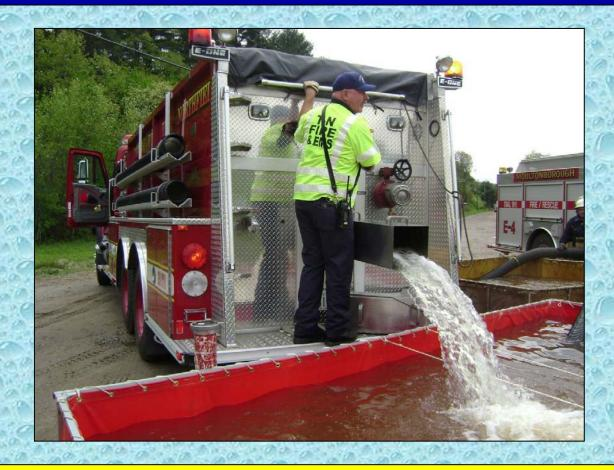
With the dump site now operational at 500 gpm, the ability to quickly off-load tankers becomes an important function.
