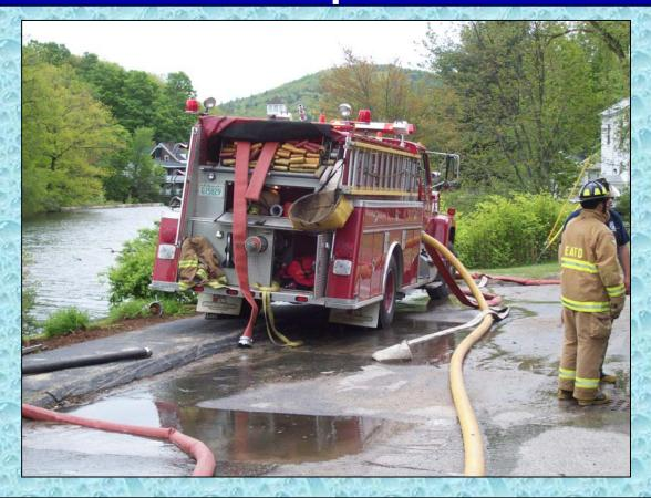
The crew of East Andover 32E3 gave their older rig a great workout at this fill site. The 1,250 gpm pumper and its crew drafted from a manmade lake in downtown Ashland and filled tankers using 4-inch hose.
