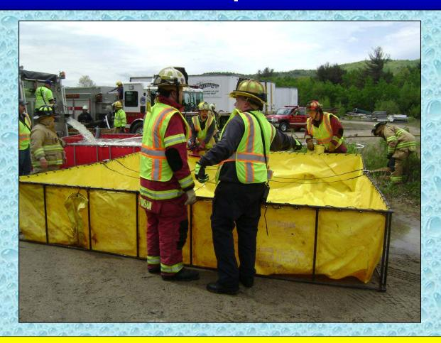
With the arrival of units from the 3<sup>rd</sup> Water Supply Task Force, another 3,500-gallon dump tank is deployed.
