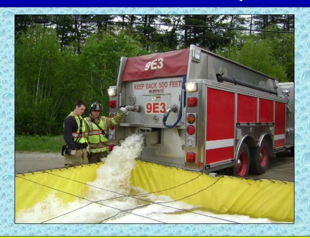
Gilmanton 9E3 offloads its 2,500 gallons using a rear 10-inch dump. These large dumps can off-load water at a rate in excess of 1,500 gpm.
