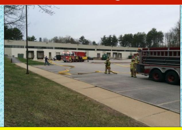
Alton 1 Engine 2 was the first-arriving engine followed shortly thereafter by Meredith 14 Engine 4 which set up for nurse tanker operation using 4-inch LDH and a double-clappered siamese ("the rural hitch.")
