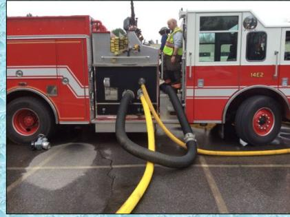
Triple suctions were used on the Meredith dump site pumper so that the rig could support a 1,400 gpm flow and run three jet siphons at the same. The triple suctions allowed this 1,250 gpm pumper to exceed its rated capacity.
