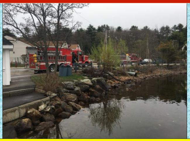
Holderness 12 Engine 5 (1,500 gpm) drafts out of Waukewan Lake and loads tankers at a rate of 1,000 gpm.
