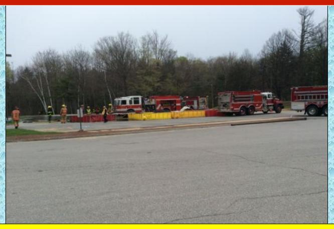
The final set-up of the dump site. The four-dump tank arrangement produced a peak flow of 1,400 gpm.
