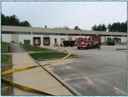
Within a couple of minutes, Meredith 14 Engine 2 arrived on the scene and began setting up to transition to a dump tank operation because flow was expected to exceed 1,000 gpm. Water flow was started at 250 gpm at the 5mimute mark.
