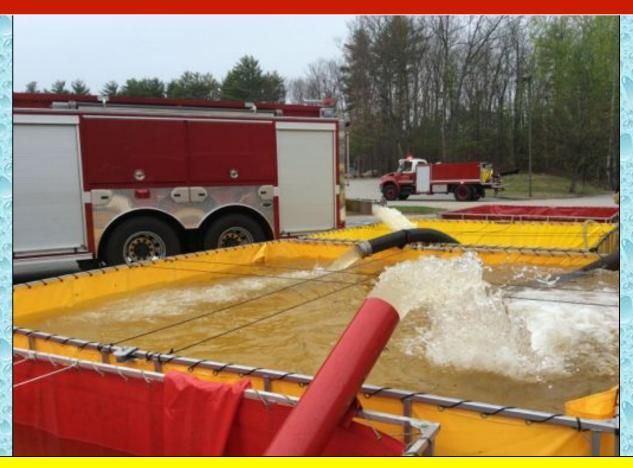
With four dump tanks in operation, water transfer operations became very important. A Kochek Holley Tube and a traditional jet siphon are seen in use in this photo.
