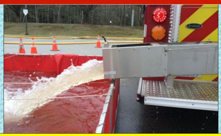
Knowing the importance of when to "cut and run" for another load of water...a piece of white medical tape on this 10-inch dump chute lets the folks know when to close the valve and head for another load of water.
