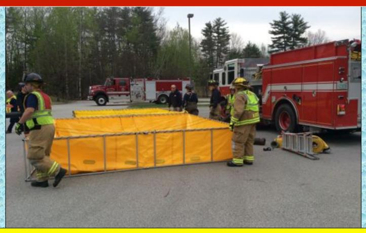
Crews work to set up the dump site while nurse tanker operations are under way.
