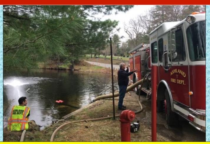
Ashland 2 Engine 2 (1,500 gpm) drafts directly from Wickwas Lake and loads tankers at a 1,000 gpm rate.
