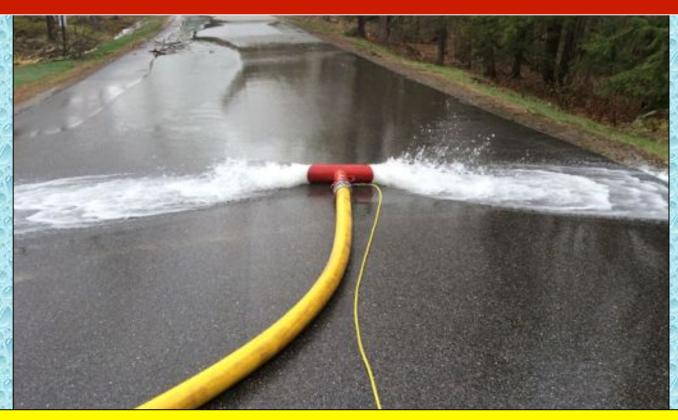
A Hose Monster flow diffuser with fixed-pitot was used to control and measure the discharge flow during the drill.
