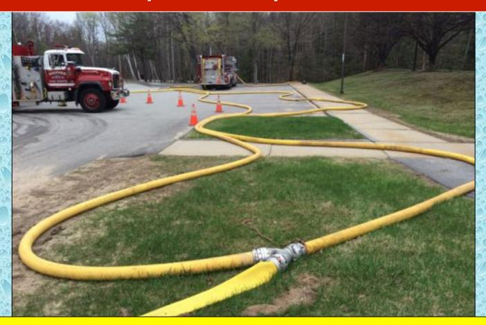
The rural hitch in operation ...but now changed over to dump site operations with flow at 750 gpm at the 15-minute mark. The charged 4-inch LDH on the left side of the photo is being supplied by Meredith 14 Engine 2 at the dump site.
