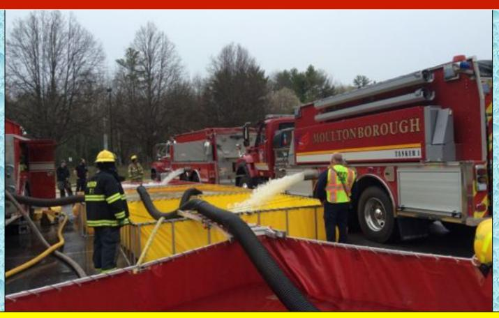
At the 19-minute mark, three dump tanks were down and in operation and flow was being sustained at 750 gpm. Preparations were underway to bring a fourth dump tank on line.
