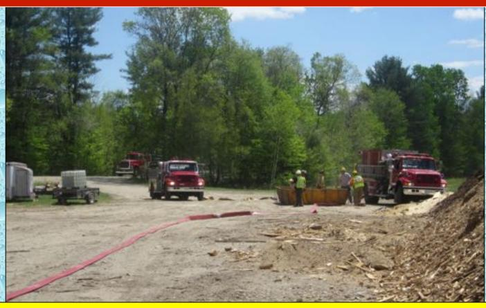
Taken at around the 3-minute mark, the photo shows Wentworth 42 Engine 3 (right) setting up as the dump site engine. The engine is ready to pump into a 4" double-clappered siamese (rural hitch) while the dump tanks are being set up.
