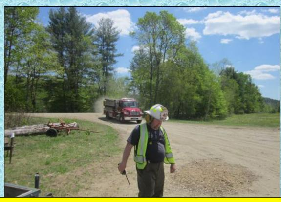
Wentworth 42 Engine 3 was the first-arriving unit and assumed the role as the attack pumper. The plan was to use a "rural hitch" operation initially and then transition to a dump tank operation. The stopwatch was started when the pumper driver applied the air brakes.
