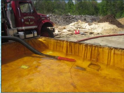
One of the issues that arose early in the drill was the lack of a low level strainer for use in the dump tank. The dump site engine had to use a floating barrel strainer from about 15 minutes until a low level strainer arrived on a tanker. The floating barrel kept wanting to turn over, so the float was taken off.
