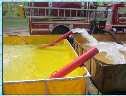
Two, 6-inch Kochek Holley Pipes were used as the initial transfer devices for the second dump tank that was placed in operation. The pipes worked really well.
