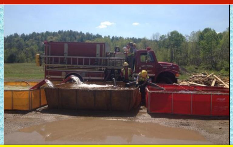
The final set-up. All three tanks are full of water and the flow has moved to 500 gpm for the final 30-minutes of the drill.
