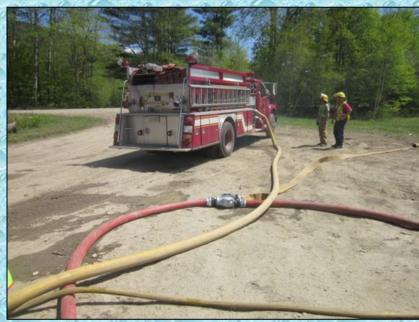
With the operation shifted to a dump tank operation, use of the rural hitch ceased – however, it was kept in place in case it was needed (double-clappered siamese in photo on the right). In the mean time, a pump-off pipe (photo on the left) was used to allow engines to pump off their water directly into a dump tank. This allowed each engine to get back on the road sooner to get another load of water.
