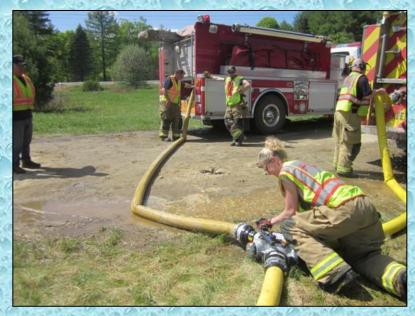
Warren Engine 2 (1,250 gpm) was used to draft from the pond using a dry fire hydrant and supply a TFT LDH manifold which controlled the 4-inch lines used to load tankers.
