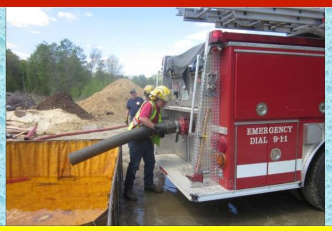
Many of the water hauling rigs could only dump from the rear, so dump tanks were arranged to accommodate that off-loading method.
