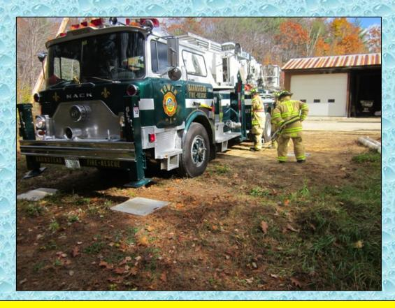
Barnstead's 6-Tower-1 (a gorgeous Mack Aerialscope) arrived next and got into position to operate a 1,000 gpm aerial stream once the dump site operation was ready to support such a flow.
