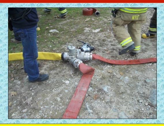
An older style Jaffrey manifold valve was used as the tanker loading valve. The valve was supplied via 4-inch LDH and in turn, tankers were loaded using 4-inch LDH.
