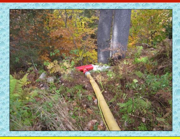
Water flow was started at the 5:00 minute mark at a rate of 250 gpm. A Hose Monster flow diffuser was used to accurately measure the flow during this part of the drill.
