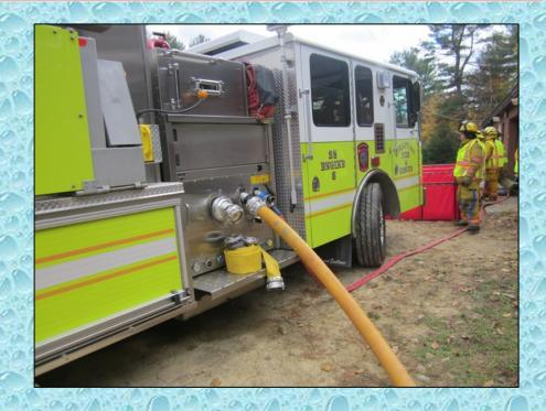
Around the 13:00-minute mark, 25-Engine-3 started drafting from the dump tanks and the operation was switched from a nurse tanker operation to a dump tank operation.
