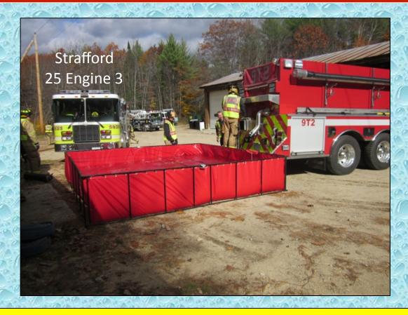
Strafford 25-Engine-3 arrived and assumed the role of the dump site pumper. The 1,750 gpm pumper was going to be needed if a 1,000 gpm flow was to be attained.
