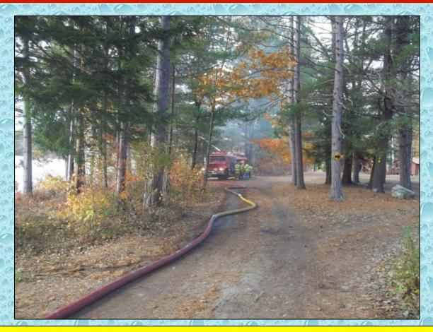
The pumper laid out several hundred feet of 4-inch LDH to supply the loading manifold.
