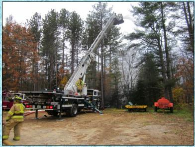
At the 60:00-minute mark, water flow was moved to 750 gpm and flow was switched from the Hose Monster to 6-Tower-1's elevated master stream which was equipped with a fixed pitot tube and gauge for accurate flow measurement. Water flow was moved to 800 gpm at the 75:00-minute mark.
