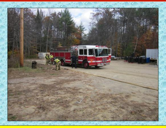
Gilmanton 9-Engine-3 arrived next and got into position to supply its 2,500 gallons of water to the attack pumper via the clappered siamese.
