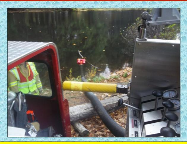
About 30-feet of suction hose was needed to reach an adequate water depth.
