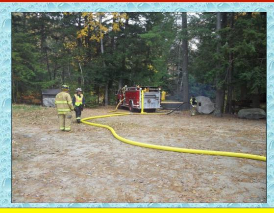
Several hundred feet of 4-inch hose was used between the Chichester pumper and the loading site – which once again shows the value of using LDH in the rural setting.
