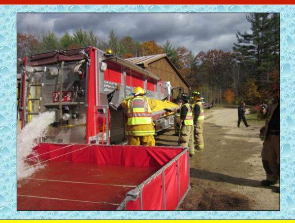
With the first dump tank in operation, the crews now go to work getting ready to set up a second tank knowing that they want to get to that 1,000 gpm flow.
