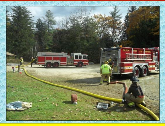
A fill station needs to operate much like a "NASCAR pit stop." The "loader" operates the manifold and fills one tanker at a time – meanwhile, the next tanker gets connected in preparation for filling.
