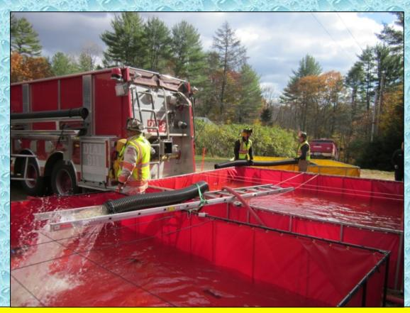
With water transfer operations now underway, water flow was moved to 630 gpm at the 16:30-minute mark.
