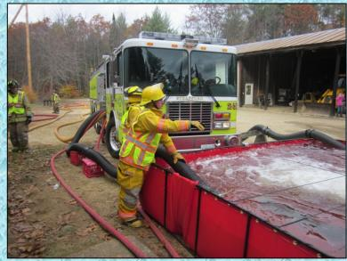
At the 83:00-minute mark, 25-Engine-3 deployed a second suction hose so that flow could be increased. The pumper is equipped with suction inlet control valves, so adding the second suction occurred without having to shut down water flow. Once the second suction was operational – flow was moved to 980 gpm. At the 85:00-minute mark, the flow was moved to 1,000 gpm where it remained through the remainder of the drill.
