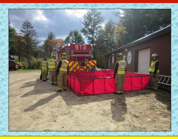
Gilmanton 9-Tanker-2 gets ready to dump its water into the dump tank. The problem is that no dump site pumper has arrived yet – so dumping the water into the tank would result in trapped water that no one could use.
