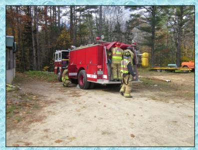
Gilmanton 9-Engine-2 was the first-arriving unit and assumed the role as the attack pumper. The 4-person crew divided up tasks and deployed an attack line and a 4-inch supply line. The stopwatch was started when the pumper driver applied the air brakes.
