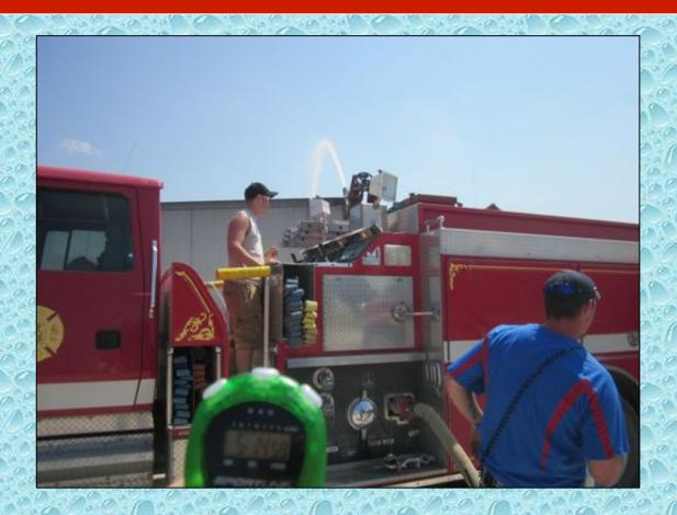
At the 5:00 minute mark, water flow is started at the attack pumper using the prepiped deck gun. A hand-held pitot gauge was used to verify flow.
