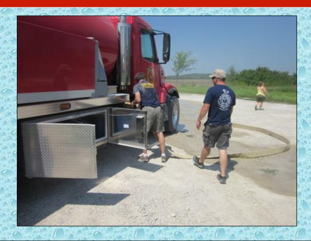
Tender 3661 prepares for nurse tanker operations using its 750 gpm pump to supply the attack pumper (E3651) until the dump site can be made operational.
