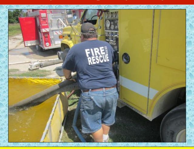
A length of 2-1/2-inch suction hose was added by the dump site pumper in order to increase pumping capacity to 1,250 gpm.
