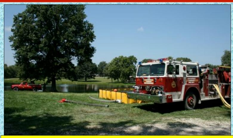
Centropolis Engine 3851 (1,000 gpm) then drafted out of the dump and filled tankers using dual, 3-inch hose lines.
