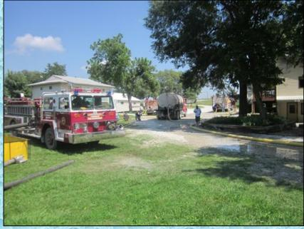
Eventually, 6-inch suction hose was located on one of the rigs and the pumper increased its ability to load tankers. The "open relay" was used to meet the 1,000 gpm fill rate while using a limited supply source (400 gpm grass rig).
