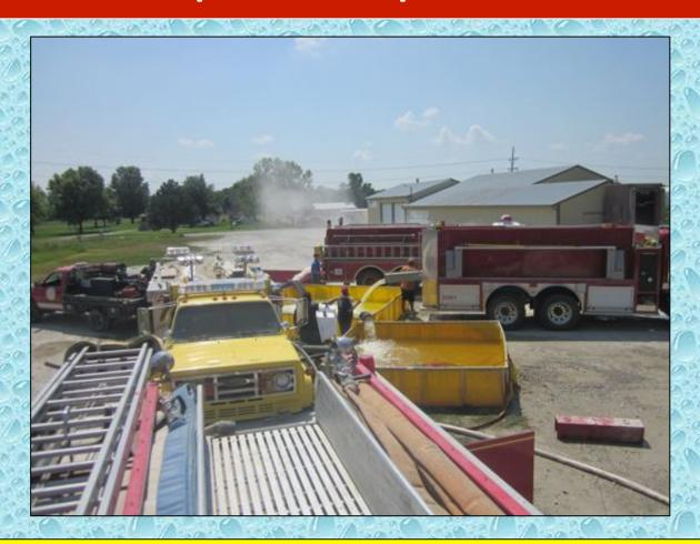
Because almost every tanker dumped off of the rear only, the three dump tanks were placed in a "diamond" configuration – thus creating a loading dock effect.
