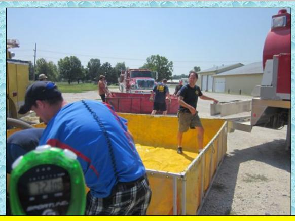
Pottawatomie Tender 3361 (3,000 gallons) arrives next around the 7:20-minute mark. With nurse tanker ops still underway, crews work to get a second dump tank down in preparation for a larger operation.
