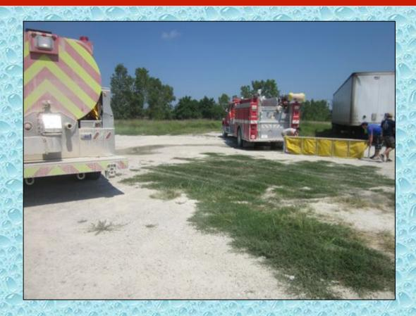
Engine 3651 carries a 2,100-gallon dump tank and crews go to work setting up that tank in preparation for moving to a dump site operation.
