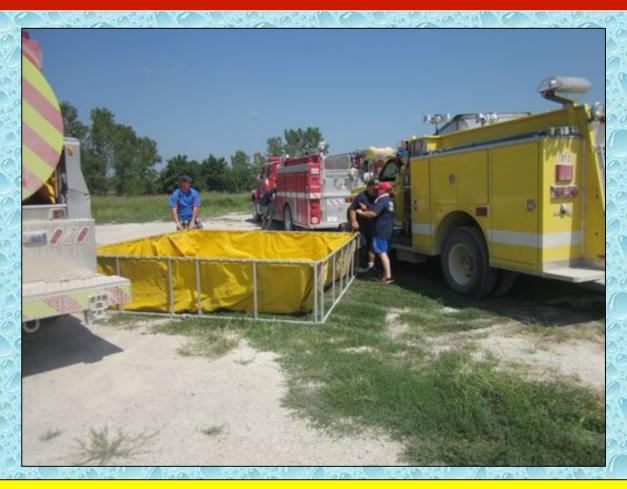
A total of five persons operated two pumpers and a tender while at the same time set up the first dump tank – all within five minutes of arrival.
