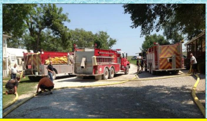
All loading operations took place in the main parking lot at the church camp. Two independent fill site pumpers supported two loading stations in the same parking lot. Note the 5-inch LDH supply line on the right that supported one of the loading stations.
