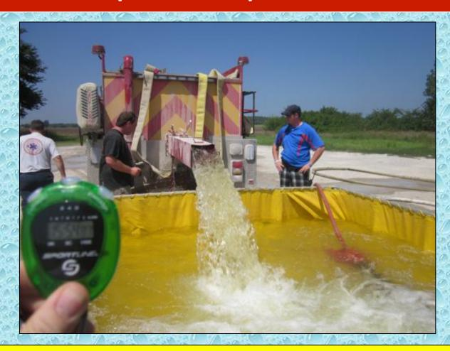
Wellsville Tender 3761 quickly dumps its 1,800 gallons of water as flow is moved to 500 gpm.
