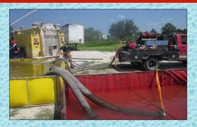
The Cutler grass rig (400 gpm) drafted from Tank 2 and powered a jet siphon (orange supply feed) to transfer water from Tank 3 into Tank 2. Note: the second suction line in the red tank was not in use at the time of the photo. Crews were waiting on a jet siphon device.
