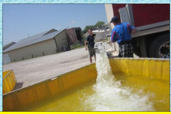
Tender 3661 dumps some of its 4,000 gallons into the first dump tank while still pumping to the attack pumper. This water was used to allow the dump pumper to obtain a draft.
