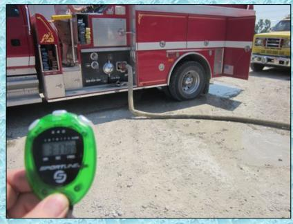
The key to the success of this drill was the ability of the first tender (T3661)to pump its water to the attack pumper (E3651) until such time that a dump site could be set up. At just over the 3-minute mark, Tender 3661 is connected and supplying water to E3651 through a single, 3-inch line.
