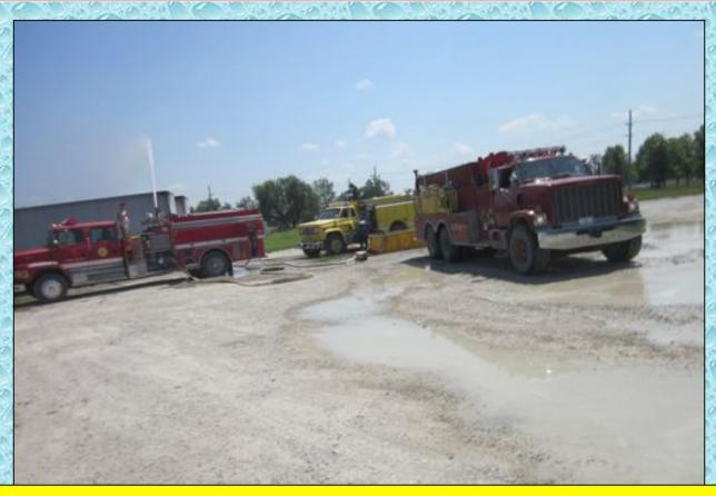
A two-dump tank operation was now underway and all nurse tanker operations had stopped. The attack pumper (red) is being supplied by the dump site pumper (yellow) via dual, 3-inch supply lines.
