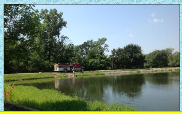
Engine 3652 (1,500 gpm) drafted from the dam and supplied water back to a loading station via 400 ft of 5-inch LDH. This loading station easily met the 1,000 gpm fill rate goal.
