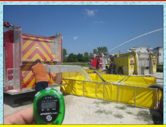
Water transfer devices are in place and the second dump tank is placed into operation at 14:41 minutes.
