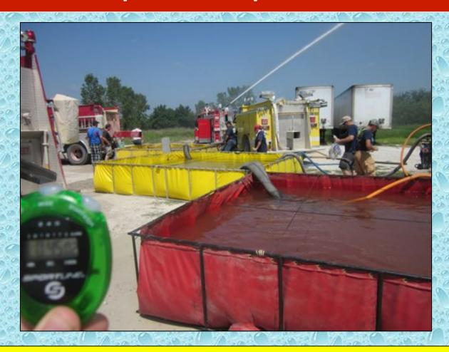
At the 45-minute mark, three dump tanks were full of water and tankers were waiting to dump.
