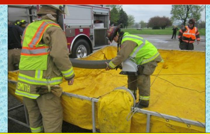
A TFT low level strainer was used for drafting. This all had to be set up in preparation for flowing water at the 5:00 minute mark.
