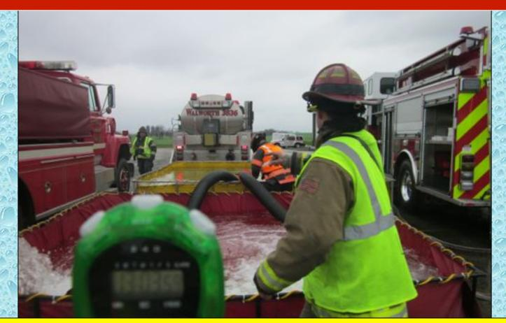
By the 13-minute mark, two dump tanks were in operation and preparation was underway to move the flow to 500 gpm.
