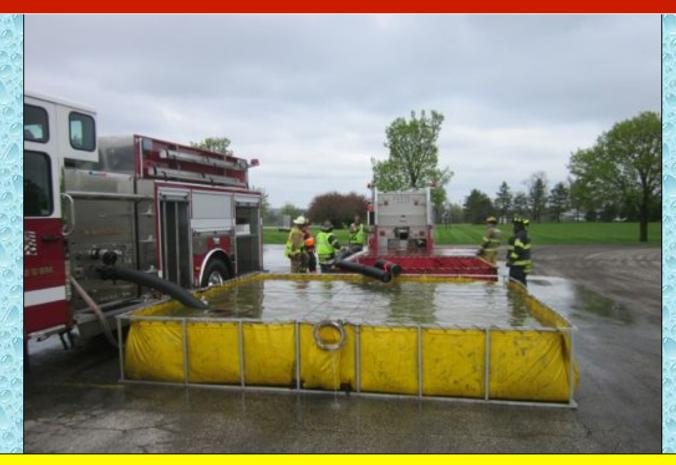
The primary dump tank was a 4,000-gallon tank from the Linn tender. The large tank created a huge reservoir from which the dump site engine could work.
