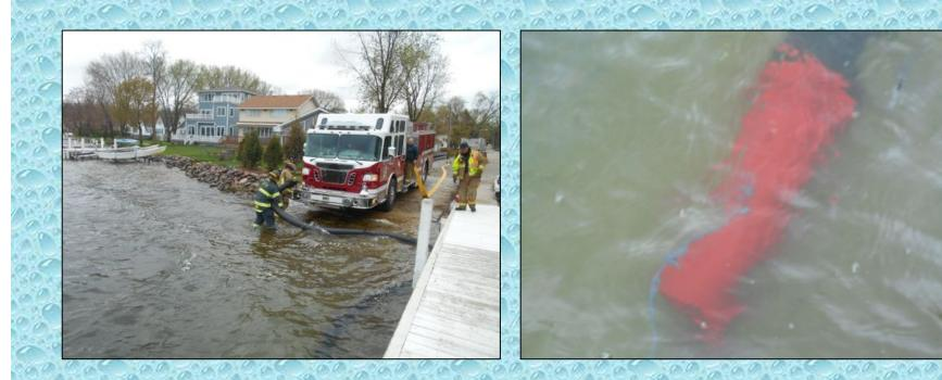
A suction intake valve problem forced the engine crew to move to using the pumper's front suction inlet. They still used the barrel strainer on the suction hose.
