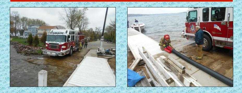
The lake had limited access but plenty of water to support a large scale loading operation. Linn Engine 3322 (2,000 gpm) is shown here arriving and getting set up as the fill site pumper. Because of the wave action on the lake, the float was removed from the strainer and the strainer was then submersed.
