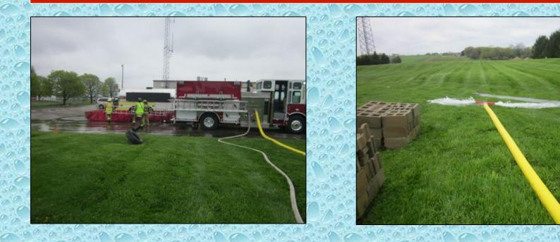
At the 15-minute mark, flow was moved to 500 gpm using a flow diffuser device supplied by a 5-inch line from Engine 3321.
