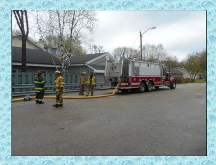
Tenders were loaded using 5-inch LDH. Engine 3322 drafted and pumped to an LDH manifold which was then used to control the loading of the tenders. The goal was to load at a rate of 1,000 gpm or more.
