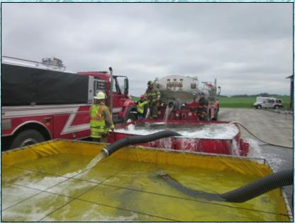
Around the 1-hour mark, a fourth dump tank was placed in-service and flow was moved to 1,250 gpm using Engine 3321's pre-piped deck gun. A Firovac low level strainer was used as the jet siphon in the fourth tank.
