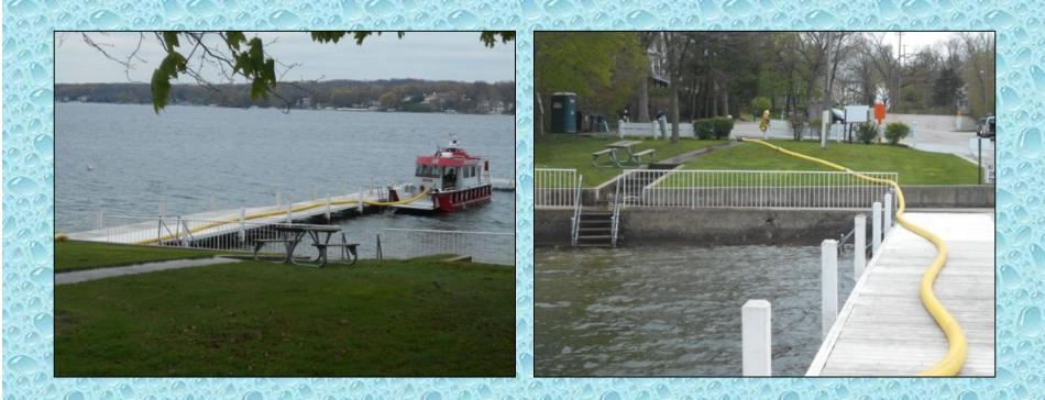
Linn Fireboat 3370 (2,000 gpm) ran quite an impressive fill site. They were in position and set up very quickly and loaded tenders at 1,000+ gpm – using a couple hundred feet of 5-inch LDH and two people.
