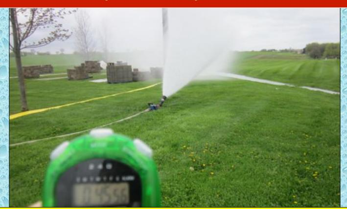
At the 45-minute mark, the 500 gpm flow was moved to a TFT Blitzfire device instead of the flow diffuser. The diffuser was being supplied by Engine 3321's high-flow discharge and the discharge pressure was a problem due to the size of the diffuser.
