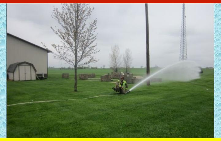
Water flow was started at 250 gpm at the 5-minute using a 2-1/2-inch attack line manned by one person.
