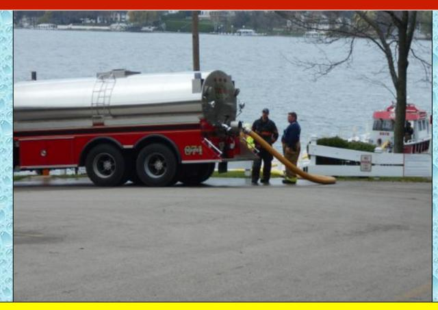
As in our other water supply drills in Wisconsin, the use of 5-inch LDH and standard fill connections made a huge difference at this drill in the ability to get the tenders loaded fast and back on the road.
