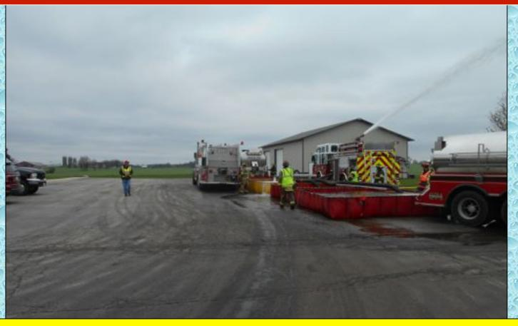
In the end, four dump tanks and two fill sites were used to support the 1,250 gpm flow.
