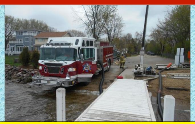
The Firovac vacuum tender also used this fill site to load. The vacuum tender's suction hose is seen on the right side of the photo. The vacuum tender self-loaded – there was no need for the engine or its crew to be involved in that loading process.
