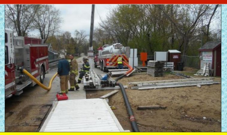
The vacuum tender (3,000 gal) is shown here self-loading while Engine 3322 awaits the arrival of a traditional tender at the fill site.
