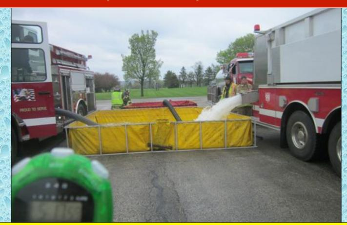
Shortly after the 5-minute mark was reached, water was dumped into the first dump tank and drafting operations commenced.
