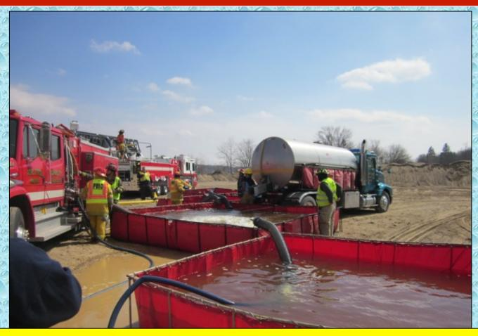
With flow now at 1,250 gpm, fewer tankers are seen at the dump site. Dixon's tanker is dumping its 3,000 gallons into the "primary" dump tank.
