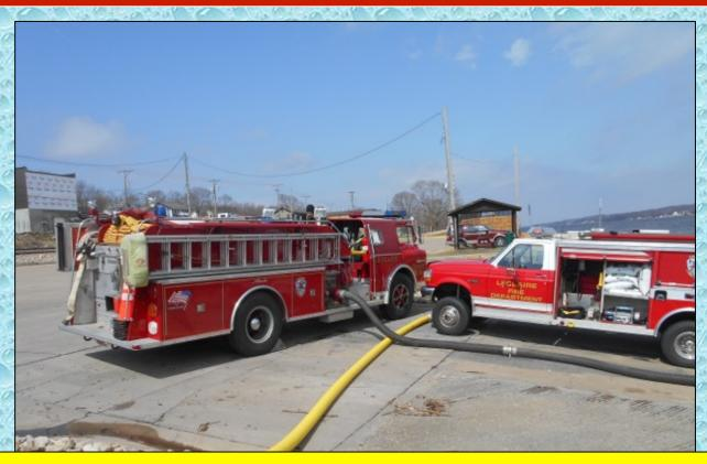
The pumper drafted through 40-feet of 6-inch suction hose after abandoning the attempt at using the dry fire hydrant. The suction hose was outfitted with a barrel strainer that was tied off to the boat trailer in order to keep it up and off the bottom of the boat ramp.
