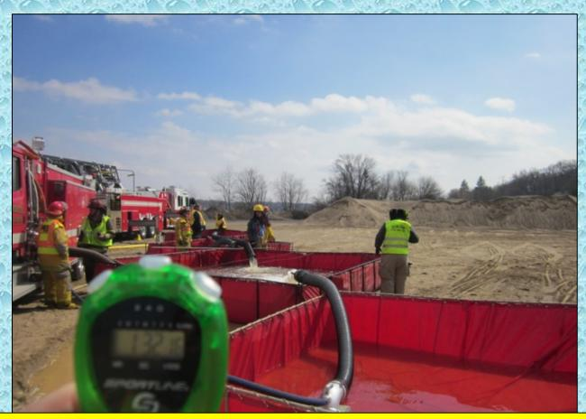
Things looked very slim at the 92-minute mark – 1,250 gpm flow and no tankers dumping! Flow had to be cut back to 1,000 gpm until a tanker arrived.
