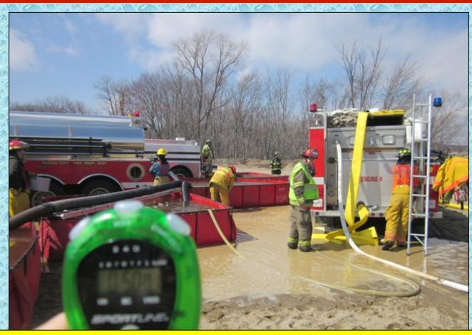
At the 48-minute mark, flow was moved to 1,000 gpm and at the 50-minute mark, a second supply line was stretched to the tower (the white 2-1/2" hose).
