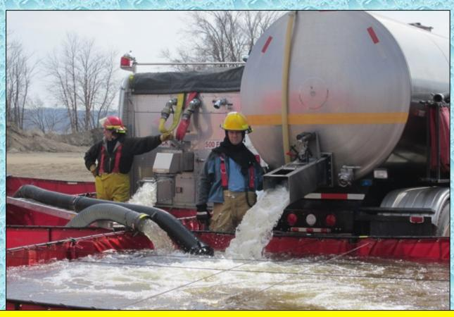
Dump site operations are well underway in this photo and supporting a 1,250 gpm flow. Crews worked very hard to keep the primary dump tank (3,500 gallons) full at all times – which made a huge contribution to the successful outcome.
