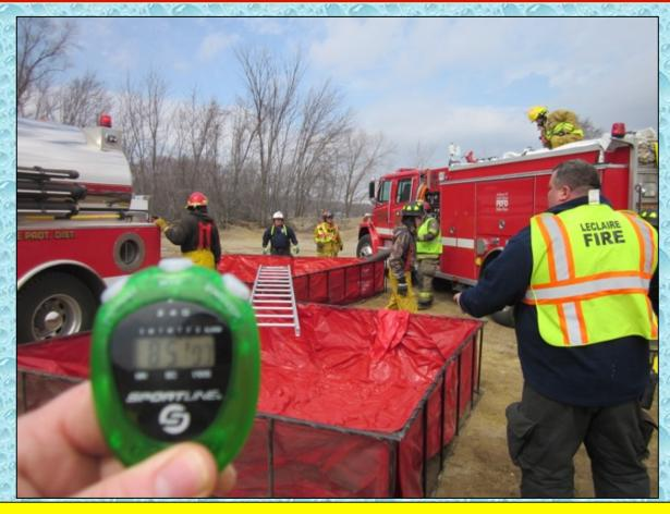
Right around the 9-minute mark, the first load of water (3,000 gallons) was dumped into the 3500-gallon dump tank and drafting commenced.
