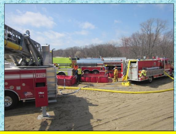
Units from the 2<sup>nd</sup> Tanker Task Force (2 tankers) began to arrive and water supply operations started to stabilize. Flow was moved to 750 gpm at the 30-minute mark.
