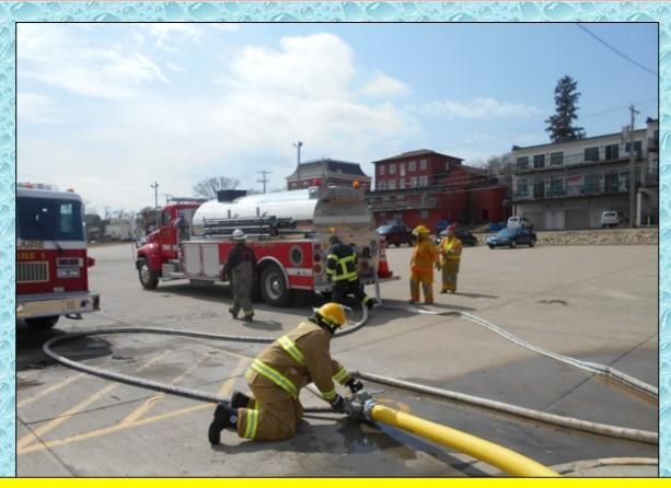
Most of the tankers had to be loaded using 2-1/2" hose because of a lack of fittings and adaptors. By keeping the 2-1/2" hose lines under 100-feet in length, fill times were acceptable when two fill lines were used.
