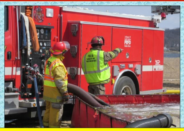
The Port Byron engine driver added a length of 2-1/2" suction hose to "boost" intake capacity so that the 1,250 gpm pumper could support the 1,250 gpm flow plus three jet siphons.
