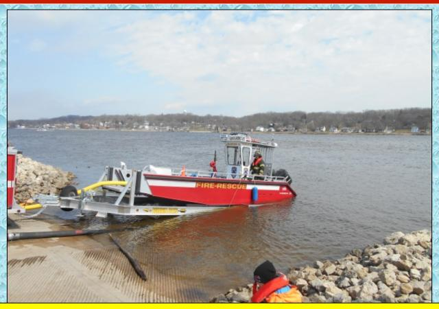
The fire boat drafted and supplied an LDH appliance via 100-ft of 5-inch hose. The boat was able to load tankers at a rate of at least 1,000 gpm because of the use of the 5-inch hose.
