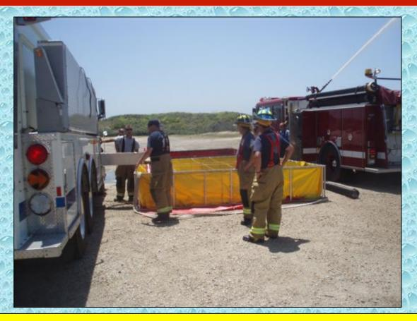
Because of the scarcity of equipment, the IC elected not to use a nurse tanker. All 4 tankers operated in the dump and run mode.
