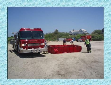
LC Engine 1 was the first-arriving unit at the Beach Club and assumed the role as the attack pumper. The stopwatch was started when the Engine driver applied the air brakes. Because of manpower and equipment shortages, we elected to use a wagon pipe to begin flowing water. Flows were verified via Pitot Gauge.
