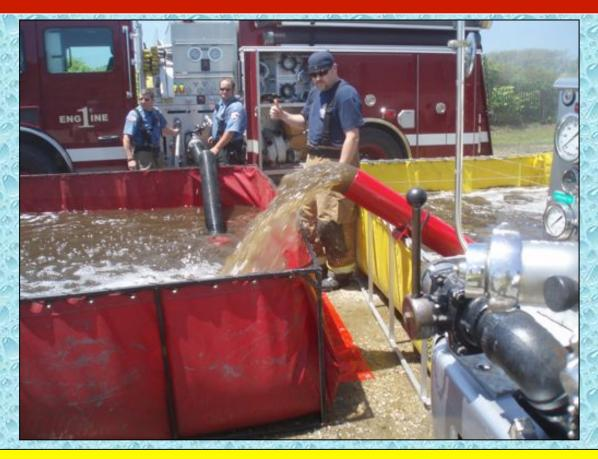
At the 7:00-minute mark, two dump tanks were down and the dump site was operational. The dump site engine switched from tank water to drafting – and dump site operations were underway.
