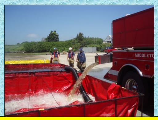
Middletown Tanker 1 dumps its 2500 gallons of water. After filling up the main tank, the tanker moved down to dump a little extra in the side tank. However, this crew soon moved on as the critical dump time of 90 seconds for this piece was just about over. Just about all tankers in this drill were able to dump about 90% of their load within 90 seconds.
