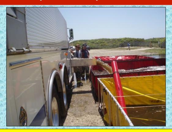
When using detachable dump chutes, it is often easier to just leave the chute at the dump site instead of trying to remove it and stow it in a compartment each time. Here LC Tanker 1 uses their detachable chute – but would leave it on the scene each time.
