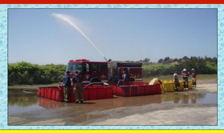
At about the 80 minute mark, the crews noticed that they were finally gaining ground and were able to go to a three tank operation at about the 100 minute mark. Flow was increased to 500 gpm at 110 minutes for the last 10 minutes of the drill.
