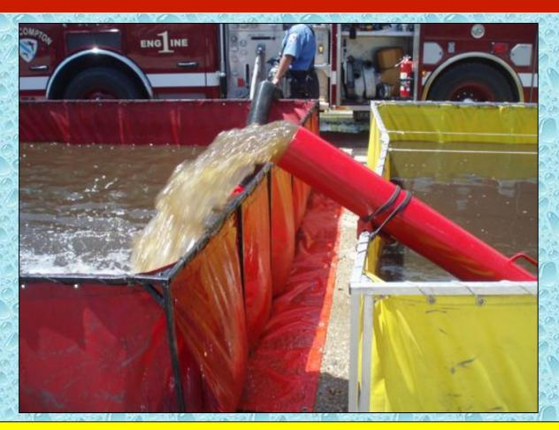
The flow from this Holley tube is a good, solid stream of water – which is exactly what is needed.
