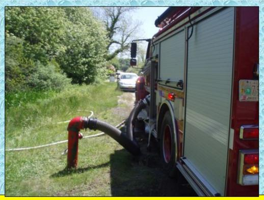
This wasn't the prettiest hook up but the crew was ultimately able to support a fill rate of around 900 gpm. To augment this the crew could have used another set of hard sleeves to the pond or used the booster tank (and refilled it when no tanker was waiting to be filled). However, there was limited manpower and folks were hustling.
