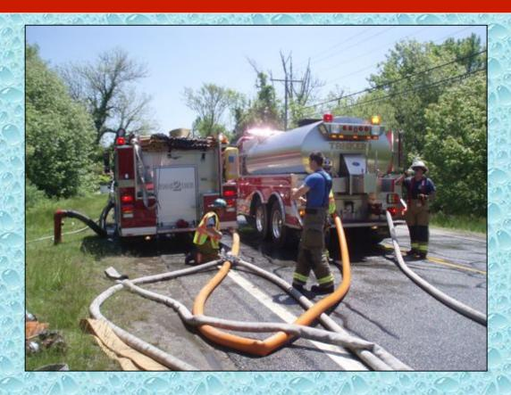
The crew had a hard time assembling the right adapters and hoses – but once they had the set up fixed, the fill times got better. They originally used a couple of 2.5" hoses – but switched over to 4" and 3" – which worked much better.
