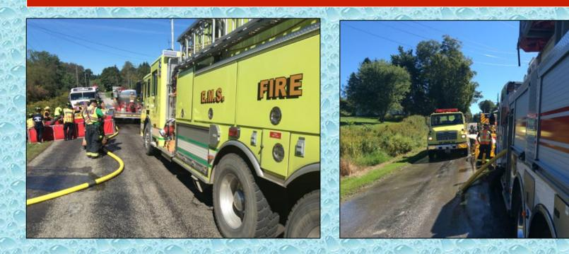
The narrow roadway forced the crews to use a single-lane arrangement of dump tanks....which was very realistic for the Kuhl response area.
