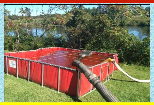
By keeping this dump tank full, every time East Meade's vacuum tanker arrived at the pond fill site the rig simply self-loaded and got back on the road to the dump site.
