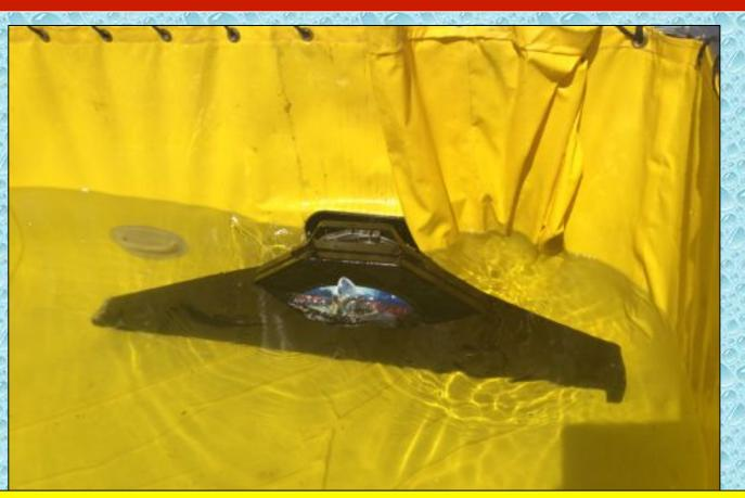
The Water Shark strainer allowed the engine/tanker to access almost all of the water in the dump tank while supporting a large flow.
