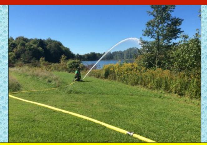
Water flow was started at 250 gpm at the 5-minute mark using tank water.
