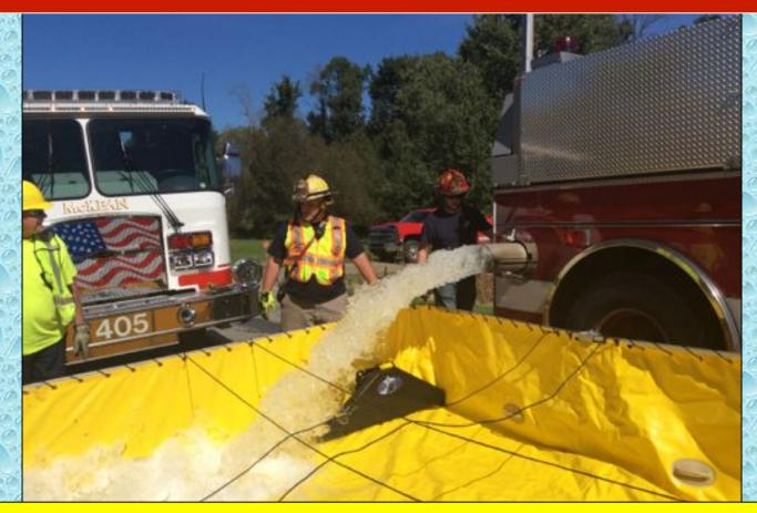
Engine/Tanker 405 set up to draft from the first dump tank using an ETT Water Shark strainer.
