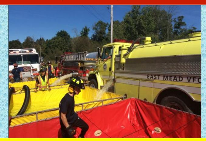
As additional tankers arrived the second and third dump tanks were brought on line. East Mead VFC's vacuum tanker is shown off-loading in this photo.
