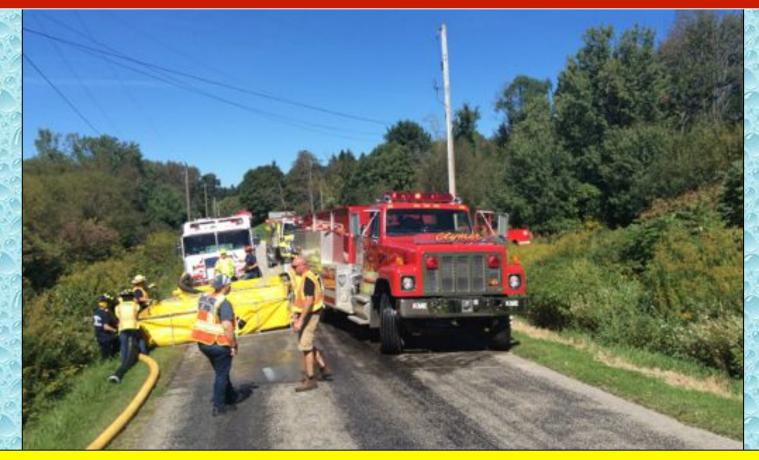
Around the 15-minute mark one dump tank was in operation and flow was moved to 500 gpm.
