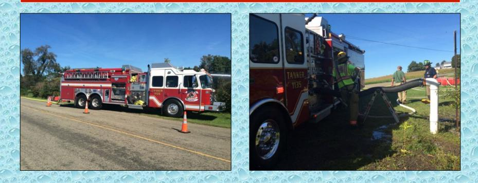
Union City Engine/Tanker 1135 (2000 gpm) supplied water for the second fill site which also included keeping a dump tank full for the vacuum tanker that was hauling water.
