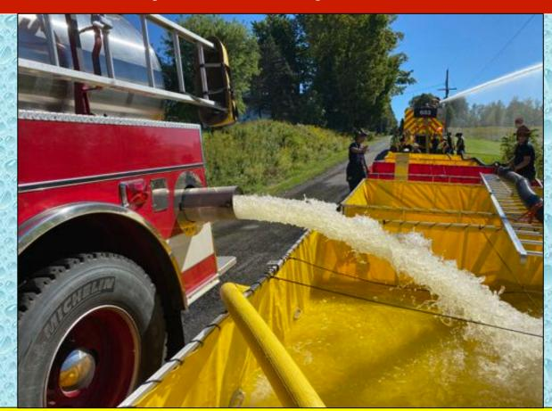
Flow eventually made it to 1000 gpm using four dump tanks and twin suction lines.
