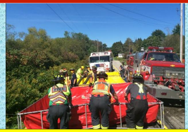
By the 19-minute mark, three dump tanks were down and one was in operation supporting the 500 gpm flow.
