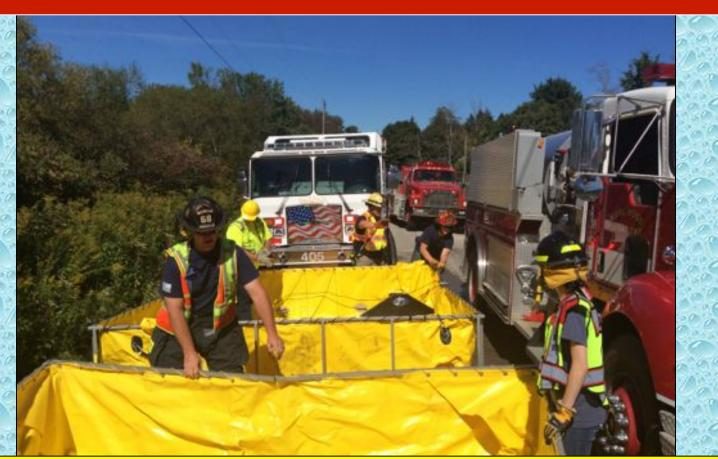
Crews worked to get two dump tanks down quickly once an additional tanker arrived in anticipation of a large-scale flow operation.
