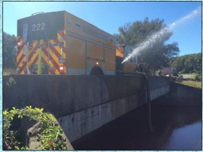
Harbor Creek Engine 222 (1500 gpm) drafted off a bridge and loaded tankers using LDH. A Hydra-Assist valve was used as the control valve on one of the loading lines.
