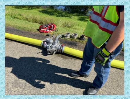
5-inch LDH was used to load the traditional tankers at the pond fill site.
