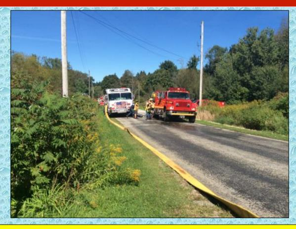
As nurse tanker operations are about to get underway the first-arriving tanker shows up at the dump site and crews work to gather and deploy a dump tank.
