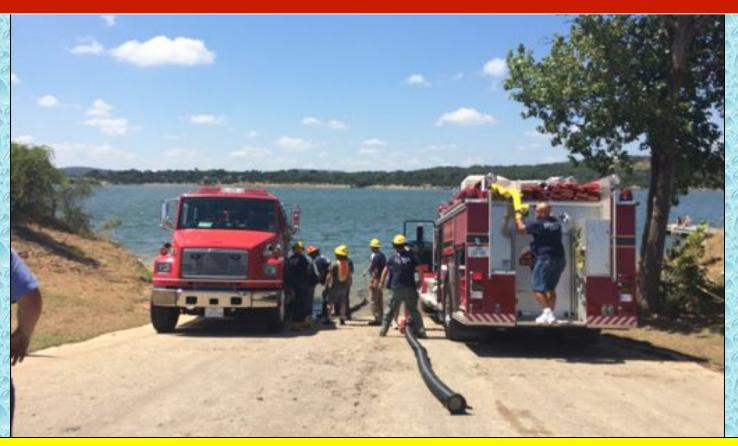
Waring Engine 86 (1,000 gpm) backed down the boat ramp and Sisterdale Engine 65 (1,250 gpm) nosed-into the lake. Each pumper drafted and supported its own tender loading station.
