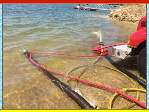
Multiple suction lines were used in order to bolster pump capacity so that tenders could be loaded at 1,000 gpm.
