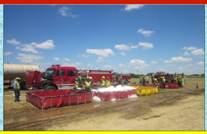
The final set-up, five dump tanks, two engines, and one 6,000-gallon nurse tender supported a 1,000 gpm flow.
