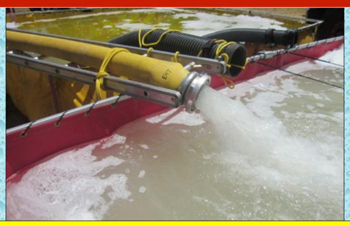
The 5-inch LDH was secured to the tip of the ladder and seemed to work just fine in supporting the water transfer operation.
