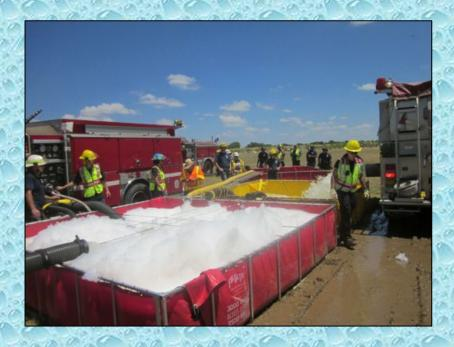
The 5-inch LDH was stretched over a 24-ft ground ladder. The ladder allowed the transfer of water from the 4<sup>th</sup> tank directly to the primary dump tank without first passing through the 3<sup>rd</sup> tank.
