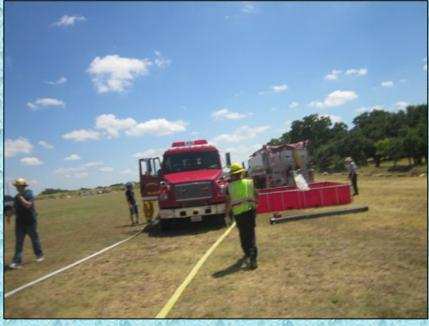
Kendalia Engine 77 (1,250 gpm) was the first-arriving unit and assumed the role as the attack pumper. Folks went to work setting up a portable monitor and a dump tank from the first-arriving tender – Boerne Tender 46 (2,500 gal). The stopwatch was started when the pumper came to a stop. Water flow was started at 350 gpm at the 2:30-minute mark.
