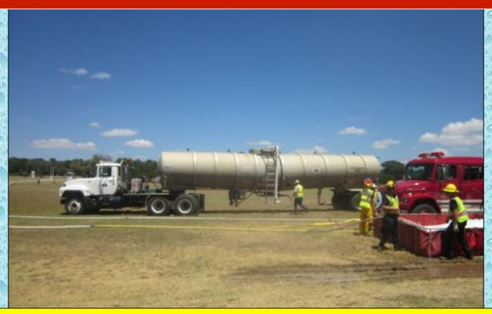
Flow was moved to 1,000 gpm at the 84 minute mark. Unit 9 arrived with its 6,000 gallons of water and prepared to support the operation by offloading into the primary dump tank using a nurse tender operation.
