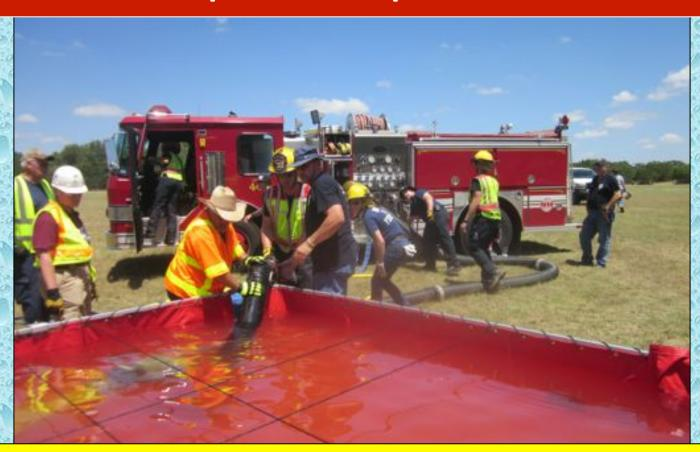
With the flow at 750 gpm and with a plan to move to 1,000 gpm, Boerne Engine 47 was brought in to help run jet siphons. The engine drafted from the 4<sup>th</sup> dump tank and supported the operation of two additional jet siphons.
