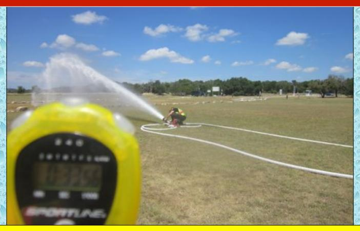
Flow was increased to 500 gpm at about the 34-minute mark. An adjustable gallonage portable monitor was used as the water flow device for the drill.
