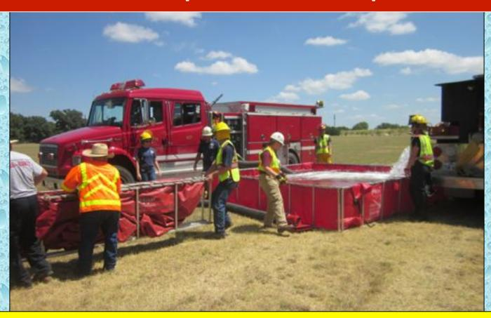
With the first dump tank in operation, the next dump tank was acquired from the second arriving tender – Sisterdale Tender 68 (2,200 gal).
