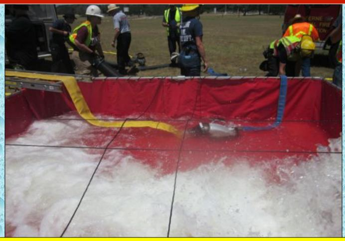
A TFT low level strainer being used as a jet siphon was equipped with a 25-ft section of 5-LDH in lieu of suction hose. The set-up worked just fine.
