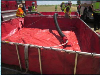
Comfort Tender 57 (2,500 gal) was the third tender to arrive on the scene. Crews were ready to use its water as soon as it arrived. The second dump tank was set-up and outfitted with a jet siphon device.
