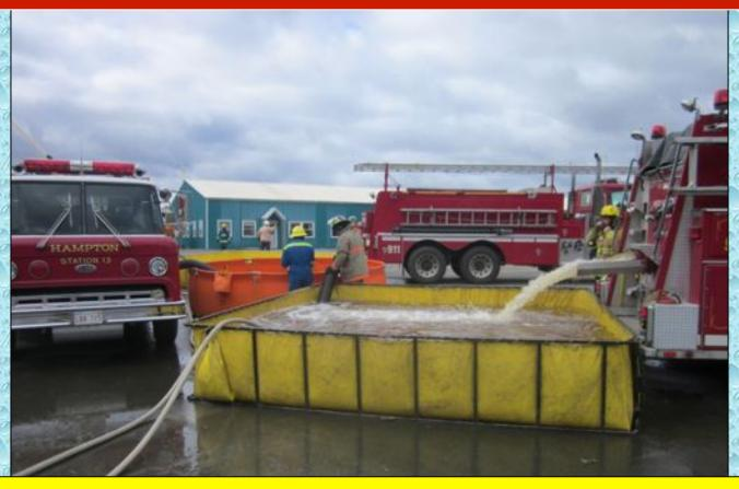
The dump tanks were positioned to best support the numerous tankers that could only dump off of the rear.
