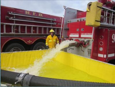
The tankers for the drill came in all different sizes and most of them could only dump off the rear of the vehicle. Fortunately, by using the parking lot for dump site ops, there was adequate space for maneuverability.
