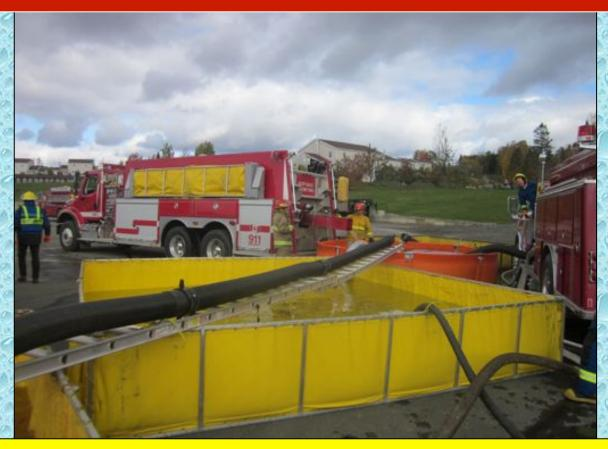
The jet siphon used in the fourth dump tank was rigged to "jump" the third dump tank so that all three jet siphons dumped their water into the primary dump tank (orange tank).
