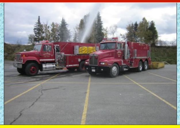
The dump tank arrangement allowed multiple tankers to dump simultaneously – which is what would be needed for a large fire at this facility.
