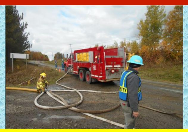
An LDH appliance was used as the control valve for loading the tankers. All the pump operator had to do was supply the appliance. Traffic control was important at this location and one person was dedicated to traffic control ops.
