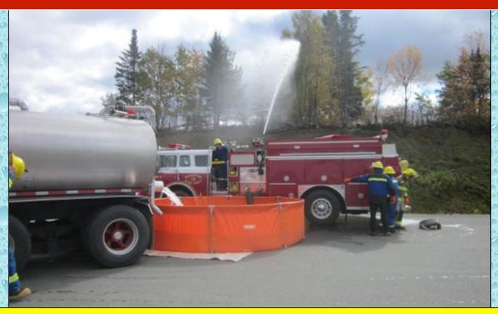
Water flow was started at 250 gpm at the 5-minute mark using the pumper's pre-piped deck gun. The plan was to expand operations to a 1,000 gpm flow so crews members developed a plan to acquire additional resources.
