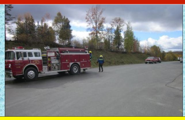
Jolly Farmer Pumper 1 (1,250 gpm) arrived on the scene and began setting up for attack pumper operations. The stop watch was started when the driver engaged the parking brake.
