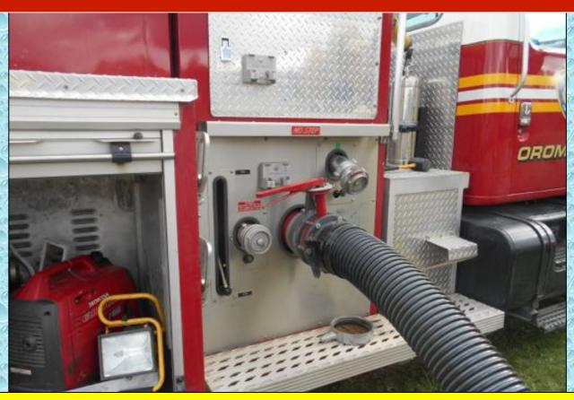
Note the use of a butterfly valve on the officer's side suction inlet. Best practice has all suction inlets equipped with some type of control valve so that operations can be easily switched between on-board tank water and drafting.
