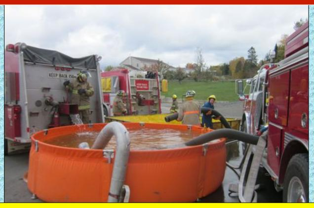
Meanwhile, another large dump tank arrived (2,500 gal) and the dump site crew deployed it. The plan was to eventually use at least three dump tanks to achieve the 1,000 gpm flow rate. Therefore, planning was very important as resources arrived. Flow was moved to 500 gpm at the 15-minute mark.
