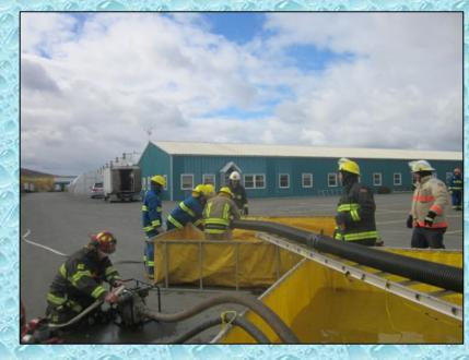
Three portable pumps were used to supply the jet siphons. The pumps varied in capacities and pressures but they all were able to support some level of water transfer. The ultra-high pressure pump worked well on the short transfer run while the higher volume pump worked better on the 30-ft run.
