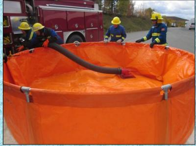
More fire brigade members arrived on the scene and immediately went to work setting up the first dump tank (2,500 gal). The tank was ready in about 4 minutes, just in time for the arrival of the first tanker.
