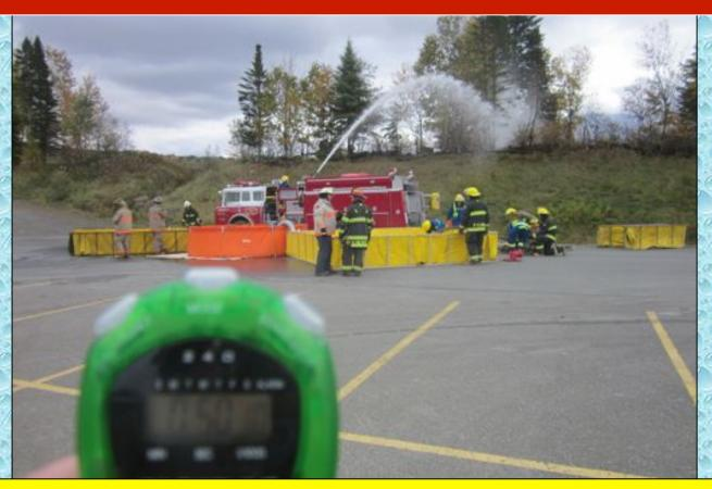
At the 50-minute mark, the three dump tank operation was supplying the 1,000 gpm flow without much difficulty other than waiting on tankers. The crew decided to place a fourth dump tank into operation.
