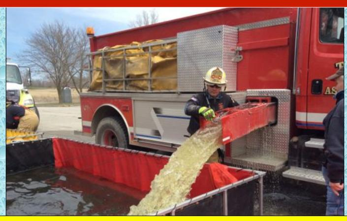
All of the tankers could side dump which made the single-lane dump tank arrange work quite well. The white line on the dump chute indicates when it is time to "cut and run" for another load of water.
