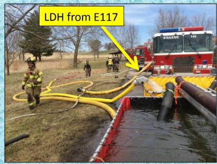
North Liberty Engine 117 arrived at the dump site and their 1,000 gallons of water was needed. Thus, the operator positioned the rig out of the way and pumped off the water using a 5-inch hose line feeding into the main dump tank.
