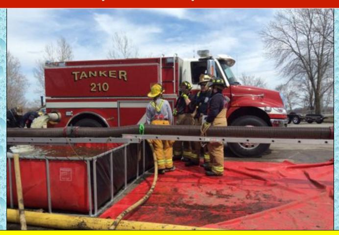
The dump site crew spread out the third and fourth dump tanks in order to allow two tankers to off-load at the same time.
