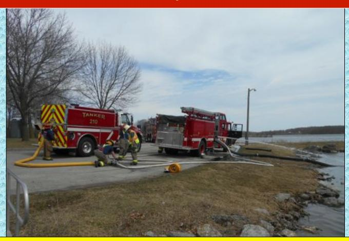
Engine 117 had no high-flow discharge so the crew used two, 2-1/2-inch lines to feed an LDH appliance and then load tankers using 5-inch LDH.
