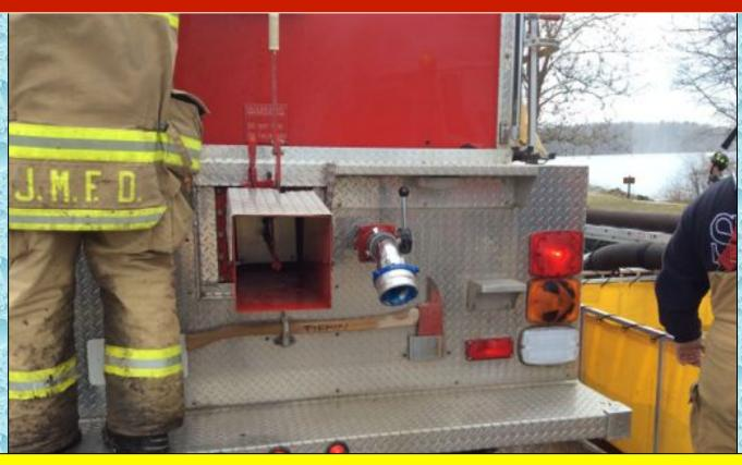
At the fill site, one of the loading stations had a "fill site package" that had sets of 4-inch cam lock fittings. As tankers cycled through the fill site, they were outfitted with the male cam lock fitting so that the next loading session would go faster. This was another great idea that worked very well!
