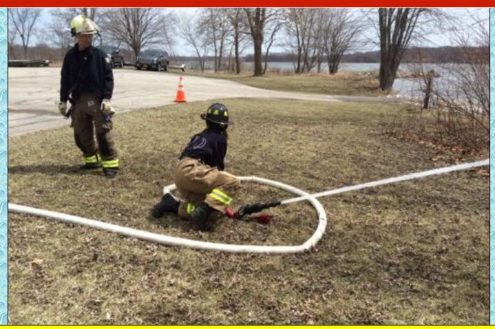
Water flow was started at the 5-minute using an Elkhart RAM monitor. Flow was started at 250 gpm.
