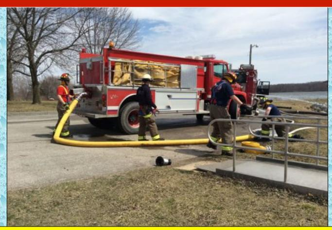
Loading tankers at the 1,000 gpm flow rate was the goal of this fill station and they did just that!
