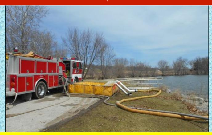
Coralville Engine 72 (1,000 gpm) used two, Turbo Draft devices to supply water back to a dump tank. The pumper then drafted and loaded tankers at just under the 1,000 gpm goal.
