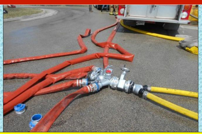
The 4-inch hose with cam locks sped up the loading process while also being manageable in terms of making and breaking connections. The manifold also supplied a 5-inch fill hose for those tankers loading using 5-inch hose.
