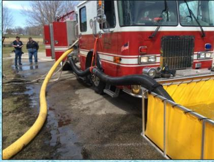
Around the 1-hour mark, the dump site crew worked to place a second, suction line in operation for the dump site engine. Because Engine 141 was outfitted with suction inlet control valves (Hale MIV), the second suction line was able to be brought on-line without an interruption in flow.
