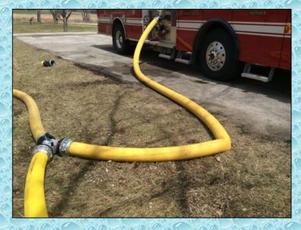
The supply line feeding the attack engine (E132) was outfitted with a Task Force Tips clappered siamese. Once the dump tank operation was ready, the supply engine began pumping its side of the siamese and nurse tanker operations were then stopped.
