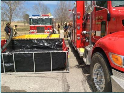
The folks wanted to try the single-lane dump tank arrangement...even though they only had square shaped tanks. The goal was to build out a 3 or 4 dump tank arrangement in front of the supply engine.
