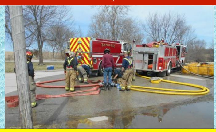
Rodger Sill from the Stanley FD brought a "tanker loading package" to use. The package consisted of an LDH manifold, some valves, and most importantly, 4-inch hose with cam lock fittings to speed up the loading process. Coralville Engine 72 supplied this operation.
