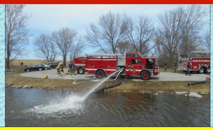
North Liberty Engine 117 established a second fill site after pumping off its water at the dump site. The crew drafted directly from the lake and loaded tankers at a fill rate just over 1,000 gpm.
