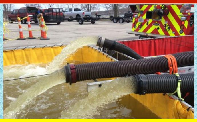
By adding in the second suction intake, the dump site pumper (Engine 141) was able to improve its 1,250 gpm capacity and thus supply the attack engine AND supply four jet siphons...three of which are shown in this photo. All three jet siphons have excellent looking output streams.
