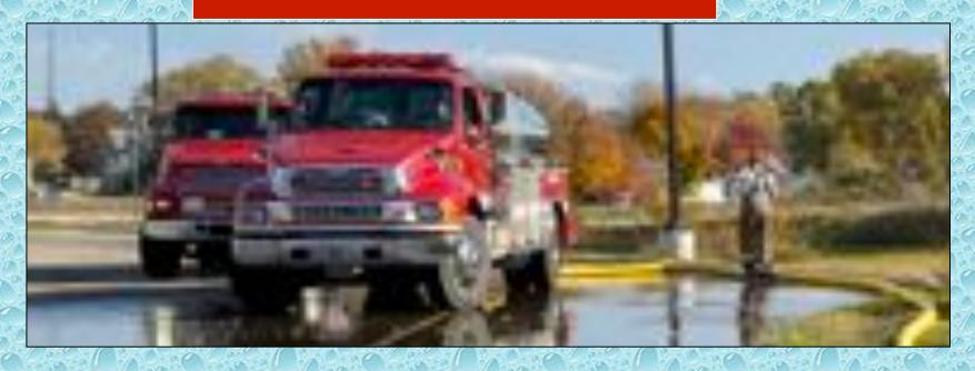
Two fill lines allowed a second tender to be connected and start filling within a few seconds after the first tender was finished filling. It is best practice to fill one tender at a time (due to pump capacity) but this set-up assured that there was no time wasted inbetween tender fills due to having to unconnect and reconnect fill lines. There was plenty of space for tenders to drive in and position.
