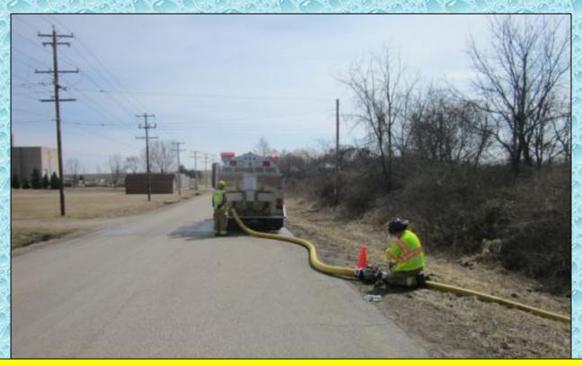
A 5-way LDH manifold was used as the loading control device. One person manned the valve and one person made the connection to the tenders. This was a very efficient set-up and most tenders were filled at a rate approaching 1,500 gpm.
