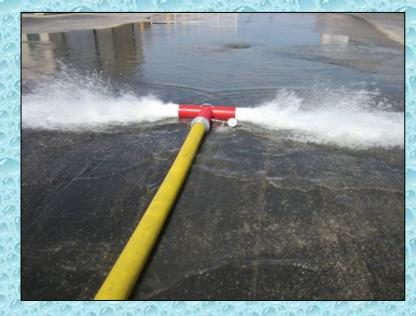
At the 15-minute mark, water flow was moved to 500 gpm using the flow diffuser device with built in pitot tube for flow measurement.
