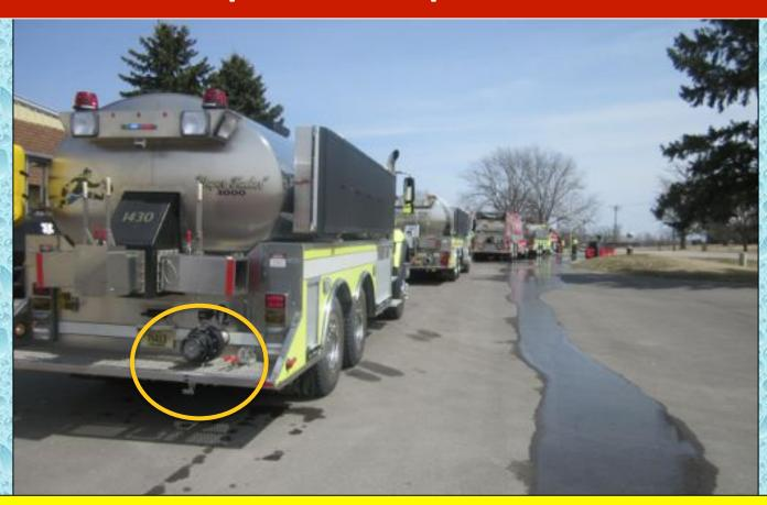
What made the drill such a success was the ability to reload the tenders. All of the tenders in the mutual aid system are equipped with a 5-inch LDH direct fill line which meant the rigs were filled at a rate of 1,000 gpm or greater.
