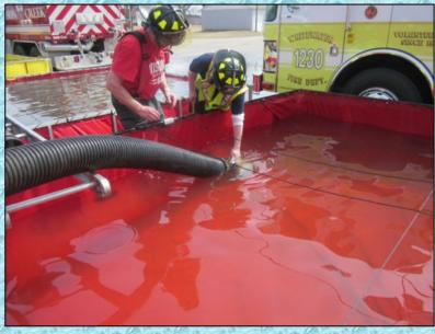
This changeover occurred about 56-minutes into the drill. The strainer on the driver side suction line was also changed out for a better performing one. Once this was done, water flow was increased to 1,300 gpm and then finally to 1,750 gpm about 14 minutes later - where it was sustained for the remainder of the drill.
