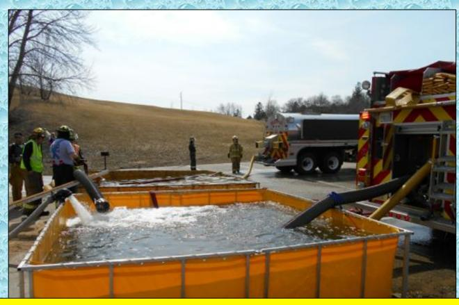
By using two dump tanks, sufficient capacity was available to fill the large tenders when they arrived. During the period in between tenders – the dump tanks would refill.
