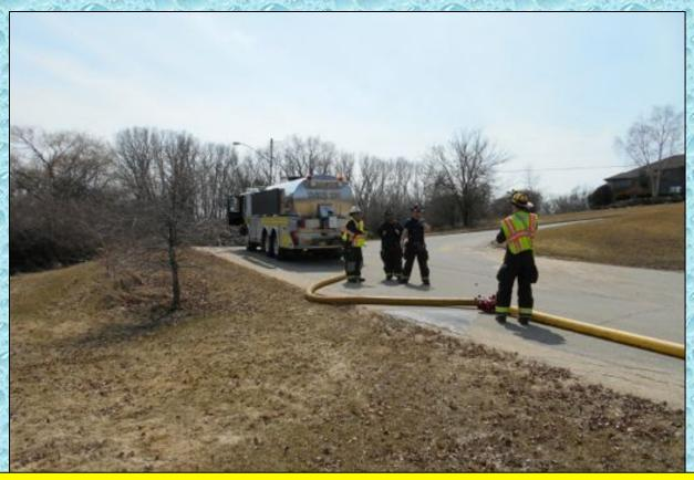
The fill site operation initially used a single, 5-inch line to a manifold as the loading station supply.
