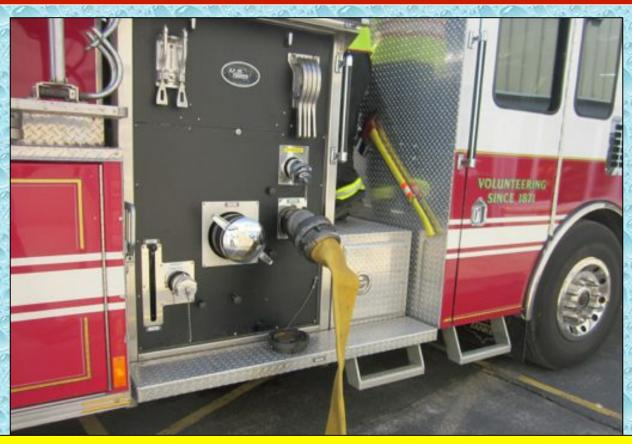
A 5-inch line was deployed to a hose diffuser device so that flow could be increased when the 15-minute mark was reached. The line was connected to the 2,000 gpm pumper's high-flow discharge.
