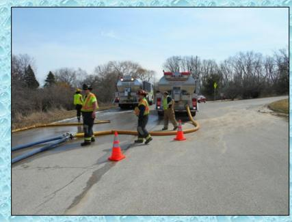
With the 2,000 gpm pumper now capable of maximum capacity, the crew set up a second loading operation so that two tenders could be loaded at the same time at a rate of 1,000 gpm each.
