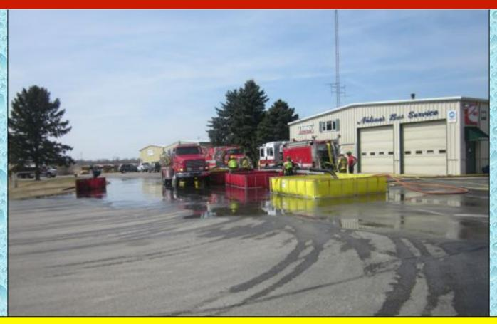
With the flow now at 1,750 gpm, this photo at the 85-minute mark shows a single tender at the dump site – which was the norm for the remainder of the drill.
