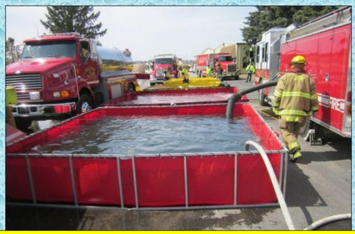
Four dump tanks are now deployed around the 22-minute mark and three are in operation. Additional alarms are struck bringing more tenders.
