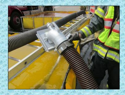
One of problems that arose was the inability to "get water into the pumper." The pumper was drafting from both the driver side and front intakes using 6-inch suction hose. The problem was the low level strainer selection. The strainer on the front intake suction line (left) was exchanged for a better performing strainer (right).
