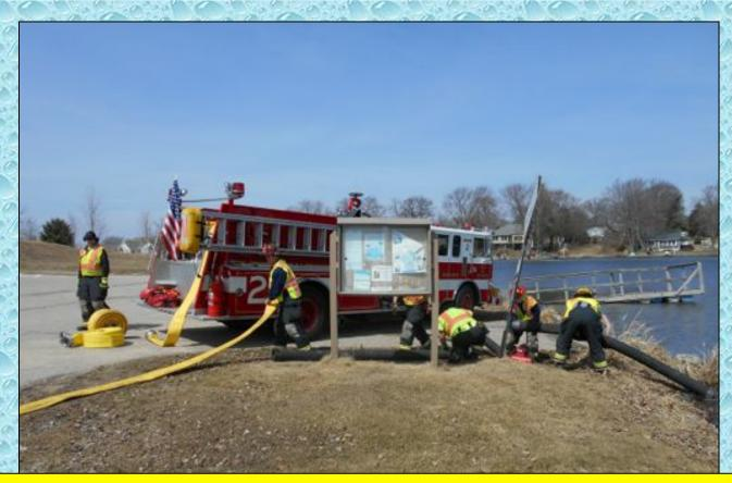
Delavan Engine 2 (2,000 gpm) operated this fill site. The crew is seen here during the initial set up of the site. This site was the first fill site established – so the crew had to work quickly in order to be ready for the first empty tender.
