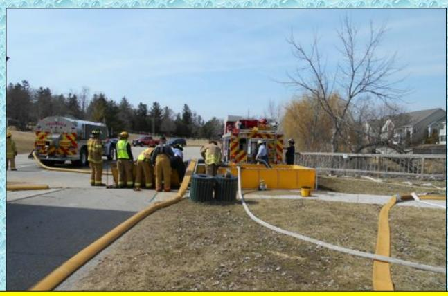
Ample space existed to run the supply set-up and the loading set-up. The use of 5-inch LDH made a big difference in being able to quickly load the tenders.
