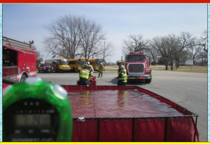
A second dump tank was deployed around the 7:00 minute mark in preparation for rapidly expanding the water flow.
