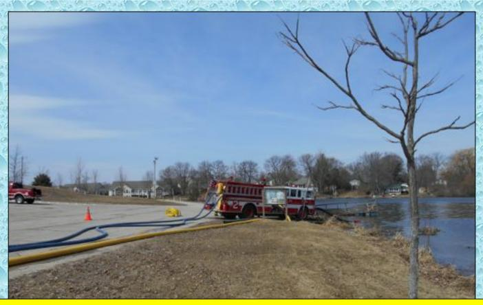
After the site was operational and a few tenders had been loaded, the crew went to work expanding the operation by adding a second suction line – the front intake.
