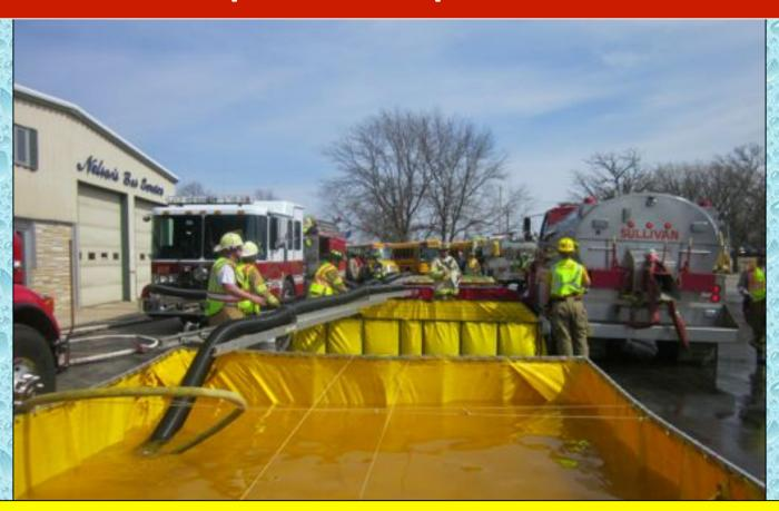
This photo (67-minute mark) shows the complexity of the dump site operation. Ixonia Tender 7 was brought in to help transfer water since the Whitewater pumper was flowing over 2,000 gpm - given the multiple jet siphons in use.
