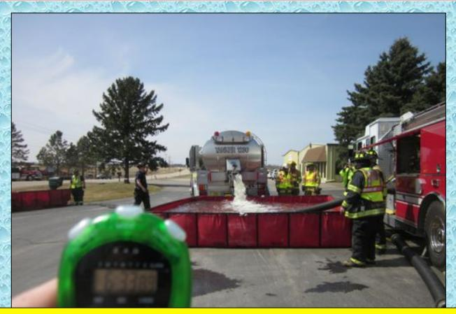
The dump site crew did an awesome job and dump site operations were underway at the 6:33 minute mark. A 250 gpm water flow had already started at the 5:00 minute using a portable ground monitor device.
