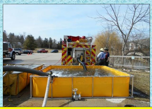
Because of the 1,750 gpm water flow back at the dump site, two dump tanks were used at this fill site in order to load tenders as fast a possible.
