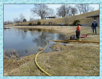
The third fill site used a combination of a portable pump and a Turbo Draft to to supply water to portable dump tanks from which Cambridge FD Engine 2 (1,500 gpm) drafted and loaded tenders.
