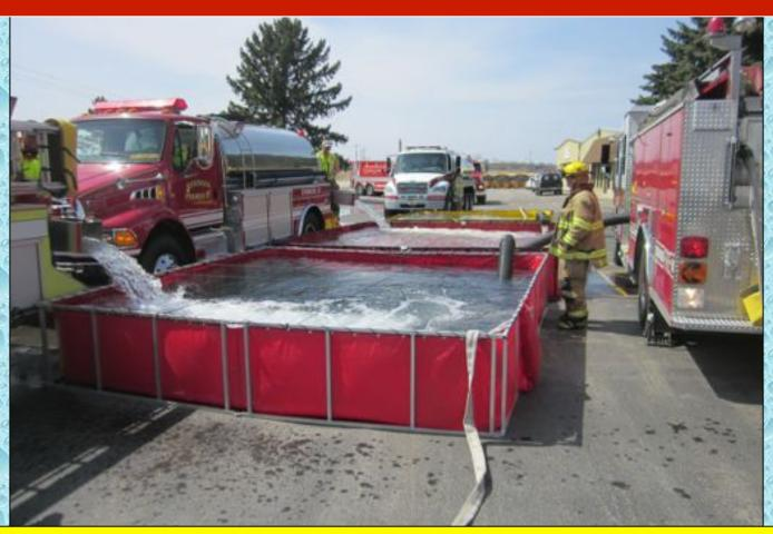
Just a few minutes later (17-minute mark) flow was increased again to 750 gpm and a third dump tank was placed in operation.
