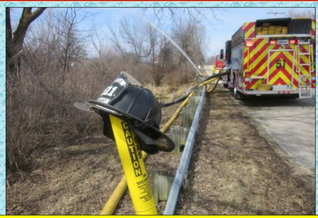
Turtle FD Engine 51 with a crew of three personnel operated this fill site. The 2,000 gpm pumper drafted from the creek and supplied a 5-inch line for the loading operation.
