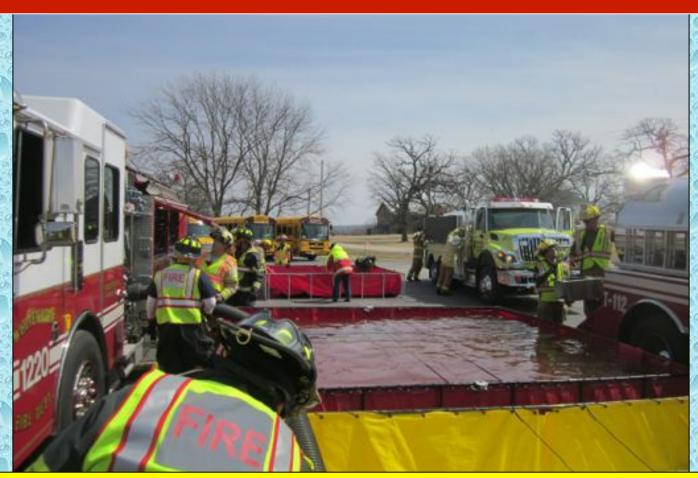
As additional tenders arrived on the 1<sup>st</sup> Alarm, crews grabbed more dump tanks. The operation would eventually grow to a 5-dump tank operation.
