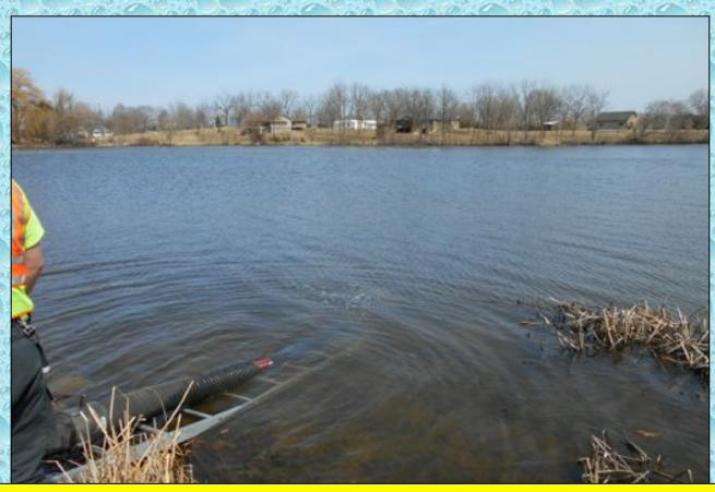
A barrel strainer and 6-inch suction hose was used to supply this operation. A roof ladder was used to keep the strainer off of the bottom of the lake.
