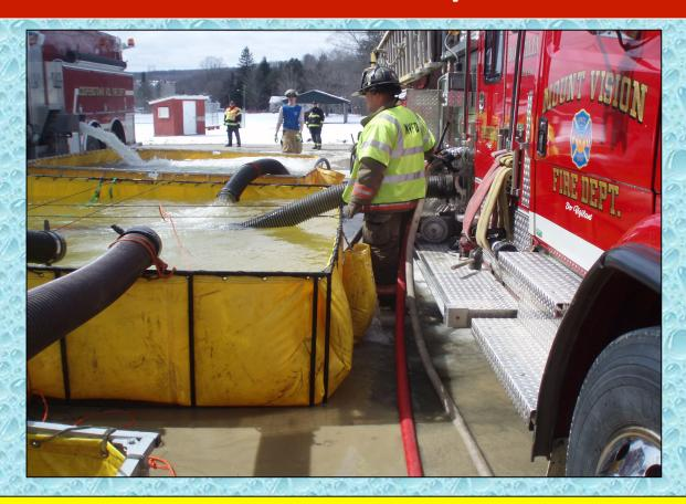
The dump site crew used a gated-wye to supply two jet siphons – and later on a third. Doing so let the pump operator concentrate on other operations instead of having to open and close valves for jet siphon ops.
