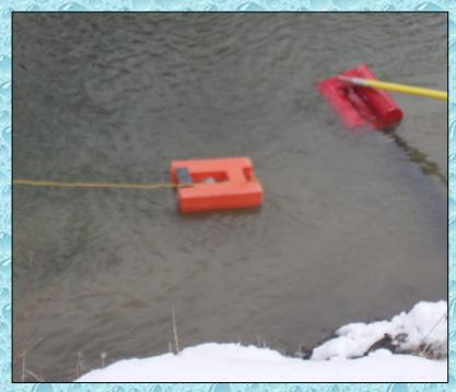
The crew from Pindars Corners worked very quickly and had this fill site operational in less than 10-minutes. This engine has a 1500 gpm pump but the crew anticipated a lower flow due to the use of the front intake and a 12' lift. With the use of the second "pony" suction this engine was able to fill at close to 1000 gpm.
