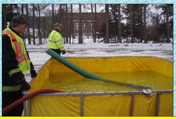
When using detachable dump chutes, it is often easier to just leave the chute at the dump site instead of trying to remove it and stow it in a compartment each time. Here Hartwick Tanker 821 leaves their cam lock adapted dump sleeve in the tank for repeated use.
