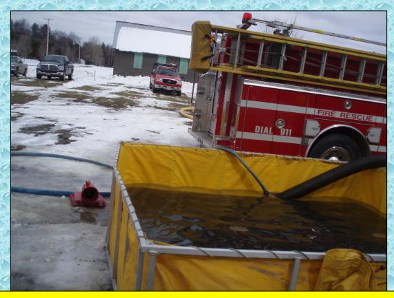
Water transfer operations were now underway. Here, the crew elected to use a simple jet siphon instead of the low level strainer. This crew stated based on their previous experience the jet siphon worked better.
