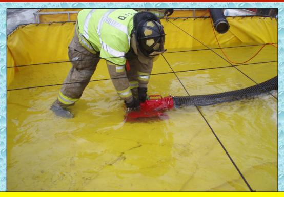
A Kochek low-level strainer w/jet siphon was used by the dump site engine. At low levels it doesn't work so well with the plug out of the jet siphon supply inlet. Fortunately both the attack engine and dump site engine had filled their booster tanks - so flow was uninterrupted. This strainer also proved problematic later when flow was increased to 700 gpm.
