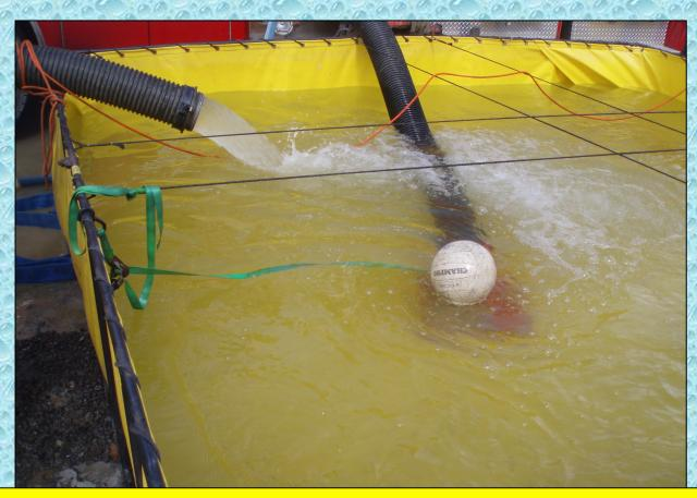
The flow from this 6-inch jet siphon is a good, solid stream of water – which is exactly what is needed.
