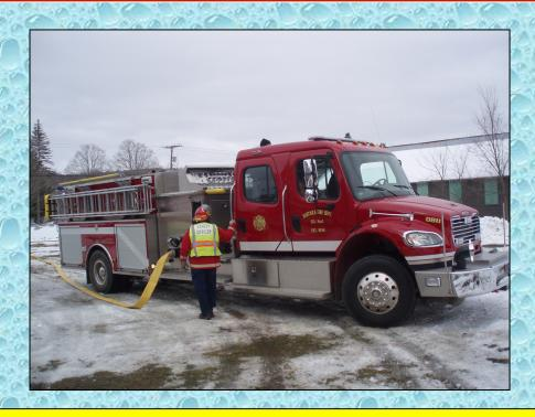
Hartwick Engine 811 was the first-arriving unit at the school and assumed the role as the attack pumper. The unit laid out 100-feet of 5-inch supply line from the main parking area. The stopwatch was started when the Engine driver applied the air brakes.
