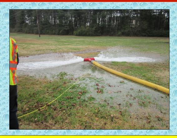
The crew stretched 100-feet of 3-inch hose to a Hose Monster flow diffuser that served as the means by which all water flow would be measured. The diffuser simulated the use of a portable master stream device.
