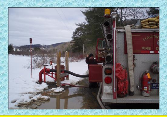
The crew from Hartwick Engine 812 struggled to set up quickly due to only having two personnel. However, the pump operator was able to achieve a flow of just over 1000 gpm with a 1000 gpm pump and a 5" sleeve – he went "old school" and used his booster tank to supplement his flow during tanker fills. Of course, the three foot of lift didn't hurt either.
