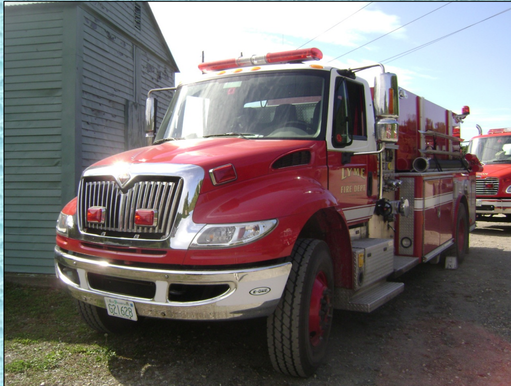
Lyme FD – Tanker 1 – 1,000 gpm w/ 2,000 gal tank
