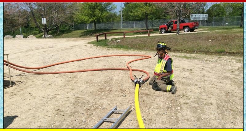
Because water transfer operations are so important at a large operation like this one person was placed in charge of controlling two of the jet siphon devices. This person never left his post and made sure that the primary dump tank was kept full of water.
