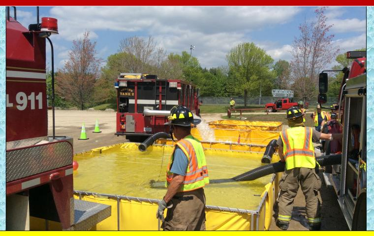
By the 20-minute mark flow is moved to 500 gpm. Three dump tanks are down and two are in operation.
