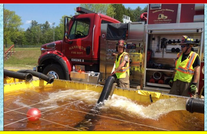
Engine 2 (1500 gpm) eventually placed a 2-1/2-inch suction line in-service which allowed the rig to support a 1000 gpm flow while pumping four jet siphon devices.
