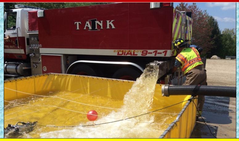
Dumping into the primary dump is not the preferred choice but there were a couple times that was needed in order to maintain water flow. An additional jet siphon was placed in-service which resolved the issue.
