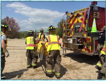
Harrison Engine 2 arrived on scene and immediately went to work setting up to supply a simulated fire attack (HoseMonster) using the rig's 3000 gallons of water. While 200-ft of 4-inch LDH was being stretched another crew worked to deploy the Engine's 3000-gallon dump tank in preparation for dump tank ops.
