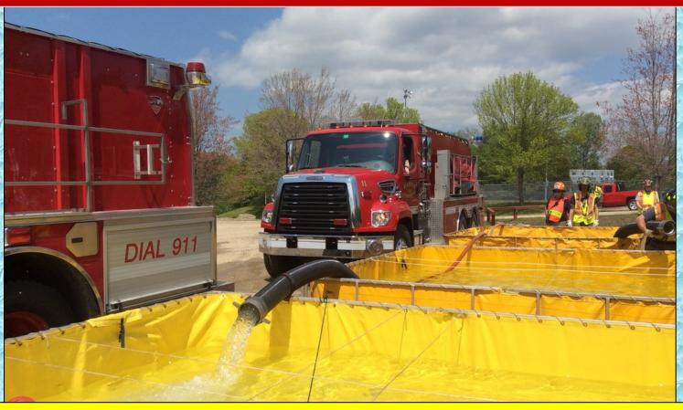
As additional tankers arrive the third dump tank is brought on-line. Flow is moved to 900 gpm around the 54-minute mark.
