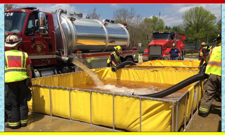
Around the 15-minute mark two dump tanks are down but only one in operation. Bridgton Tank 4 (3500 gal) dumps its first load of water.
