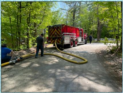
Brownfield Engine 1 (1500 gpm) drafted from the pond to support this tanker loading site.
