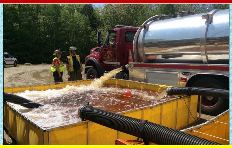
Bridgton Tanker 4 was the only vacuum tanker in the shuttle and did a great job hauling water during the drill.
