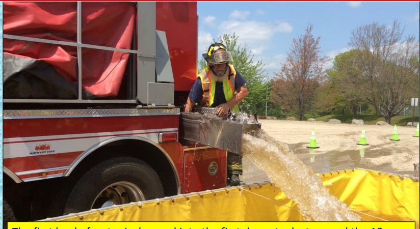
The first load of water is dumped into the first dump tank at around the 10-minute mark and drafting operations commence very soon afterward..
