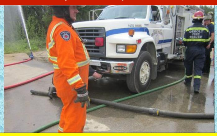
Realizing that they wanted to maximize their flow capability from this engine, the crew began hooking up additional suction lines so that more water could be taken into the pump. Engine 1402 is equipped with dual, 3-inch front suction intakes. The crew is shown in this photo connecting to one of those intakes.
