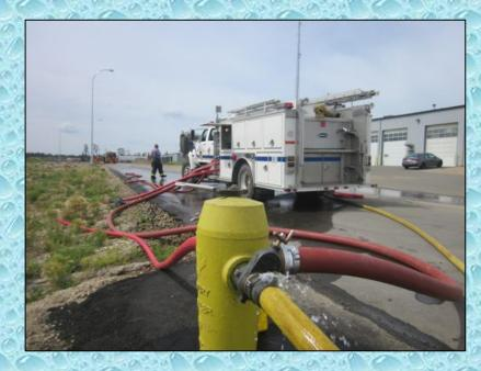
Engine 11 (750 gpm) and a crew of four personnel operated one of the fill sites using this fire hydrant. The crew did a very good job of supplying water to the engine using dual, 65mm lines and a 100 mm line. The engine crew loaded tenders at over 4,000 lpm and they worked like a "pit stop crew."
