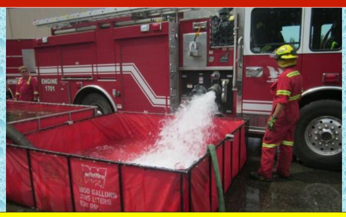
Engine 1701 "hopped" into the shuttle operation by hauling loads of water (4,000 liters). The rig is equipped with a high-flow discharge and the crew used that discharge to pump off the water. They did this when no other tender was available to dump – that way the engine did NOT block out a tender.
