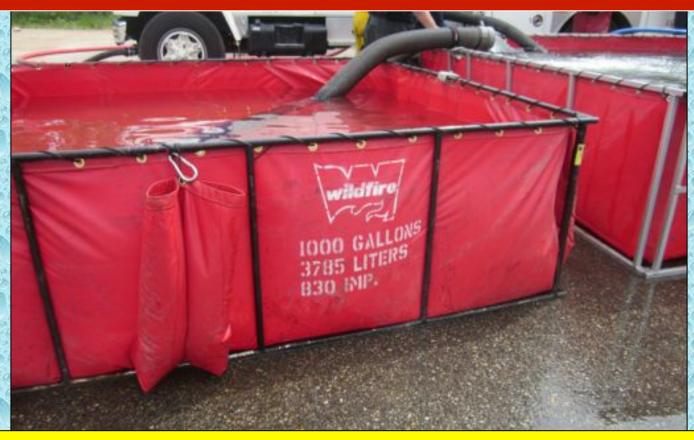
A third dump tank was added around the 20-minute mark. Flow was increased to about 2,000 lpm at the 31-minute mark and then again to about 3,000 lpm at the 44-minute mark.
