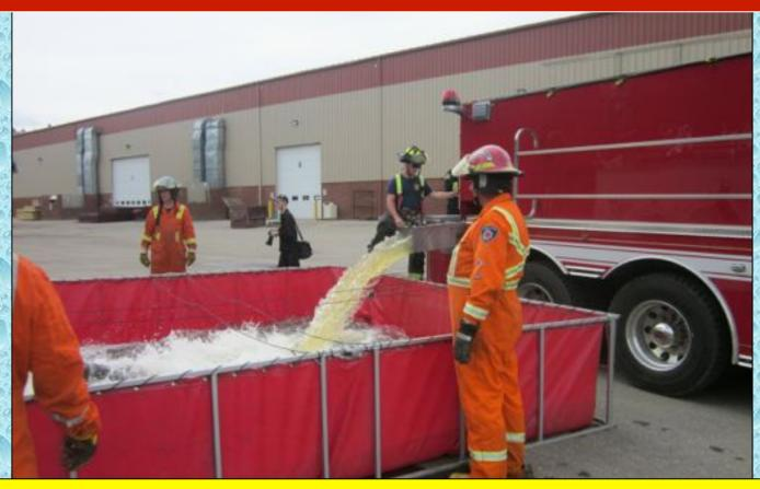
Tender 1701 was the first tender to arrive on the scene and it arrived right behind Engine 1402. The crew deployed the tender's dump tank and was ready to offload its 14,000 liters (3,500 gal) of water once the engine was ready to draft.
