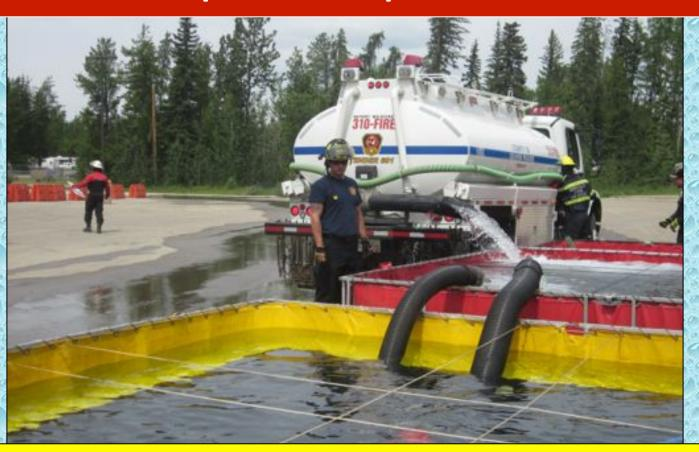
In order to support the 750 gpm flow, multiple jet siphons were needed to transfer the water. In all, four jet siphons were used – all supplied by Engine 1402!
