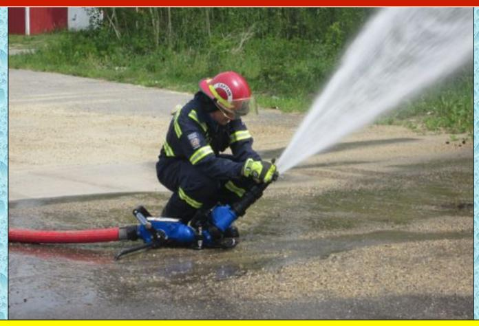
A handheld pitot tube was used to accurately measure the flow during the drill.
