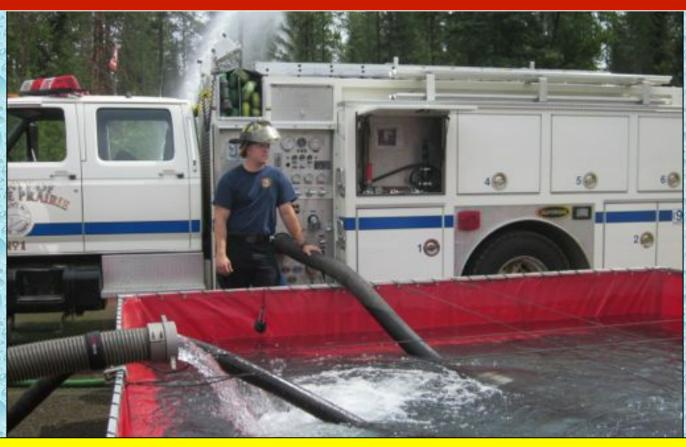
Engine 1402's operator was kept quite busy and the pumper was used to its maximum capability. A third suction line was placed into service (not shown here) later on to gain additional intake capability.
