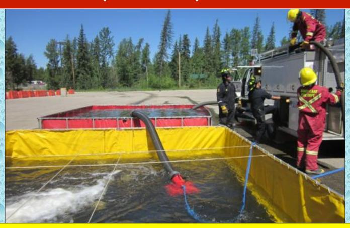
Just shy of the 14-minute mark, two dump tanks were down and in operation. Crews were working to expand the operation further in anticipation of using a third dump tank and increasing the flow.
