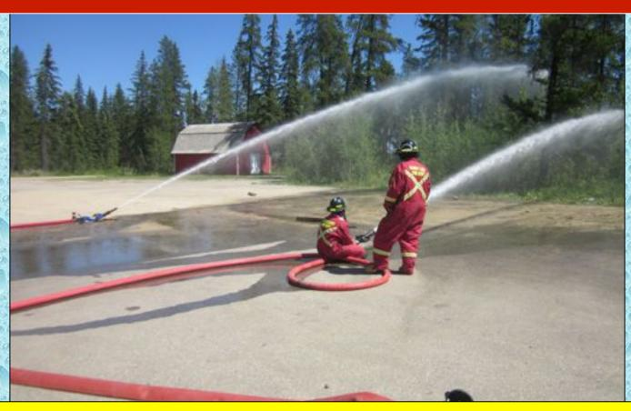
At the 47-minute mark, flow was increased to 600 gpm using the Blitzfire and a 65mm attack line with a variable flow nozzle set to 250 gpm.
