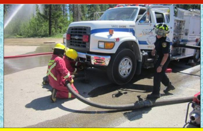
Engine 1402 had an interesting intake arrangement, in addition to the traditional steamer inlets, it also had two, 3-inch suction inlets on the front. The crew is shown here adding a 3-inch suction to bolster the 750 gpm pump's ability.
