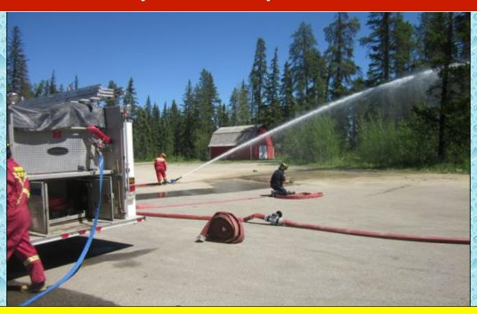
At around the 20-minute mark, flow was moved to 400 gpm using the Blitzfire equipped with smooth bore tips so that a handheld pitot could be used to accurately measure flow..
