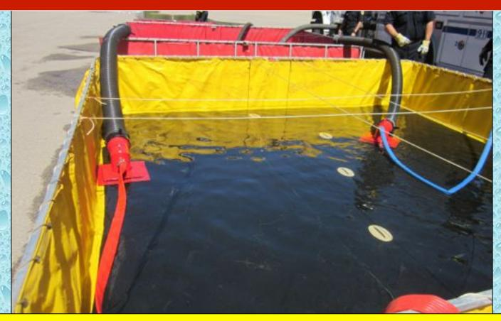
In order to transfer water at a sufficient rate, dual jet siphons were needed between the two, large dump tanks.
