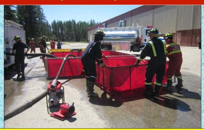
A third dump tank was eventually deployed, however it was just 1,000 gallons in size. A portable pump was also deployed to run a jet siphon, but the pump could not generate sufficient pressure to operate a jet siphon.
