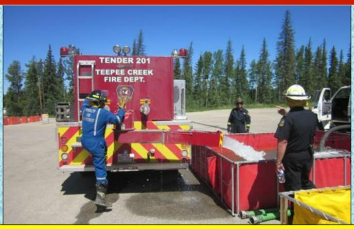
Tender 201 was the second tender to arrive on the scene and its crew helped to deploy its 3,500-gallon dump tank and then dump the tender's 3,500 gallons of water before heading to the fill site.
