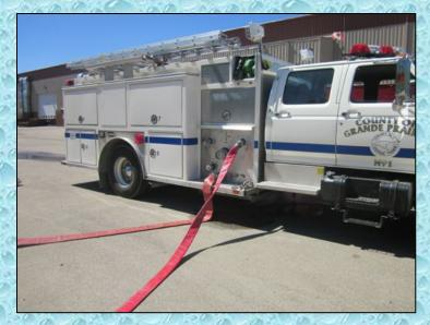
Engine 1402 served as the first-arriving engine with a crew of four people. The timer was started when the engine came to a stop at the dump site location. The crew went to work stretching a Blitzfire line and getting set up to draft from a dump tank.
