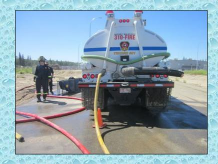
Engine 11 (750 gpm) was used at this hydrant and tenders were loaded using a single, 65mm hose line. Engine 11 was supplied by two, 65mm hose lines from the fire hydrant. This site loaded tenders much quicker.
