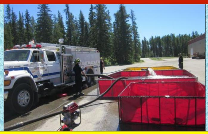
This photo taken around the 24-minute mark shows the dump tank arrangement. The engine used two suction lines (4-1/2" and a 3") to support the operation.
