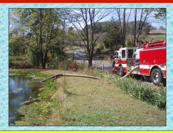
The crew from Engine 4-1 had this site set up fairly quickly. A ladder was used to try to keep the barrel strainer out of the muck.
