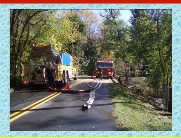
The crews set up a 5" line and two, 3" fill lines. They were set up in front of the engine to keep a driveway behind them clear.
