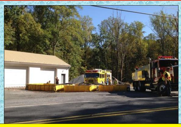
The 1,200 gpm flow was maintained for almost the rest of the drill. With five minutes left in the drill, the dump site ran out of water. It turns out that all of the tankers had ended up at one fill site – and a traffic jam had ensued. Since the drill was almost over anyway, it was decided to call it a day.
