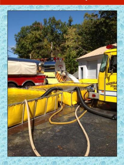
At 1200 gpm, RE23 lost its draft due to the main tank running empty. This was rectified quickly by an incoming tanker, but the crew struggled to re-establish the draft. It turned out that the auxiliary intake used to intake water from the nurse tanker – was left open. The crew figured this out but struggled to get air out of the sleeve going over the side. These problems were worked out and were a great learning experience for the new pump operator learning his craft.
