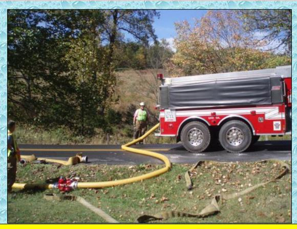
The site was able to fill at about 1,000 gpm. We're not sure the tankers got completely filled since they were sitting on a hill. The fill site crew did have to clean off the strainer occasionally due to vegetation in the pond.
