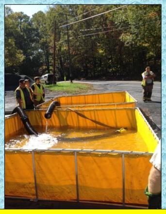
Two dump tanks in operation. The jet siphon has just been turned off. Note that the crew has positioned the low level strainer away from the jet siphon and in the lowest corner of the dump tank.
