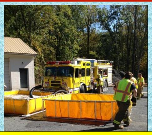
RE23 elected to draft using two suction inlets; two hard sleeves were used from the driver's side intake with the assistance of a 6" suction elbow, and one hard sleeve was used from the front intake. Both intakes had suction control valves which came in handy later.
