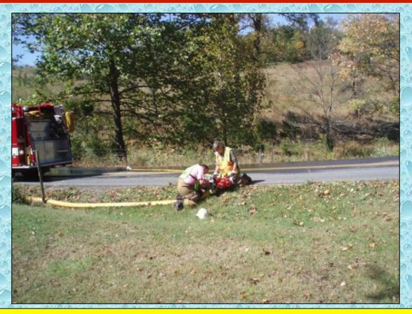
The crew set up a 5" line to a reversed 5" water thief to allow the crews to control the flow and drain the line to the tanker quickly.
