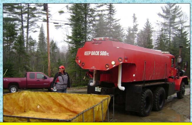
The diamond set-up of the dump tank makes it easier for the rear dumping tankers to position without blocking the entire road.
