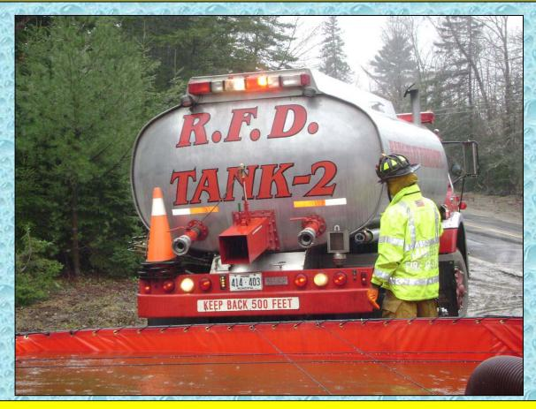
Meanwhile, on the other end of the dump site, Rangeley Tank 2 (2000-gal) backs into position to offload through its 8-inch rear dump.
