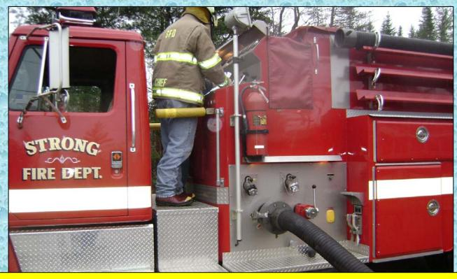
Strong Engine 3 just can't seem to get a prime. The crew works to troubleshoot – but without success. The tank is empty and there is an air leak in the suction hose connection.
