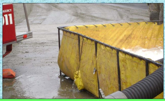
While not a big issue here, this dump tank should have been stowed with its drain tied up tighter on the inside of the tank.
