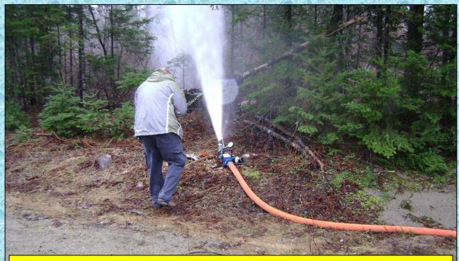
At the 13:59 minute mark, water flow is re-established to the Blitzfire and is sustained for the remainder of the 2hour test.
