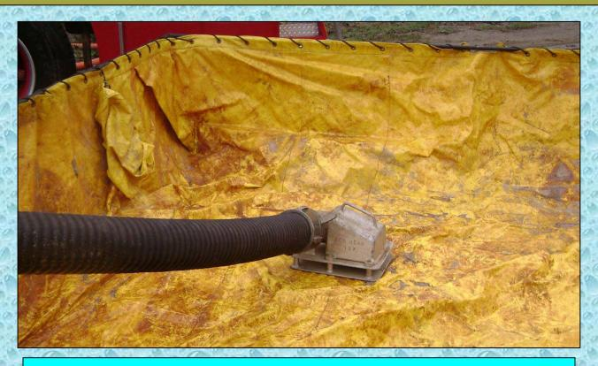
The first dump tank is ready to receive water. The use of this low level strainer will allow maximum use of the water in the tank.
