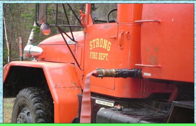
Adaptors become an issue as do threaded connections at a fill site. The connection shown above could be sped up by using 2-1/2-inch Storz adaptors.
