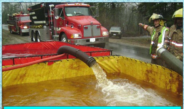
Eustis Tanker 5, the last tanker on the first Tanker Task Force arrives and gets into position to offload. Note the excellent stream of water coming from the jet siphon.
