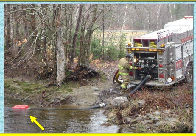
Note the floating strainer being used. There was concern over sucking up stream bottom silt – so the floating strainer was used.
