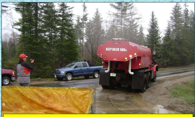
In order to better handle the rear-dumping only tankers, the 2500-gallon dump tank is relocated to the northern end of the dump site and set-up in a diamond shape.
