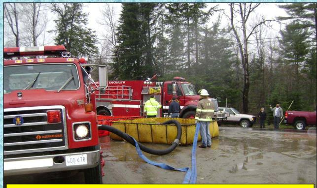
Still having drafting issues with Strong Engine 3, Phillips Engine 4 is directed to pump directly to Engine 3 in order to get water flowing again.
