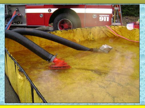
Phillips Engine 4 takes suction (red strainer) from the original dump tank and pumps to Strong Engine 3 which in turn supports the Blitzfire. The crews did a great job of overcoming the drafting problem with Engine 3.
