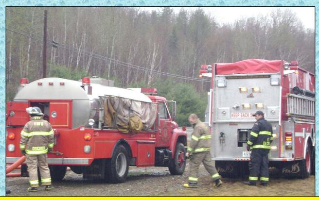
While two tankers can be connected to a fill site at the same time, the best practice is to only fill one at a time. That way all pumping resources are focused on one tanker.
