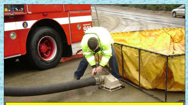
The crew works to prepare Engine 3 for drafting out of the tank. Here, a crew member connects a low-level strainer to the suction hose in preparation for placing the hose in the dump tank.
