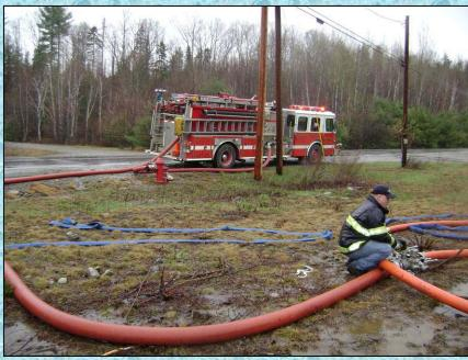
Fill Site #1 operated from a fire hydrant that had a good water supply. The goal in operating a fill site is to be able fill at a rate of 1000 gpm or better. Putting a pumper on the hydrant allows for maximum use of the available water. The 1500 gpm pumper used in this drill helped to guarantee a reliable flow to the LDH manifold.
