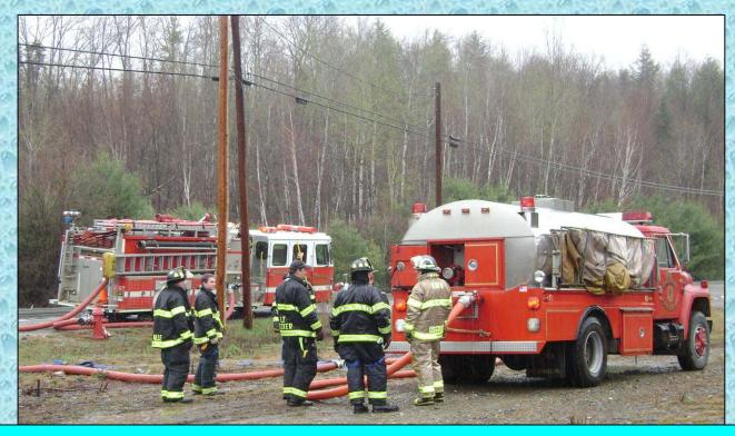
Fill site staffing is very important. At a minimum, someone is needed to run the pumper, the LDH manifold, and make and break fill line connections.
