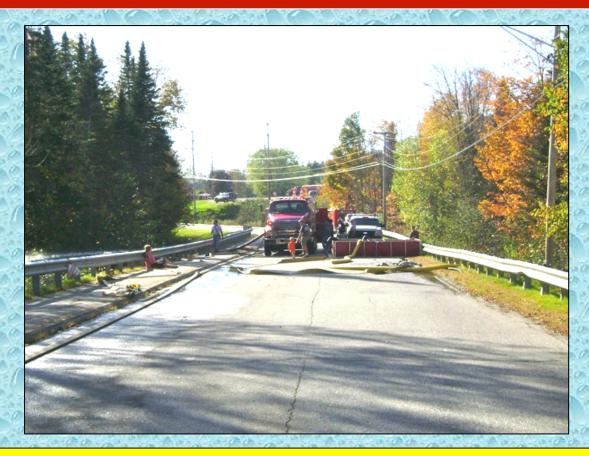
Temple Engine 3 (1,250 gpm) moves into position as the supply pumper and begins setting up for drafting operations out of the dump tank.
