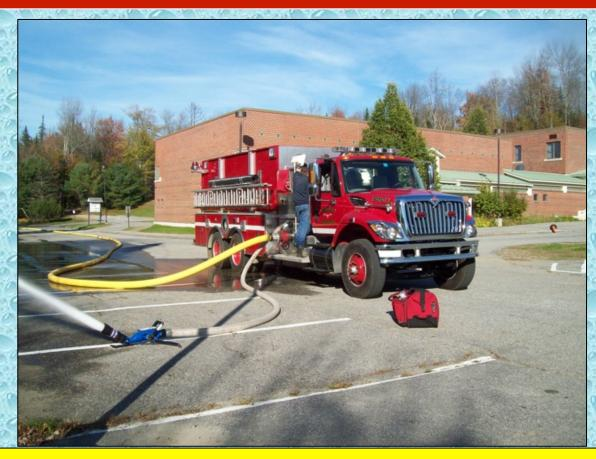
After having laid 600 feet of 5-inch LDH, Strong Engine 1 (1,250 gpm) became the attack pumper and flowed a TFT Blitzfire device.
