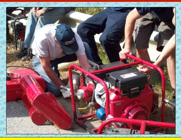
To make the relay operation a bit more challenging, portable pumps were used to draft from a brook and supply water to a dump tank from which a 1,250 gpm pumper then drafted and supplied the relay operation.
