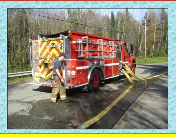
After laying out 1,000 feet of 4-inch LDH, Jay Engine 2 becomes the second relay pumper.
