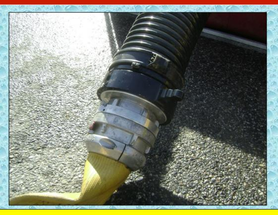
Of course, in order to use the hard suction hose, the correct adaptors are needed. An important safety point, when using hard suction as shown above, the opposite end of the hose MUST be left "open" so that the suction hose does not become pressurized.
