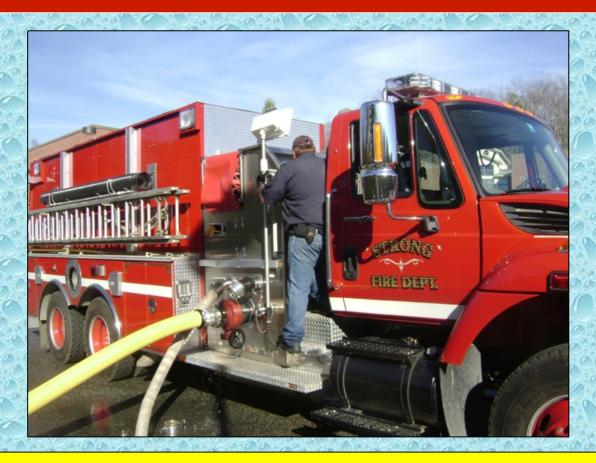
The supply line was taken directly into the officer's side suction inlet and water was discharged via 50 feet of 3-inch hose to the Blitzfire.
