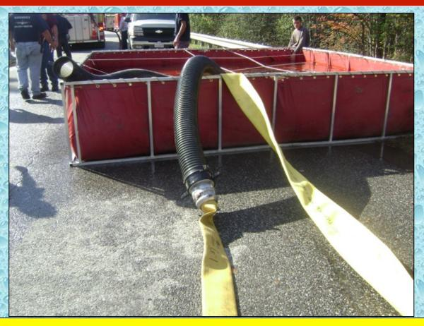
The 5-inch LDH dumped directly into a 3,000-gallon dump tank. One of the lines fed a 10-ft section of 6-inch hard suction and the other line fed an LDH manifold. The use of the hard suction hose prevents kinking of the line.
