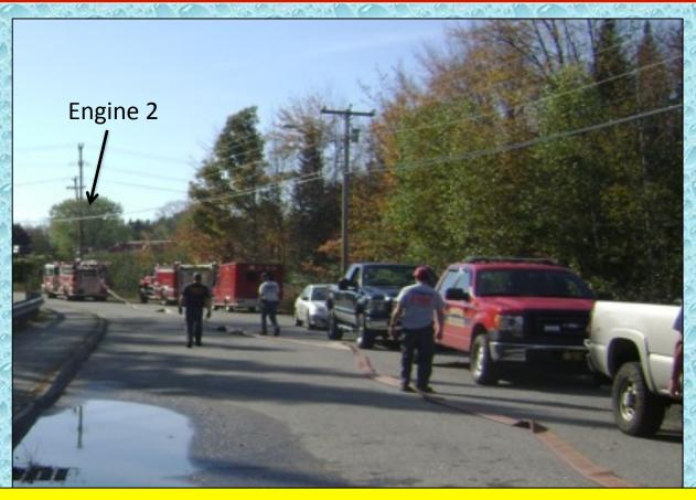
With the water supply established, Farmington Engine 2 (1,500 gpm) lays out 700 feet of 5-inch hose and takes a position as the first relay pumper.
