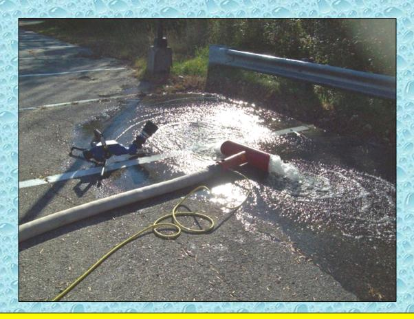
In order to accurately measure flow, the Blitzfire was changed out with a Hose Monster flow diffuser equipped with a fixed pitot tube.
