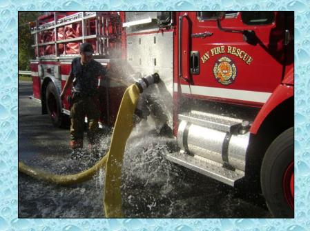
Engine 2 took in the supply via the piston intake valve with intentions of discharging via the high-flow discharge. The problem that arose was that Engine 2's piston intake relief valve was set at 70 psi (brand new valve) and the only way to make an adjustment was to remove the entire valve from the suction intake.
