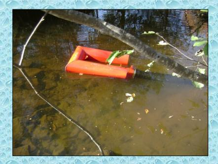
Another key to success with portable pumps is to use 3" or 4" suction hose in lieu of 2-1/2" suction hose and, use a good quality strainer. The second pump used in the drill was the 400 gpm one shown above. It took water from the same brook as the 500 gpm pump.
