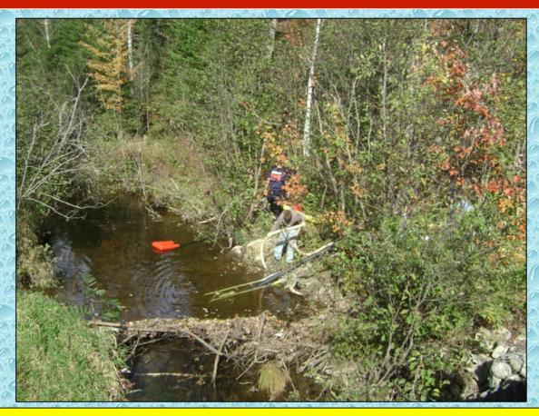
Brooks and streams can be deceiving in terms of their looks and the flow available. This brook was able to easily support the 650 gpm flow used for this drill.
