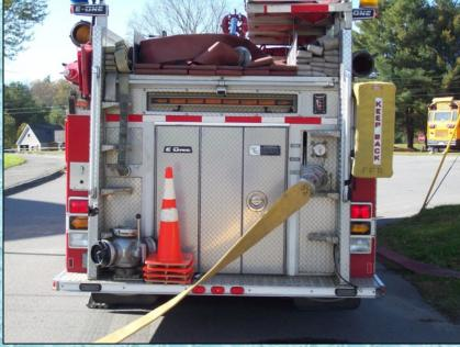
The supply line was broken and connected to the officer's side piston intake valve. The next pumper, Jay Engine 1, began its lay of hose. That hose was initially connected to the Farmington pumper's rear discharge.
