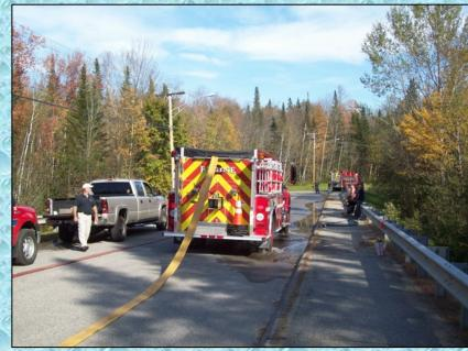
Jay Engine 1 (1,250 gpm) begins its lay of 1,000 feet of 4-inch LDH from Farmington Engine 2.
