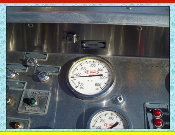
The relay was set up to test several discharge settings: 75 psi, 100 psi, 125 psi, and 150 psi. The 150 psi discharging setting on the supply and relay pumpers yielded a flow of 631 gpm – which was the highest flow achieved.
