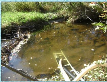
One key to success with a portable pump is to minimize the lift. This 500 gpm pump is placed as close to the water source as possible. In addition, 5-inch hose is used to improve the discharge flow.
