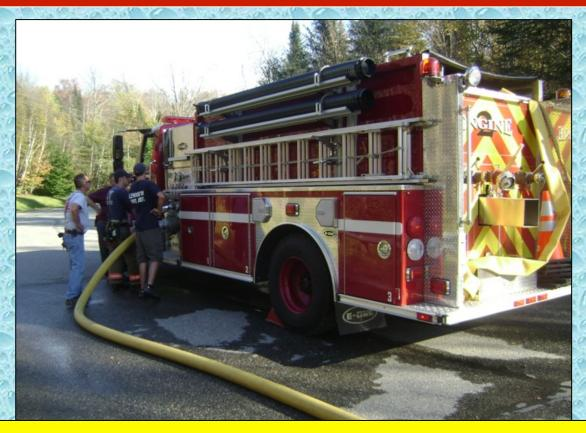
The decision was made to switch intakes and take the supply line directly into the driver's side suction inlet – however, there was NO external relief valve so intake relief was dependent on the Farmington pumper operator controlling his discharge pressure.
