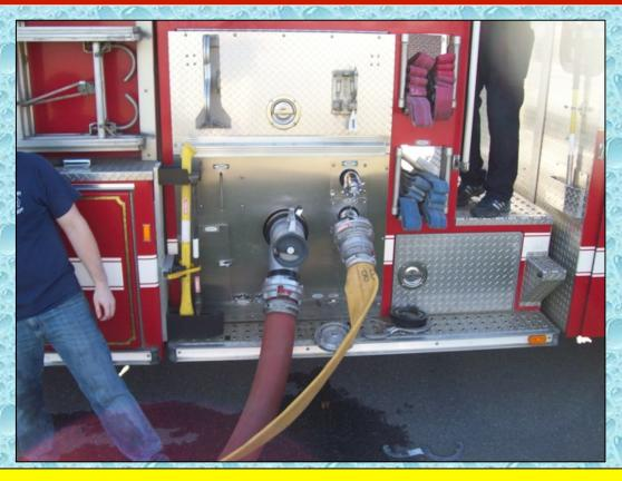
After some discussion, the hose feeding the Jay pumper was moved from the rear discharge of the Farmington engine to the officer's side discharge. This move provided a greater flow ability – the rear discharge would have been more restrictive.
