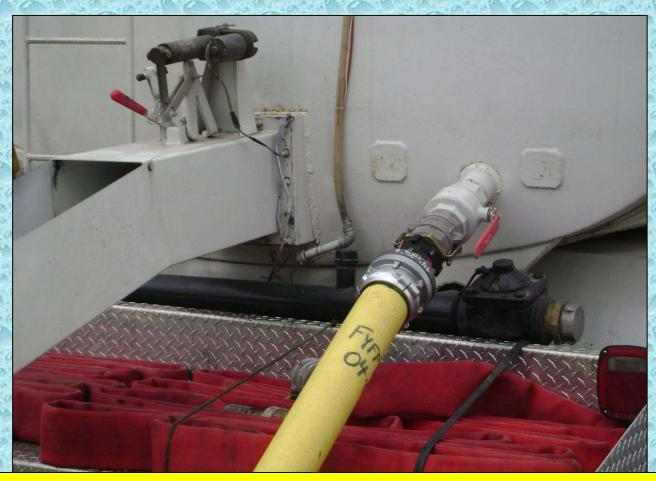
Connections and hose size make a big difference in fill times.
