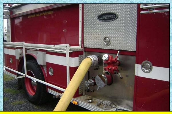
Sylvania Engine 2 supplies the 5-inch line feeding the attack engine. Note that the pumper does not have a high-flow discharge so the 5-inch is connected to a 2-1/2-inch discharge which limited its flow to about 1,000 gpm on this pumper.
