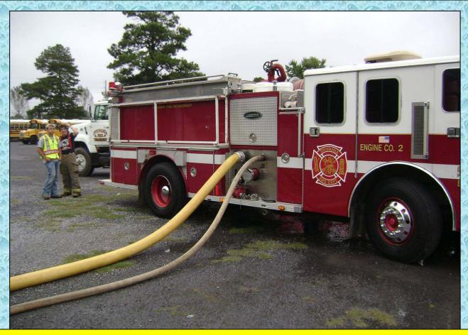
In order to increase flow, a 2-1/2-inch line was added into the supply – not ideal, but it added about 300 more gpm capability.
