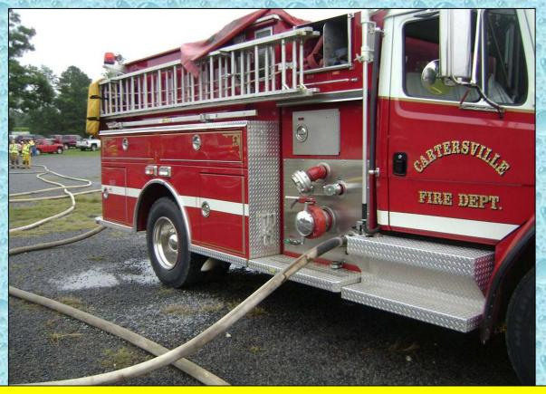
Because the 5-inch line is connected to a single, 2-1/2-inch discharge on the Sylvania engine, a 2-1/2-inch supply line is added in anticipation of higher flow needs.
