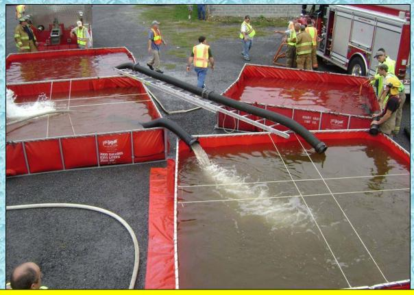
With four, large dump tanks now in operation, there is ample space for water storage thus allowing a larger fire flow. When full, this site can hold 11,500-gallons of water.
