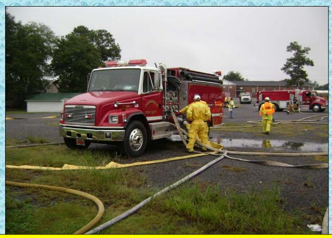
With a nurse tanker operation still in effect, a 5-inch supply line is laid from Sylvania Engine 2 (dump site engine) to Cartersville Engine 1.
