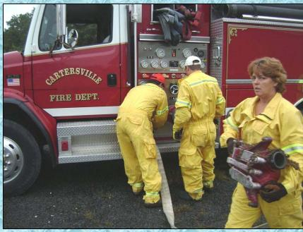
With everything set, the drill begins. The stopwatch was started when Cartersville Engine 1 came to a stop and the driver engaged the parking brake. The engine laid dual, 2-1/2-inch supply lines about 300-ft in length.
