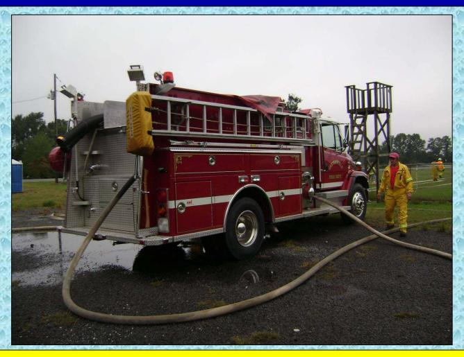
Engine 1 is now being supplied through two, 2-1/2-inch supply lines.
