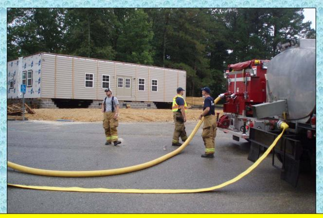
The fill site crew at the lake does a good job of filling one tanker at a time – thus committing maximum pump capacity to one tanker at a time. Note that both tankers are hooked up, but only one is being filled.
