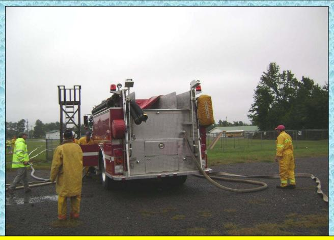
With 250 gpm now flowing, the attack engine prepares to receive water from the Adamsburg tanker.
