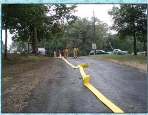
Hammondville Engine 1 (1,250 gpm) sets up to draft on the boat ramp at the lake. A 5-inch line is used to support tanker fill operations.
