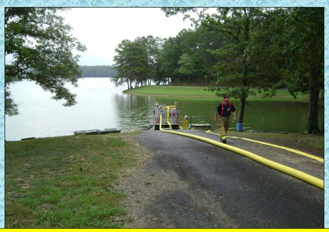
Another good use of LDH to improve pumping capacity to the fill appliance. This 5-inch hose maximizes the pumper's capability.
