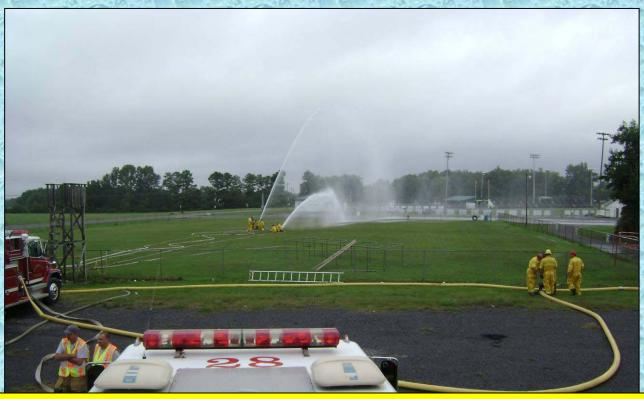
At the 40:00 minute mark, the flow was increased to 750 gpm by placing the 2-1/2-inch attack line back into service. Meanwhile, a second portable monitor is being set up on the right in anticipation of moving to a 1,000 gpm flow.
