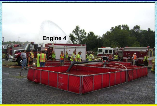
With the flow increased, Fyffe Engine 4 is taken out of the shuttle to run the jet siphons thus allowing the draft engine to commit its pumping capacity to supplying the attack engine.
