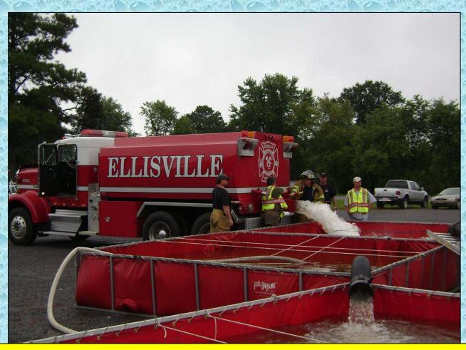
Ellisville Tanker 39 dumps it water and supports the 500 gpm flow.
