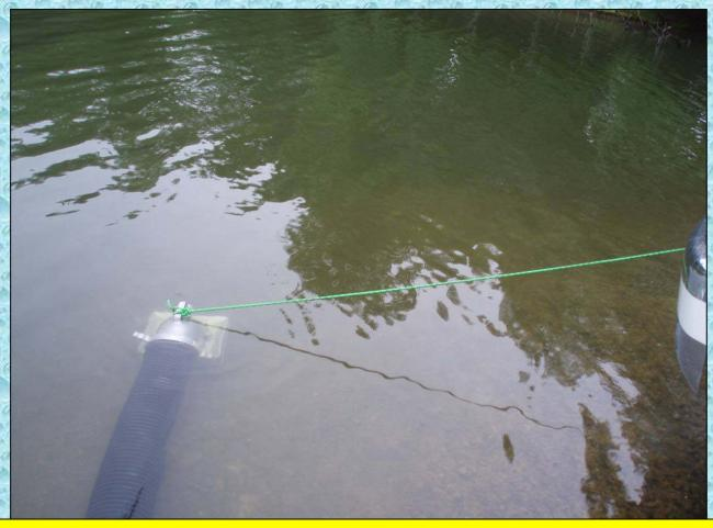
A low level strainer is used on the boat ramp to access the lake's water.
