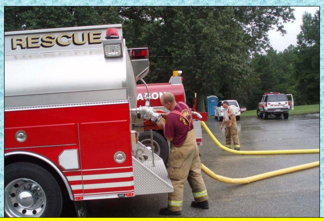
Quick connect adaptors such as Storz couplings and CamLok fittings can really reduce loading time. Much improvement occurred in this area from the 2008 drill.
