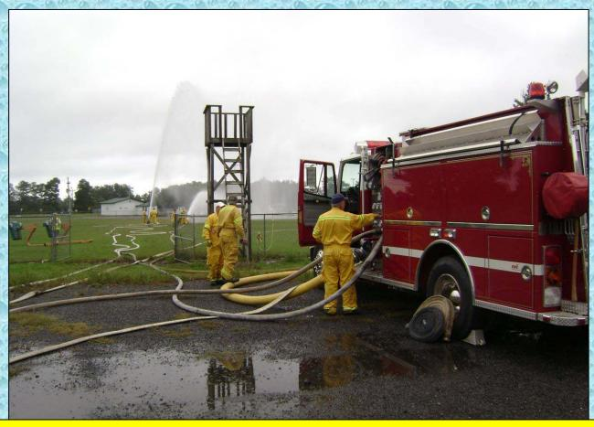
The attack engine works effortlessly to supply the 750 gpm flow - all because of the 5-inch supply line.
