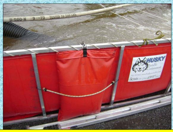
This dump tank manufacturer uses a snap hook to keep the tank drain held up high - thus eliminating the need to tie it up. Good idea and it seemed to work well!
