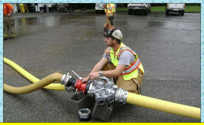
A couple of appliances were needed to make this work, but the crews are using LDH to fill tankers which means better efficiency. With the manifold reversed, a 2-1/2-inch outlet can be used as a drain when breaking a fill connection on a tanker.
