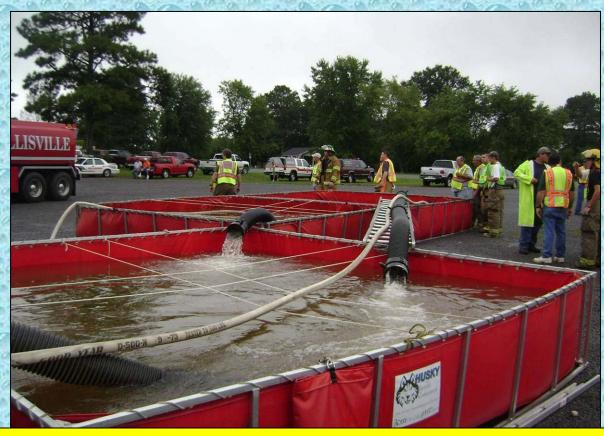
Two jet siphons are used to transfer water to the primary dump tank.
