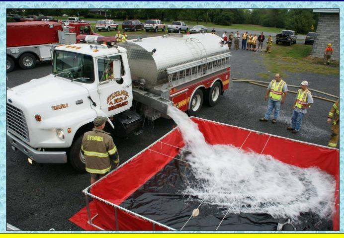
While the Adamsburg tanker continues to pump off to the attack engine, Sylvania Tanker 1 starts dumping its 3,500 gallons into the dump tank.
