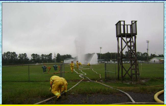
At the 15:00 minute mark the flow is increased to 500 gpm using the portable monitor. Flow was measured by a handheld pitot gauge. The photo here shows both lines in operation – it was taken during the transition to the portable monitor (the stream on the left.)
