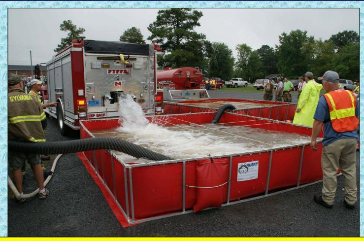
Fyffe Engine 4 is shown dumping its 1,800 gallons of water into the primary drafting tank.
