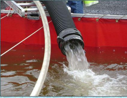
When pumping jet siphons, the goal is to have the water output look like the photo on the left. The photo on the right shows a jet siphon that needs more pressure. There should be a solid stream of water being discharged from the suction hose.
