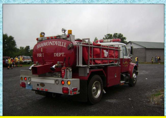
Hammondville Tanker 1 backs into position to dump its 1,500 gallons.
