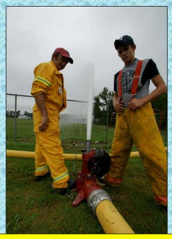
A portable monitor from a Fyffe engine is used to flow the 1,000 gpm. Note the 5-inch inlet on the device.
