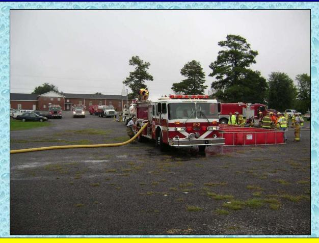
Sylvania Engine 2 (1,250 gpm) goes to work as the draft engine at the dump site.
