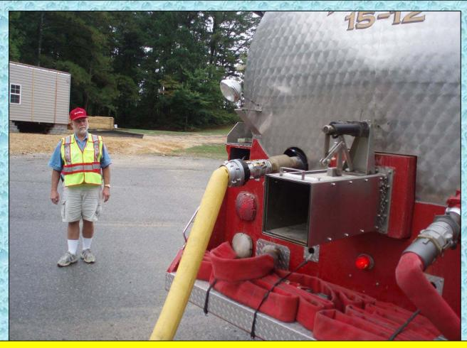
Sylvania's Tanker 1 is shown being filled using 4-inch LDH connected to one of the tanker's direct fill lines.
