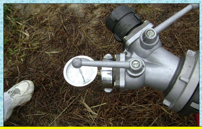
Because the hydrant was on the very outskirts of the water system, flow was less than 1,000 gpm. When filling tankers, the residual pressure dropped to about 15 psi. It wasn't great, but it worked.
