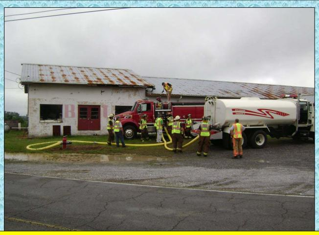
Powell Engine 1 (1,250 gpm) operates this fill site using a hydrant.
