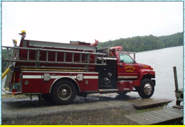
Hammondville gets in a good position to maximize drafting. By getting the pump as close to the water as possible, lift is minimized thus increasing pumping capacity.
