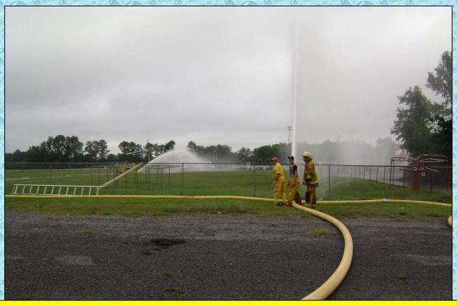
At the 1-hr, 45-minute mark, the flow is moved to 1,250 gpm using the portable monitor on the right and the 2-1/2-inch hand line on the left. The flow is sustained for the remaining 15-minutes of the drill.
