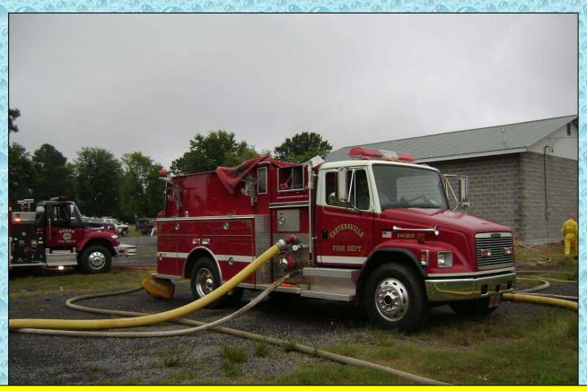
At the 60-minute mark, Engine 1 pumps the 5-inch line shown above which feeds a portable monitor. The supply to the other portable monitor and hand line is shutdown.
