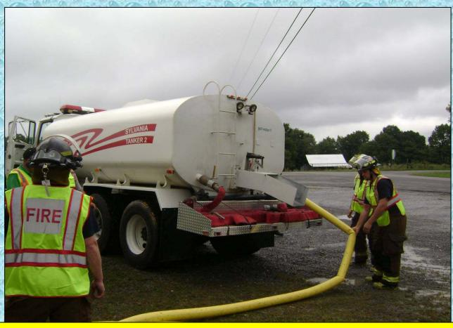
Like the lake fill site, crews use LDH to fill tankers at this fill site as well. Sylvania Tanker 2 is shown here being filled.
