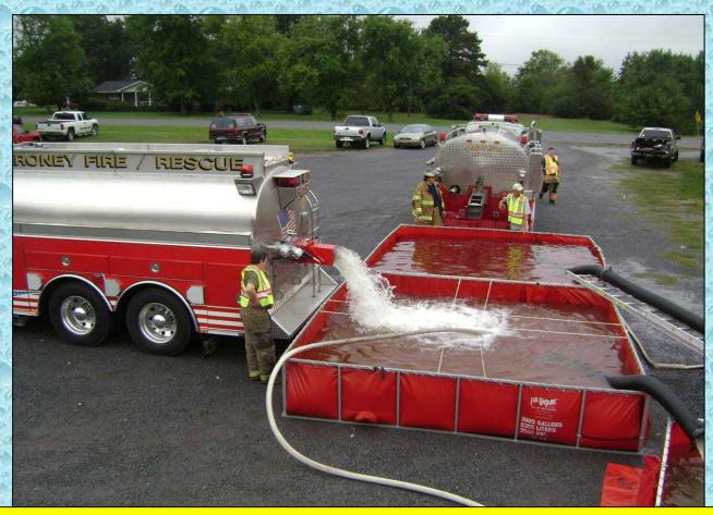
With the flow now at 750 gpm, more tankers are needed to support the operation.
