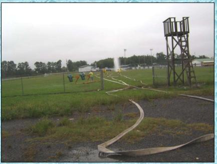
At 6:30 minutes, the water flow is interrupted but is restored 15 seconds later when Adamsburg Tanker 1 begins supplying the attack engine.
