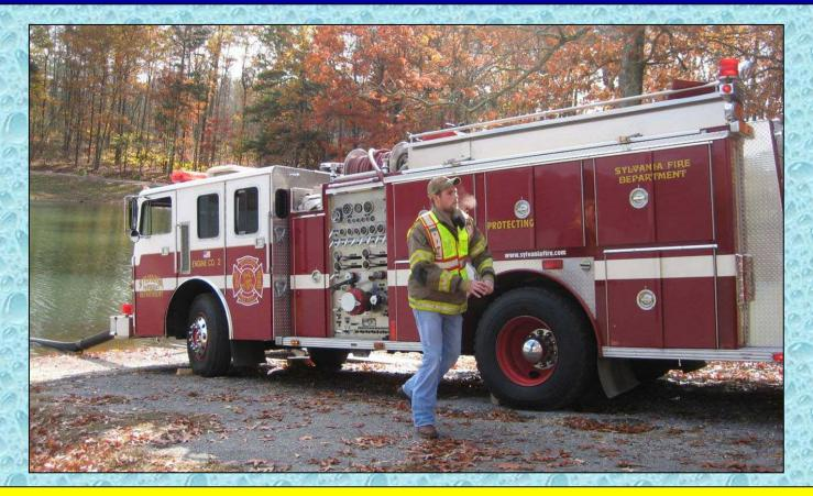
Engine 2 elects to use their front suction for drafting which ends up reducing their ability to meet the 1000 gpm filling requirement.
