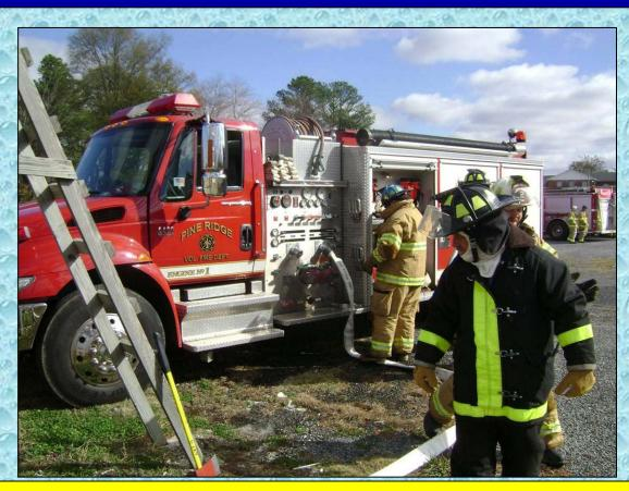
Engine 1's crew deploys a portable monitor fed by 100-ft of 2-1/2-inch hose which will allow a 250 gpm flow to be started at the 5-minute mark.
