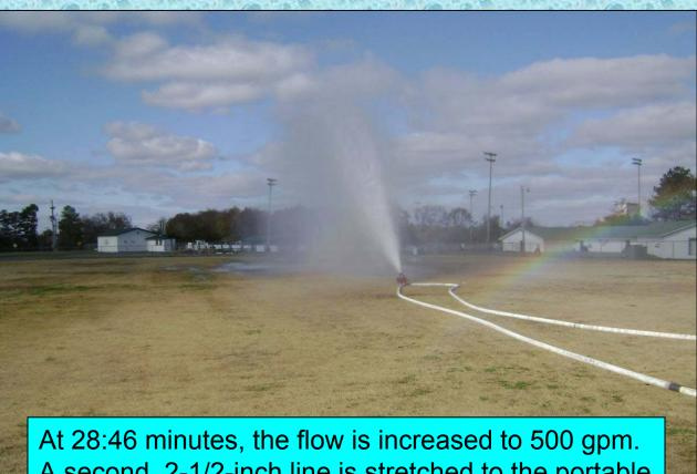
A second, 2-1/2-inch line is stretched to the portable monitor to accomplish the flow.
