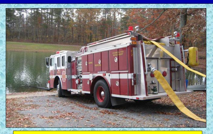
Sylvania Engine 2 sets up on the boat ramp and prepares to draft. The 5-inch hose line (lower) is set to supply a LDH appliance for filling tankers.
