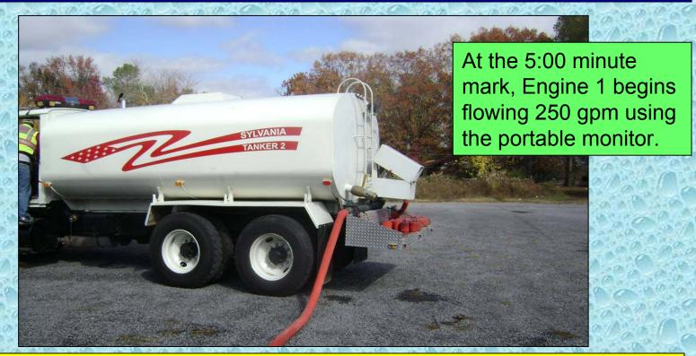
With nurse tanker operations underway, a problem is encountered; this tanker can barely keep up with the flow rate of the Pine Ridge engine. The cause of the problem is that the tanker is a "used" water tanker for street watering and its small off-loading pump cannot support the drill's 250 gpm flow.
