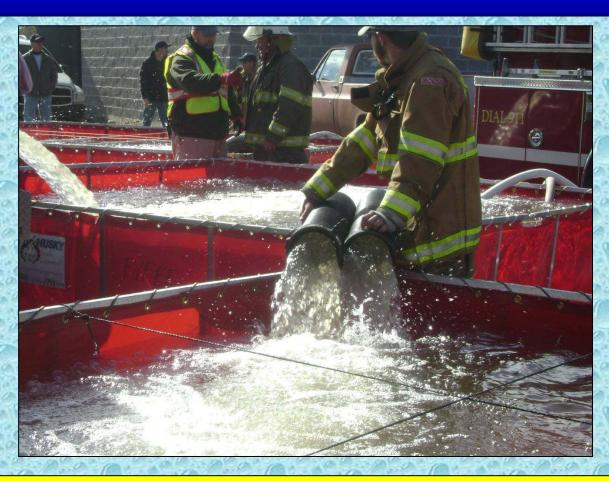
Dual jet siphons are now needed to support the flow into the primary drafting tank.
