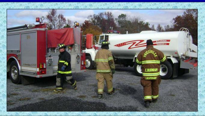
A decision is made to use a nurse tanker while dump tanks are set-up. Sylvania Tanker 2, a 3,750 gal tanker arrives and prepares to supply Pine Ridge Engine 1. LT Eric Burnham (right) assumes the role of Water Supply Group Supervisor.
