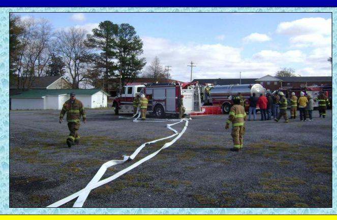
Additional crews arrive and dual, 3-inch lines are laid in order to supply Pine Ridge Engine 1 - thus switching from a nurse tanker operation to a dump site operation.
