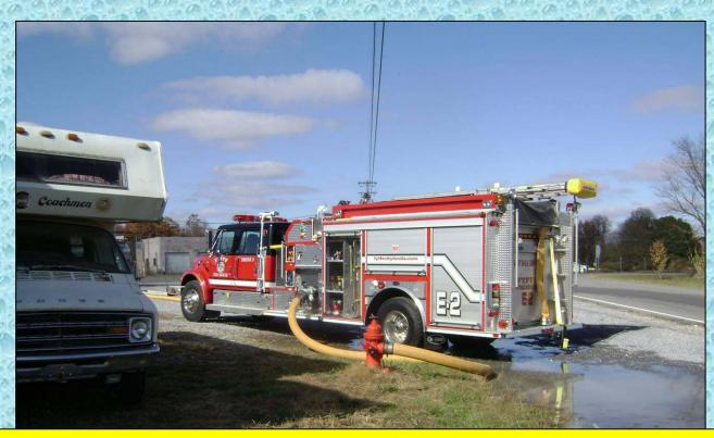
Fyffe Engine 2 (1,250 gpm) uses a municipal fire hydrant to provide water supply at its fill site. Tankers using this fill site had to make a 5-mile round trip from the dump site.
