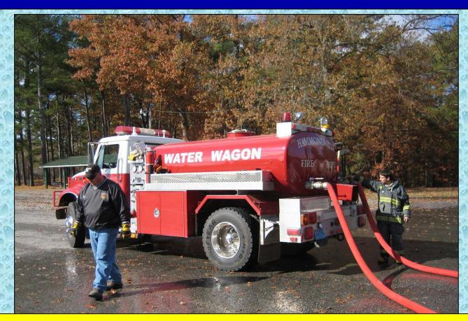
This smaller tanker has a large dump that dumps quick – filling could be faster if a larger, direct fill existed or LDH was used.
