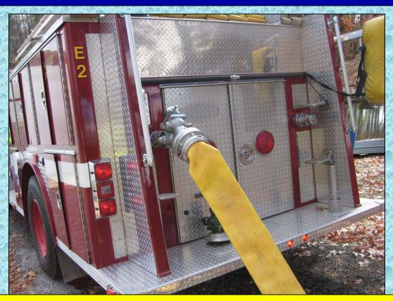
Another flow problem was encountered – Engine 2 elected to connect the 5inch hose to a 2-1/2-inch rear-discharge. While this certainly works, the problem here is that the flow was limited to about 600 gpm - when 1000 gpm was needed.
