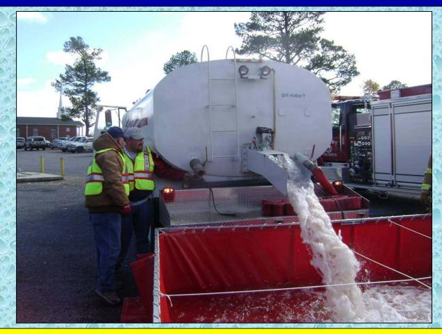
Sylvania Tanker 2 switches from the nurse mode to the dump and run mode of operation now that the dump site is operational.
