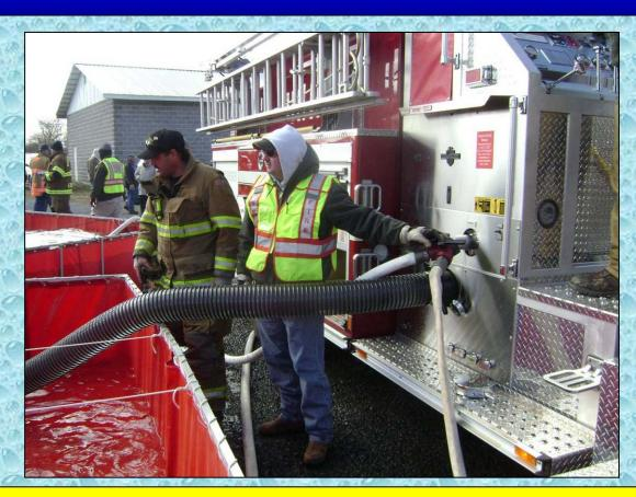
This fire fighter is controlling two jet siphons using the gated-wye attached to the pumper discharge. One of the jet siphons is used to help the Kilpatrick engine maintain its draft.
