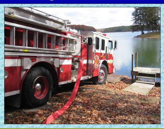
To fix the problem, two, 3-inch lines were pumped (each from a different 2-1/2-inch discharge) into the 5-inch hose. This helped but did not overcome the front suction drafting problem.
