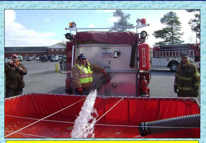
Dogtown Engine 1 uses its Jet Dump to quickly off-load 1,000 gallons of water into the initial dump tank.
