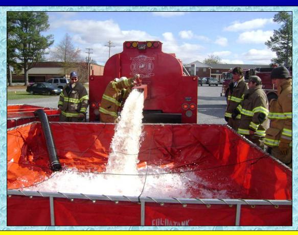
Dogtown Tanker 1 (1,400 gallon) arrives and off-loads into a second dump tank (3,000 gallon) as the dump site begins to expand.
