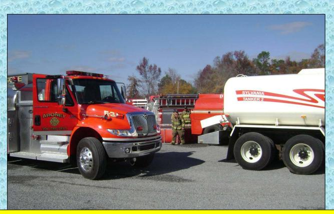
Multiple tankers are now dumping and running and keeping the shuttle operational.
