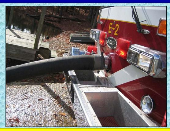
It is important to remember that a front suction on a rig with a midship mounted fire pump is NOT rated for the capacity of the pump and use of the front suction generally reduces the pump's capacity at draft.
