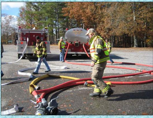
Almost all of the tankers attending this drill had small, direct fill lines which hampered their ability to load. The fill site crews used "cam lock" adaptors and LDH where possible – but large, direct fills would have made a big difference.
