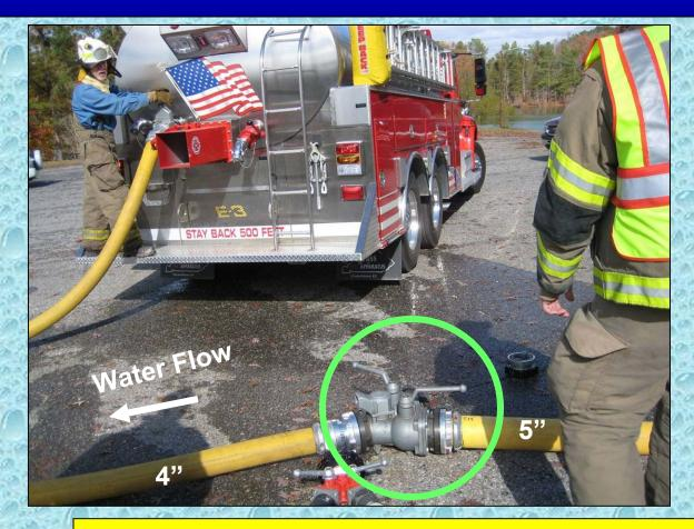
Note the wye is "reversed". This allows one outlet to serve as a large drain.
