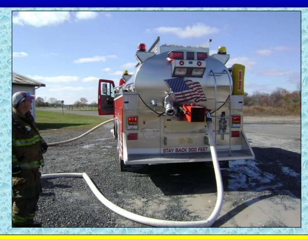
A common issue at both fill sites was the need for adaptors. Hose fittings that were used included 2-1/2-inch NST, 2-1/2-inch cam locks, 3-inch cam locks, 4-inch Storz, and 5-inch Storz.
