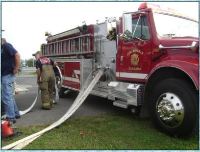
Collinsville Engine 1 (1,250 gpm) prepares to take over the dump site. Without a high flow discharge, Engine 1 must use multiple, smaller lines to feed the 5-inch hose supplying the attack engine – Crossville Engine 2.
