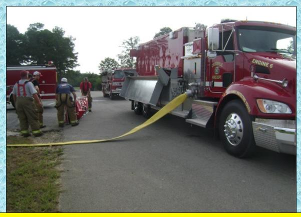
Engine 6 is connected for nurse tanker operations while additional crews begin to build a dump site.
