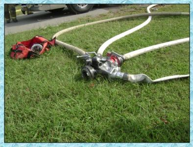
An LDH manifold is set up to combine the smaller lines into a single, 5-inch supply line. But...the 5-inch line has to be disconnected from the nurse tanker first.
