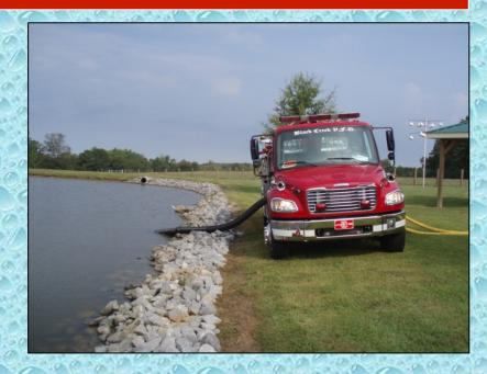
Water access was great and drafting was very easy. Engine 150 was able to fill tankers at an average rate of 1,200 gpm.
