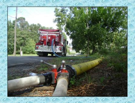
Again – no high-flow discharge, so dual, 3-inch lies feed a control valve and tankers are filled with a 4-inch line.
