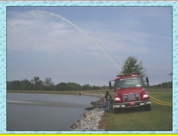
The pump operator used the pre-piped deck gun as his circulation line. The gun was shutdown while filling tankers and re-opened when done.
