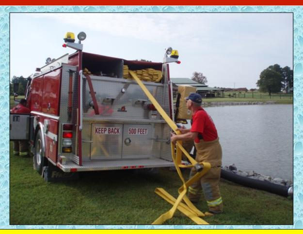
One issue with the Black Creek pumper is that it does not carry LDH, so multiple, 2-1/2-inch lines were needed to support the 1,000 gpm filling rate goal.
