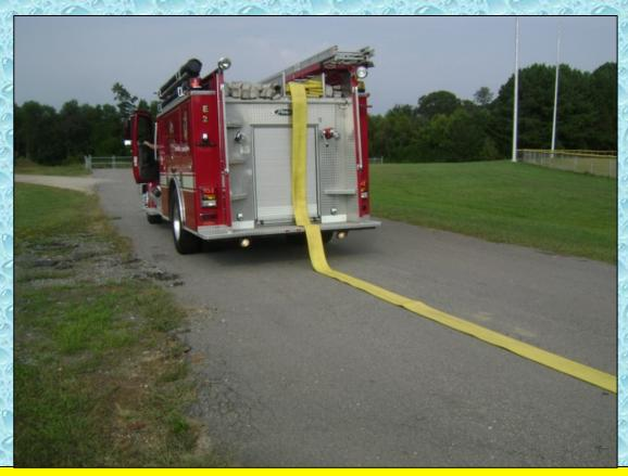
Crossville Engine 2 arrives on the scene and times starts. The crew laid out 300-ft of 5-inch supply line in preparation for being supplied by the next arriving unit.
