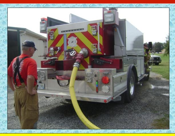
Engine 150 pumped dual, 150-ft, 2-1/2-inch lines siamesed into a 4-inch line for tanker fill operations.
