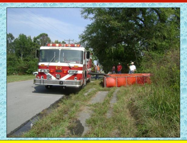
This fill site involved the use of a hydrant that could not support a 1,000 gpm flow without some help.
