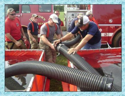
With flow expected to hit the 1,000 gpm mark, the use of another engine makes sense since the the dump site pumper has a 1,250 gpm pump. While jet siphons are much needed – they also consume pump capacity – so planning ahead is important.
