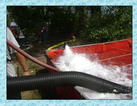
The hydrant fills the dump tank and the engine then drafts water and fills tankers at a rate faster than what the hydrant could do by itself in a direct hookup.
