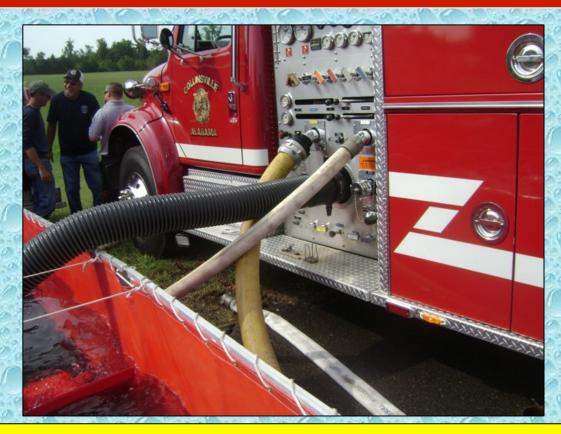
To help improve the flow from the dump site engine, one of the 2-1/2-inch lines is replaced with a 4-inch line – this helps reduce the friction loss and increase the flow.
