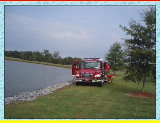
Black Creek Engine 150 (1,250 gpm) takes position to draft and support a tanker fill station.
