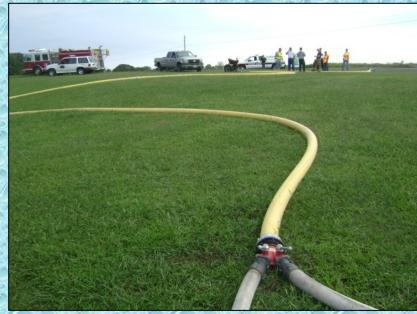
Hammondville Engine 1 (1,250 gpm) drafts and supplies 5-inch LDH for tanker fill operations. Once again, without a high-flow discharge, the pumper pumped two smaller lines into a control valve which fed the 5-inch hose.
