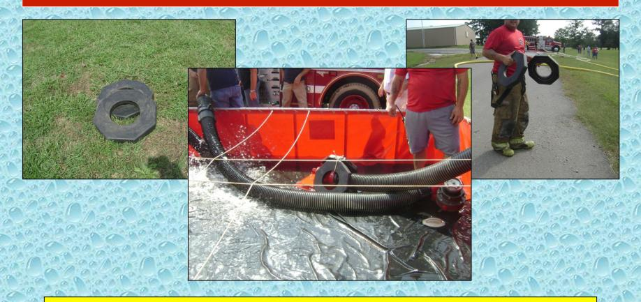
One issue that sometimes arises is low level strainers flipping over and causing the pump to lose its prime. The folks from Crossville use some traffic cone weights to keep the strainer in place – it works quite well.
