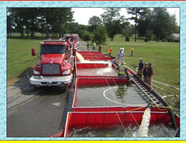
At the 48:00-minute mark the flow is moved to 750 gpm and around the 55:00-minute mark, the dump site operates five tanks.
