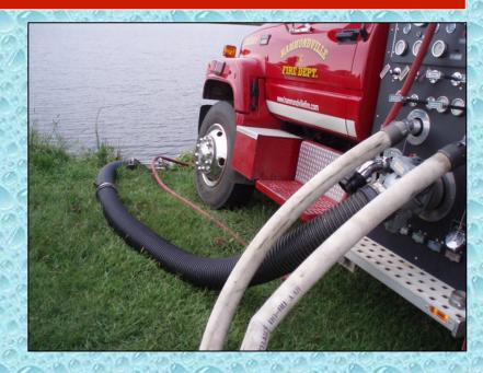
Engine 1 had good access to water at this site as well and used a low-level strainer for drafting.
