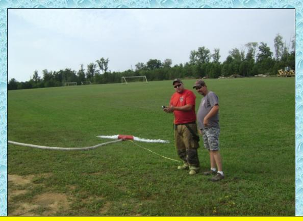
At the 5:00-minute mark, flow is started at 282 gpm using water from Engine 2. The flow is being measured using a Hose Monster flow diffuser equipped with a fixed pitot tube.
