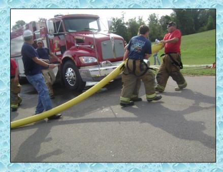
At the 18:09-minute mark, the crews begin to switch out the nurse tanker and transition to the dump site operation. The issue was no control valve on the line feeding the attack pumper. Had there been a manifold or siamese in the line, then this type of changeover would not have been necessary.
