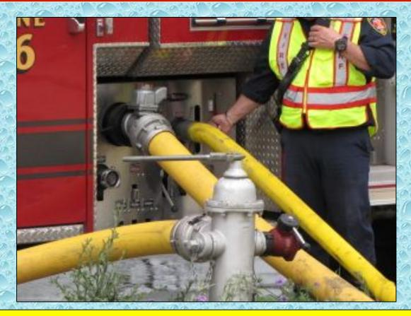
This fire hydrant provided ample water for the loading operation. The engine driver prepared the fire hydrant for additional flow (ball valve on 2-1/2" outlet) but this was never needed.
