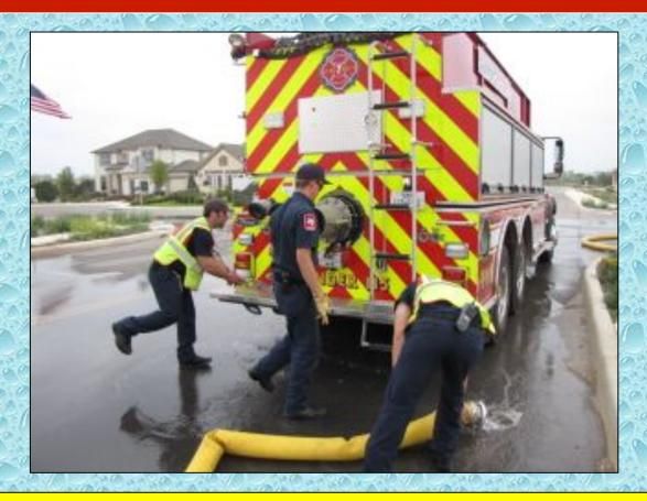
When possible, the tenders were filled using 5-inch hose. For those tenders that had smaller direct fills, 3-inch fill lines were used.
