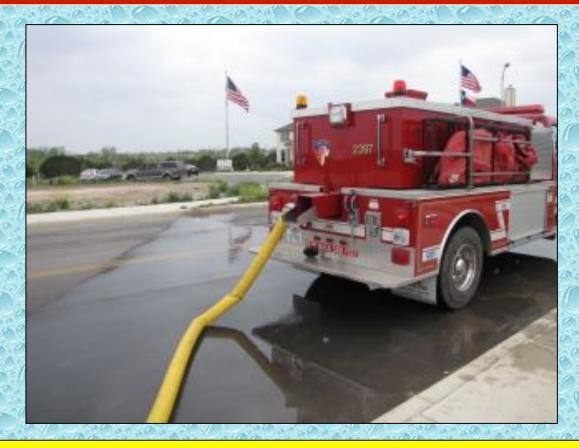
A 2,000 gallon tender being filled in just under 3-minutes – this includes hook up time!
