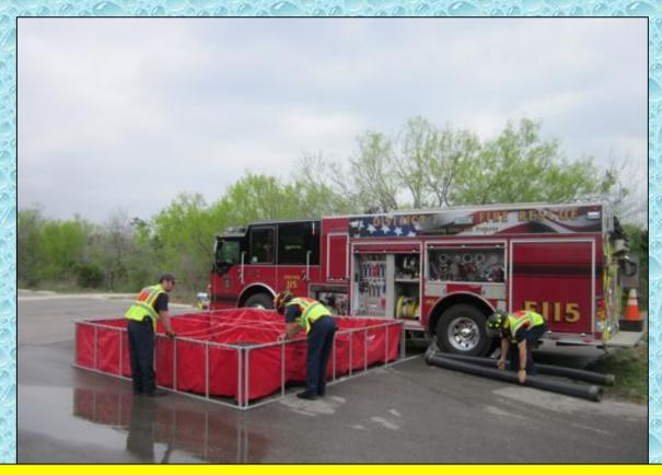
Engine 115's crew used Tender 115's dump tank and wasted no time setting up for dump site operations. Meanwhile, water flow was underway at 250 gpm to the Blitzfire from Tender 115.
