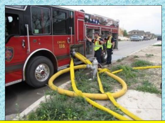
District 7's Engine 116 (1,500 gpm) operated the lone fill site using a fire hydrant. In this area of Texas, there is very little dependable surface water – so fire hydrants are a critical resource. Using a pumper on a fire hydrant ensures a quick loading rate (1,000 gpm+).
