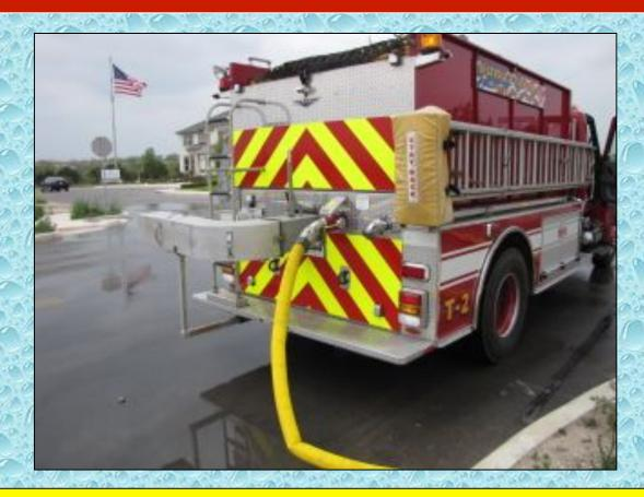
When used in short lengths, 3-inch hose can be effective in loading tankers - however, higher discharge pressures are needed at the fill site pumper.
