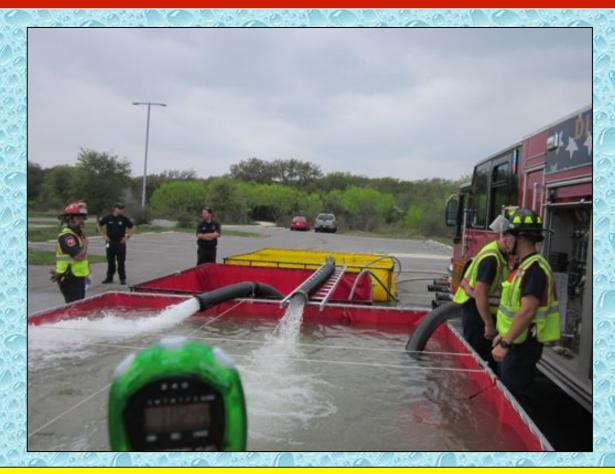
A three dump tank operation was now fully operational and supporting the 825 gpm flow.
