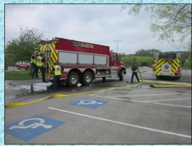
District 7's Engine 115 was the first unit to arrive on the scene. Six hundred feet of 5-inch supply line had already been laid out to two Blitzfire devices which simulated an attack pumper. The stopwatch was started when Engine 115's driver applied the air brakes. Tender 115 (3,000 gallons) arrived shortly thereafter and went to work setting up a "nurse tender" operation.
