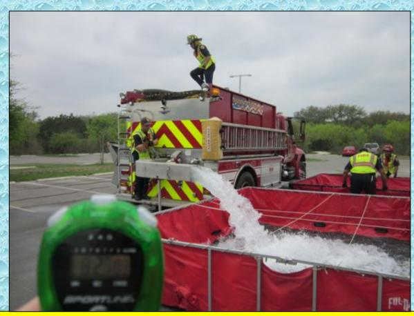
At around the 8:20 minute mark, the first load of water was dumped into a dump tank – and a second dump tank was deployed.
