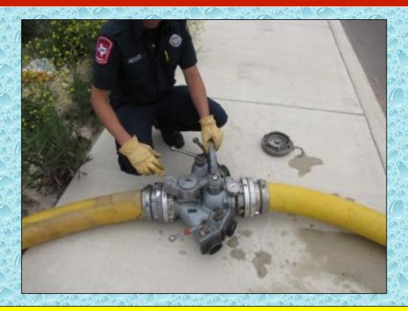
An LDH manifold was used as the loading valve and one member staffed the valve and controlled flow into the tenders. The valve was supplied by Engine 116 off of the fire hydrant.
