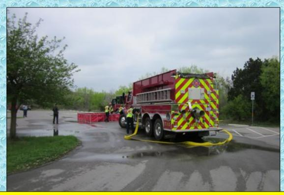
Tender 115 supplied a 3-inch hose line that fed one side of a 2-1/2" x 2-1/2" x 5" clappered siamese connected to the supply line feeding the simulated attack pumper. Once the operation switched to a dump site operation, Engine 115 took over and supplied dual 3-inch lines into the siamese.
