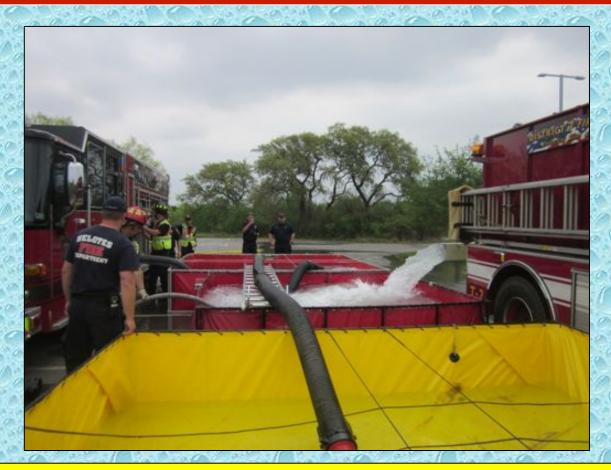
A third dump tank was dropped with expectations of increasing flow. The key was building a transfer device – which required some additional suction hose.
