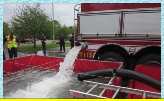
Engine 115 had now switched to drafting out of the dump tank, so Tender 115 broke free from nursing and dumped the remainder of its water into the dump tank before heading to be reloaded. Water flow was moved to 448 gpm at the 15-minute mark.
