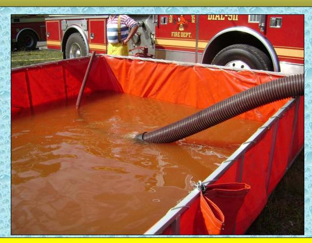
Engine 61 begins to transfer water between the two dump tanks using a jet siphon and a 6-inch hard sleeve.
