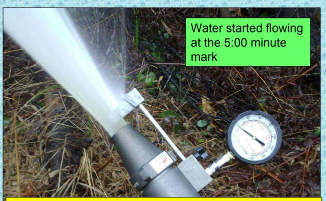
A 1-1/2-inch tip was installed. Using 20 psi as the desired gauge pressure – a flow of 300 gpm is achieved.
