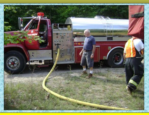
With water being used faster than tankers can supply it, Tanker 35 operates in the "nurse-mode" and supports Engine 61 when the dump tank gets low.
