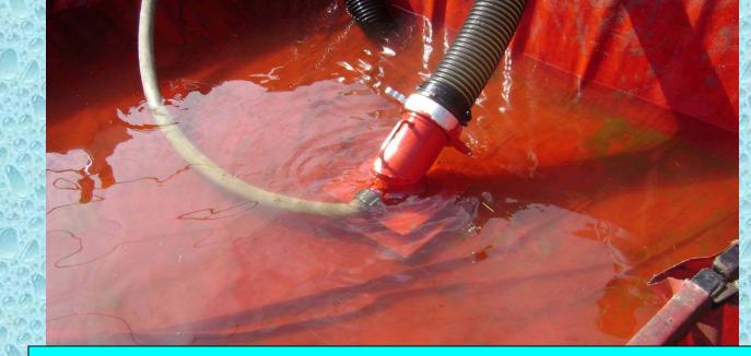
The first dump tank is made operational. The use of this low level strainer will allow maximum use of the water in the tank.
