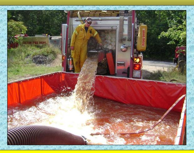
Colton Engine 81 offloads its 1,000 gallons into a second dump tank (2,000 gallon) as the crews try to build out the dump site.
