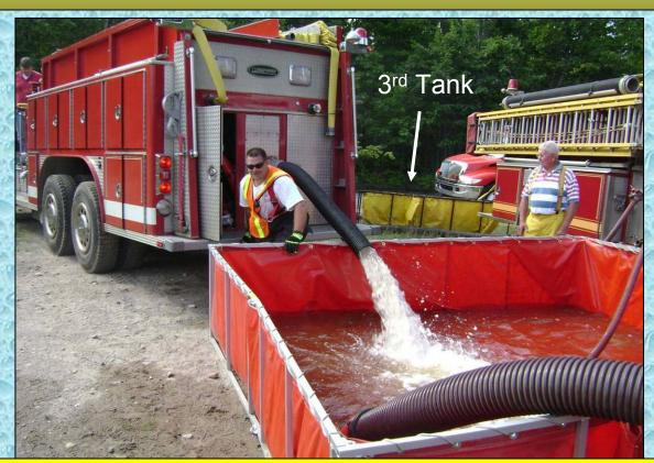
As Engine Tanker 44 dumps another load of water, a 3<sup>rd</sup> dump tank is placed out on the main road in an attempt to have some of the tankers dump off of their side instead of their rear. However, the flow did not allow a break in the action so that the tank could be made operational.
