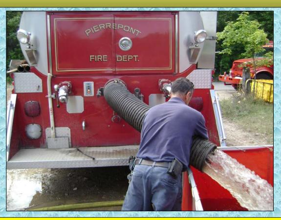
With the dump site operational, Tanker 35 switches from the nurse-mode to the "dump and run" mode. Here, a flexible tube with a cam lock fitting is used to direct the offload stream.
