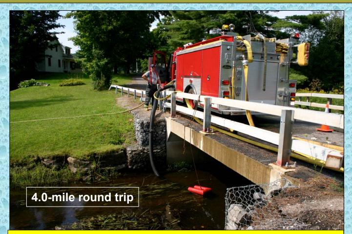
Pierrepont Engine 65 drafts from a stream through 20-ft of suction hose and fills tankers.
