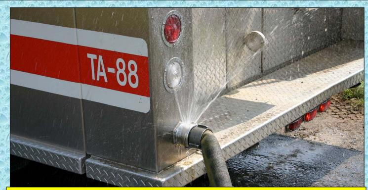
All of the tankers attending this drill had small, direct fill lines which hampered their ability to load. If the fill piping cannot be made larger (4—inch or bigger), then at least 4-inch LDH should be used to fill the rig.
