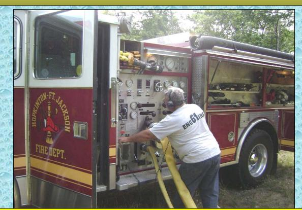
Engine 61's operator is kept pretty busy shifting between taking in water from Tanker 35 and drafting from the dump tanks in order to supply the attack pumper. At 23:00 minutes, the dump tanks are empty and no tankers are in place to dump.
