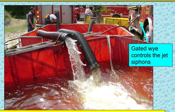
Engine 61 puts a second jet siphon into service which really helped sustain the flow.
