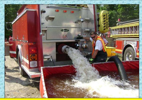
Pierrepont Engine 47 quickly off-loads its 1,500 gallons through its 7-inch rear dump.
