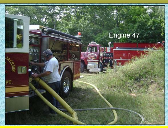
Engine 61 transitions from being supplied by Engine 47 to drafting from the dump tank. The "experienced" operator of this rig made this transition run smoothly.
