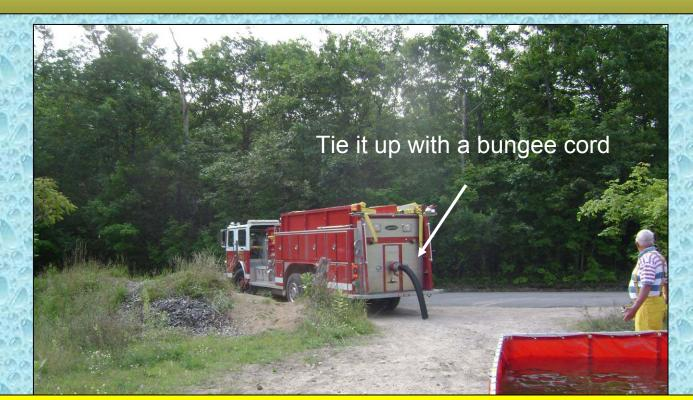
Engine Tanker 44 leaves the dump site with its dump tube dragging. This is one of the problems with rear dump "only" rigs. This cam lock tube could have been tied up so that it is ready to go when the rig returns to dump.
