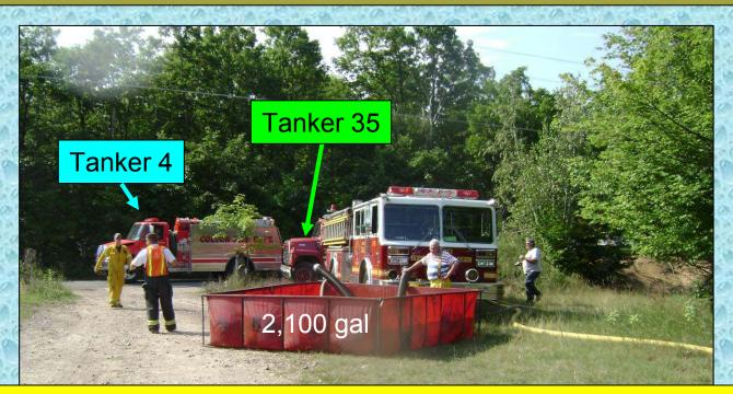
The fellow in the orange vest is Chief Kevin LaBrake (Pierrepont FD) who assumed the Water Supply ICS position. Engine 61 is now being supplied by Pierrepont Tanker 35 and is in-turn supplying Engine 10 through the LDH supply line. A draft has not yet been attained.
