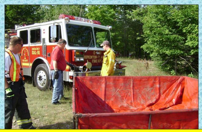
The crew works here to prepare Engine 61 for drafting out of the dump tank - they elect to use the engine's front suction.
