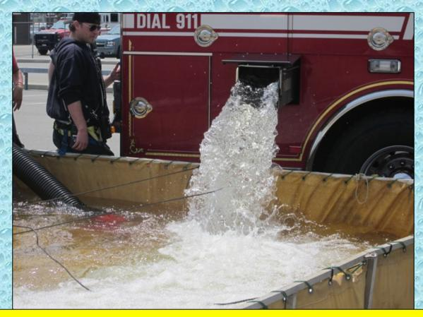
Additional tankers continue to arrive and off-load their water. The nurse tanker operation is discontinued and that tanker moves into the water hauling rotation.
