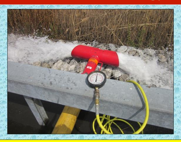
At the 57:00-minute mark, flow was moved to 1,000 gpm. A Hose Monster flow diffuser with built-in pitot was used to measure the flow.
