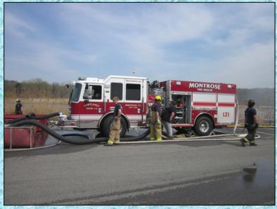
In order to improve operation. A second suction line was set-up using the Montrose pumper's driver side suction inlet. The addition of this suction line aided in maintaining the 1,250 gpm flow.
