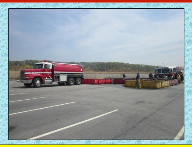
Garrison Tanker 15-41 dumps its 3,500 gallons of water. It is important to note that there are no other tankers waiting to dump or dumping water.
