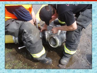
A 5-way LDH manifold was the first valve used at the loading station. The problem was that there was no easy way to drain the lines when the tankers were full. Had the manifold been turned the other way before the supply line was charged, the need to make changes later would not have occurred.
