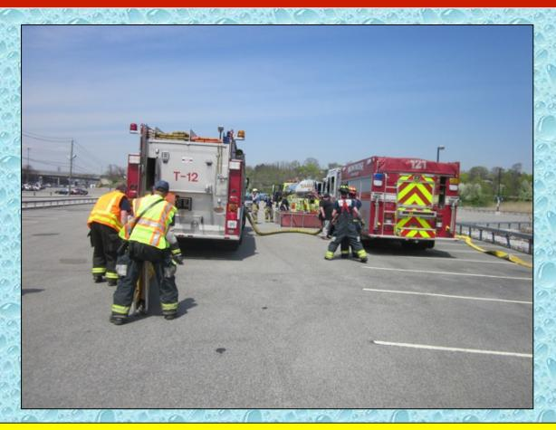
Montrose Engine 121 arrived and began setting up as the dump site pumper while Pocantico Hills Tanker 12 engaged in nurse tanker operations.
