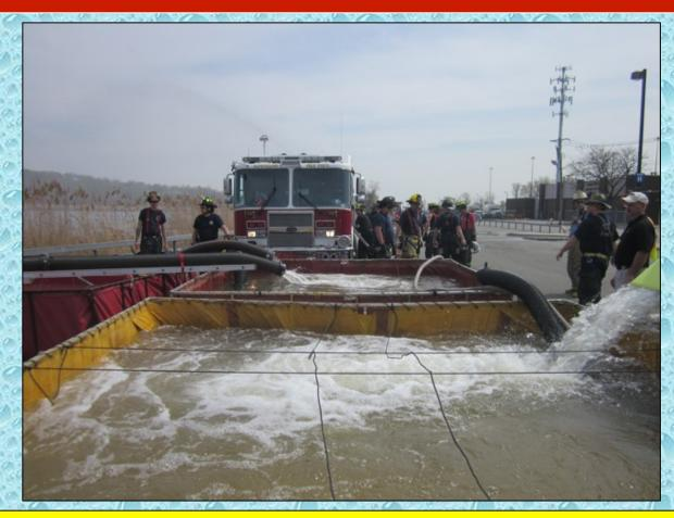
At the 63:00-minute mark, flow was moved to 1,250 gpm and the four dump tank operation was stabile.
