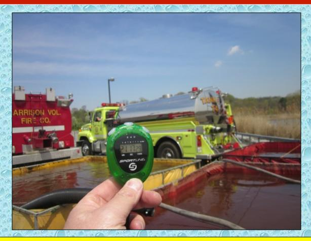
Flow was moved to 750 gpm at around the 15:00-minute mark. At the 21:00-minute mark, three dump tanks were in use.
