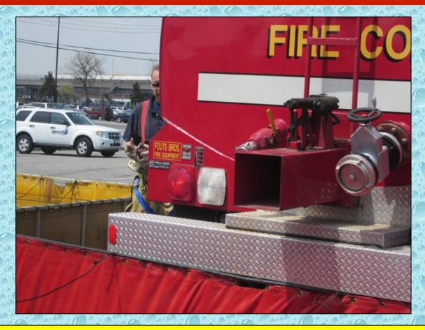
An interesting situation occurred when the bumper height on this tanker was greater than the height of the dump tank – which complicated backing actions a bit.
