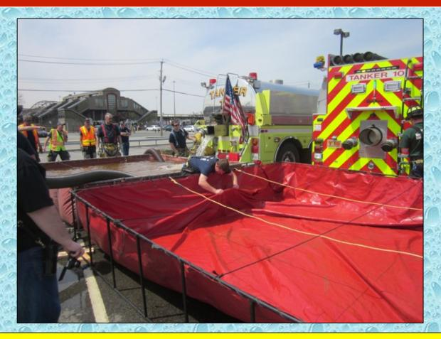
Additional tankers begin to arrive and the second dump tank (3,500 gallons) is set-up.
