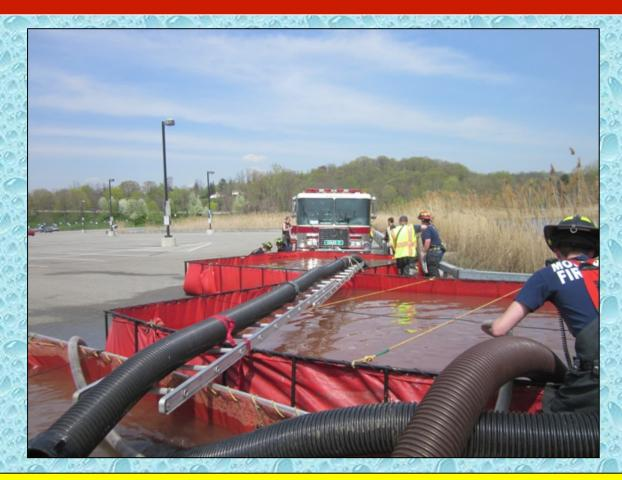
The Montrose pumper was having difficulty increasing flow and a second pumper (Croton Engine 118) was brought in to operate jet siphon devices.
