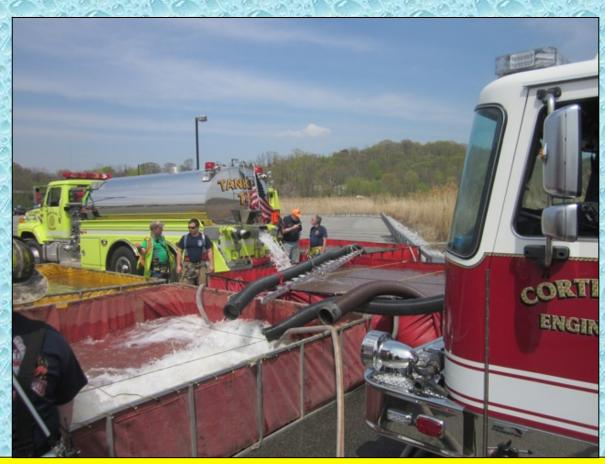
The dump tank arrangement was a bit unusual but was driven by the placement of a utility pole that limited the maneuvering of the larger tankers.
