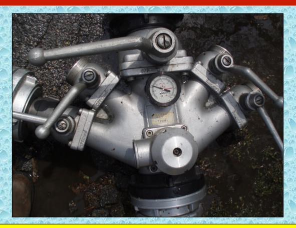
Tankers were filled at a rate of 1,000 gpm and the supply pumper maintained a pressure of 75 psi at the manifold.
