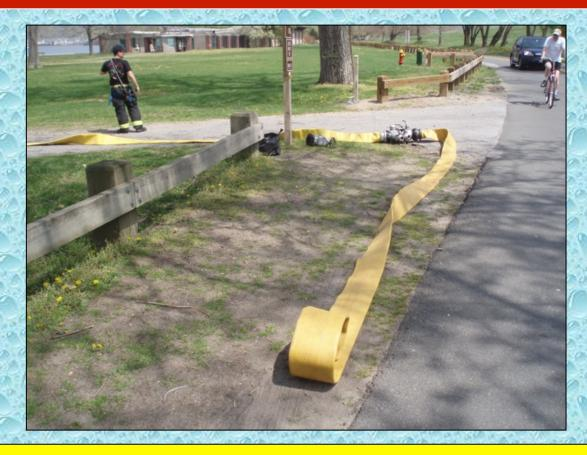
FDVA Engine 225 arrived at the fill site location and laid out 500-ft of 5-inch LDH from the gate back to the river access point.
