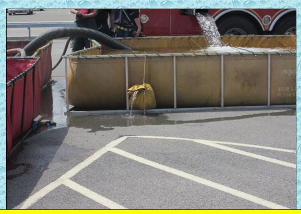
It is important to tie up dump tank drains. While this leak is not huge, it would help create a big mess in a more rural setting or during times of freezing temperatures. Best practice for older style tanks is to tie the drains up on the inside of the dump tank.
