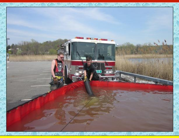
Engine 118 drafted out of the 4<sup>th</sup> dump tank and supplied water to run two jet siphon transfer devices.
