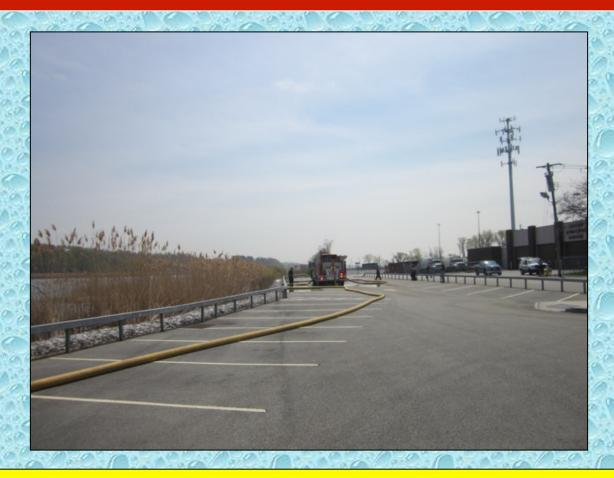
At the 4:45-minute mark, water flow was started at 630 gpm.
