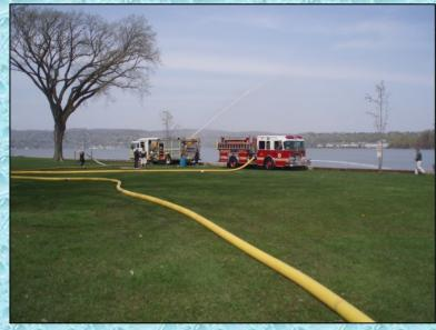
At around the 45-minute mark, Croton Engine 120 (2,000 gpm) was put into operation as a second fill site pumper. They laid their own 5-inch supply line and set-up a second loading station.
