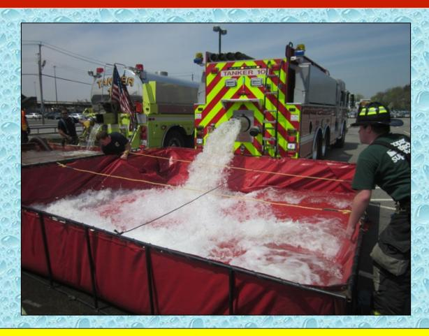
Croton Tanker 10 dumps its 3,000 gallons of water – a little bit premature since no transfer device is yet in place.
