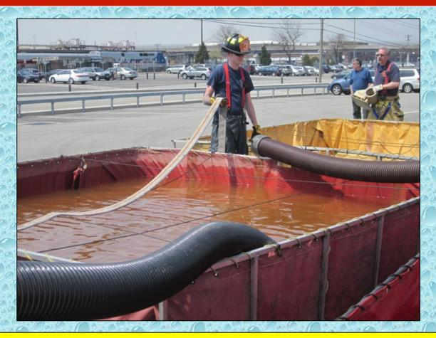
Crews work quickly to get water transfer devices set-up so that the dump site can move to a three-dump tank operation.
