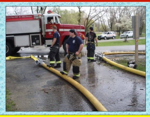
The use of LDH and LDH appliances and fittings makes for a very effective and efficient loading operation that helps meet that 1000 gpm minimum fill rate.
