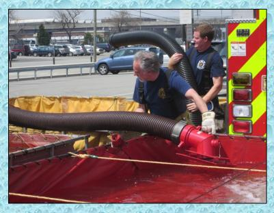
A third dump tank (3,000 gallons) is set-up as is a jet siphon to transfer water from the second dump tank into the primary dump tank.
