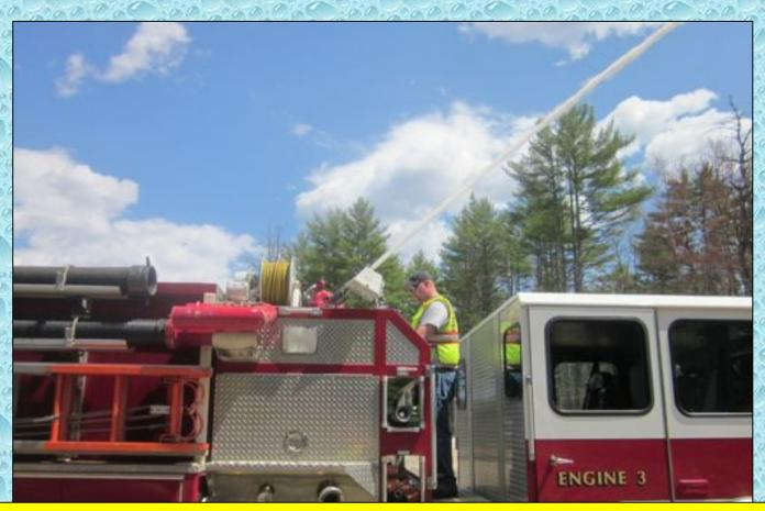
At the 5-minute mark, flow was started at 250 gpm using the attack engine's deck gun.
