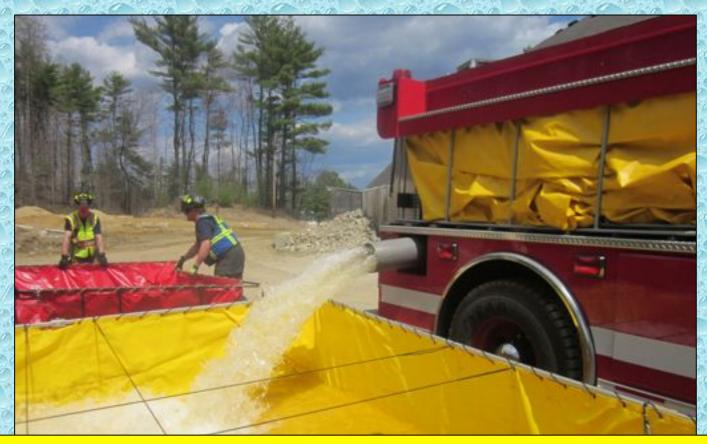
At the 15-minute mark, flow was moved to 523 gpm and operations were moved over to a dump tank operation. Barnstead's 3,000-gallon served as a nurse tanker during the early moments of the operation.
