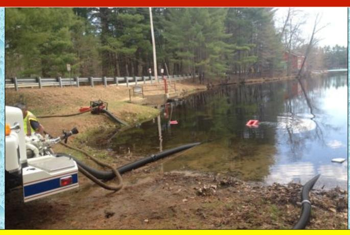
The access area to the lake provided ample room for the pumper to set up drafting operations. The addition of the portable pump increased the ability to load tankers by allowing the pumper to take in more volume.
