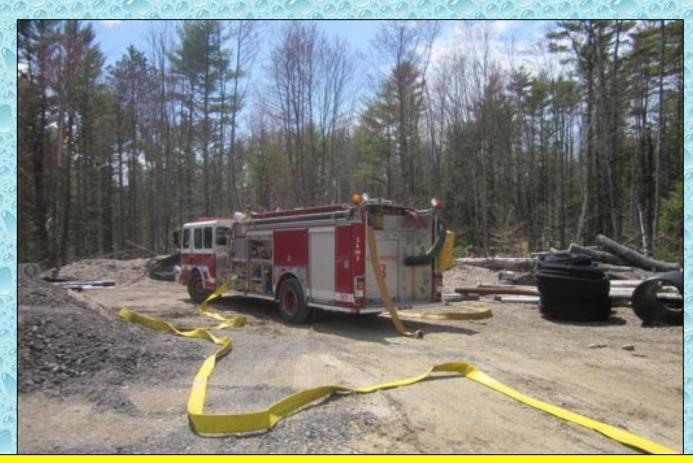
The attack engine worked to stretch a 4-inch line to a HoseMonster flow diffuser for accurate flow monitoring.
