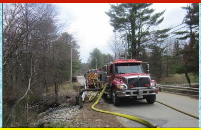
The large capacity pumper had little trouble obtaining a draft. Tankers were loaded at this fill site using 4-inch LDH.
