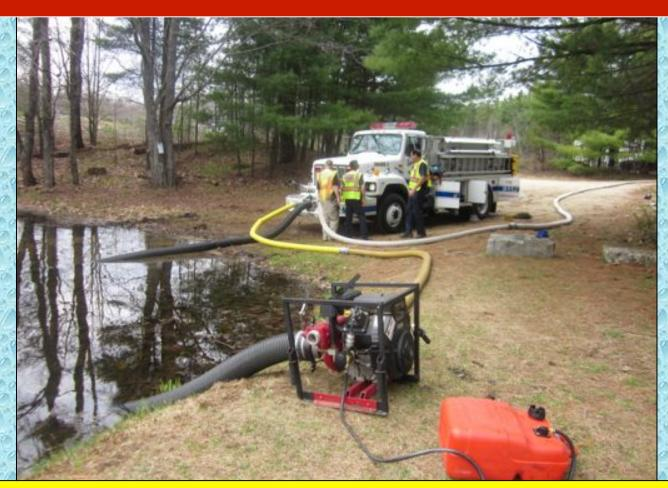
Pembroke 62-Engine-3's (1,250 gpm) crew used a 500 gpm portable fire pump to bolster their pumper's output capability at the pond fill site.
