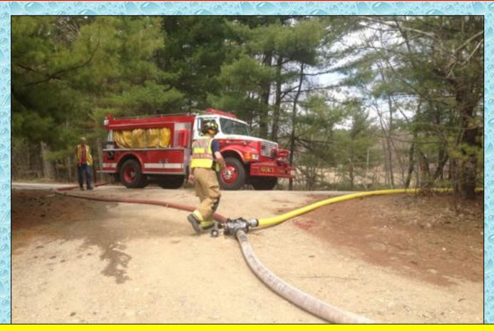
The Pembroke engine supplied a TFT manifold which was used to load the tankers as they arrived at the fill site. Tankers were loaded using 4-inch LDH.
