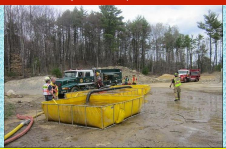
The dump site crew replaced the small red tank with a larger (yellow) tank and that change made a big difference in flow sustainability.
