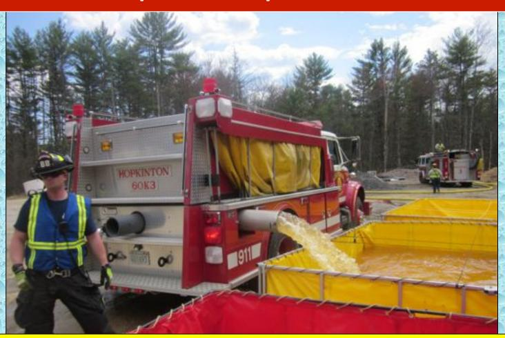
Two dump tanks are now in operation as the Hopkinton tanker dumps its 2,000 gallons of water.
