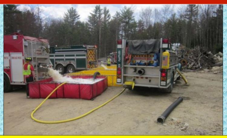
The operation moved to a 3-dump tank operation. The red tank is just 1,500 gallons in size and ended up being replaced with a larger tank in order to have greater storage capacity.
