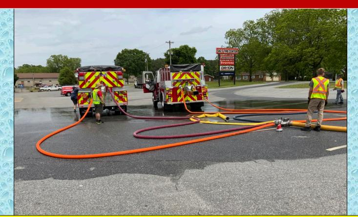
A good example of "connecting two but loading one" at the fill site. The hydrant supply was not capable of a 2,000 gpm flow (as few fill sites are) so the crews did a good job of focusing on filling one tanker at a time at the 1,000 gpm fill rate.
