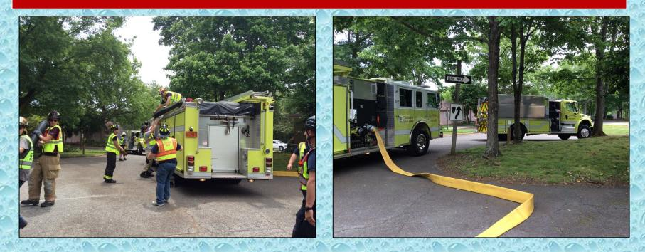
St Stephens Engine 42 arrives next and goes to work setting up to supply Conover Engine 4. The initial plan was to use tank water (1000 gal) until a dump site could be set up.
