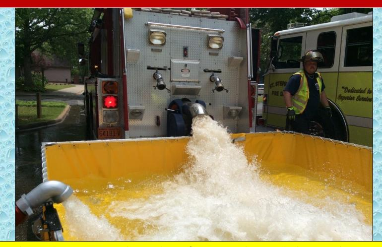
Maiden Tanker 1 engages the jet dump feature on the 8-inch dump and very quickly offloads its water. This jet dump was quite impressive!
