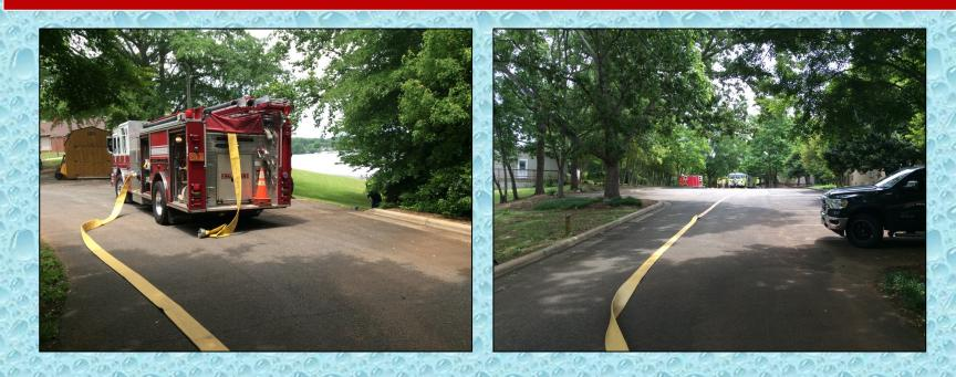
Conover Engine 4 arrives on the scene as the attack pumper and lays out a 5inch LDH supply line.
