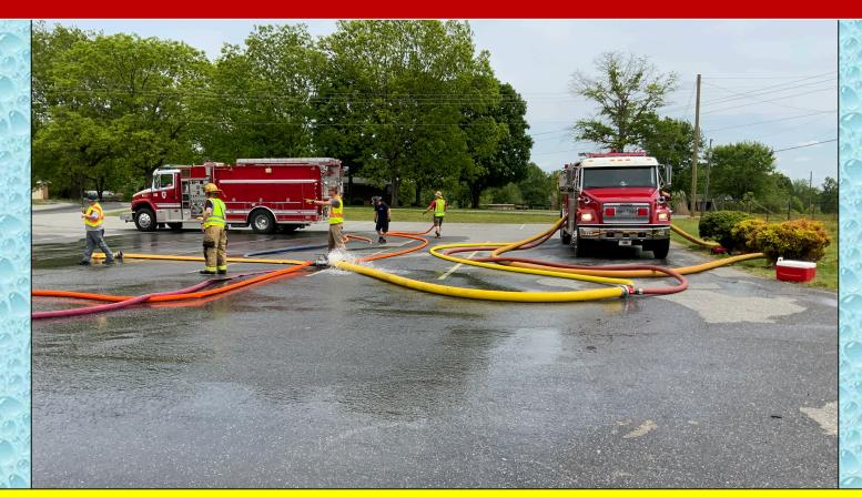
Oxford Engine 132 (1500 gpm) obtained water from the fire hydrant and then loaded tankers at the 1,000 gpm target fill rate.
