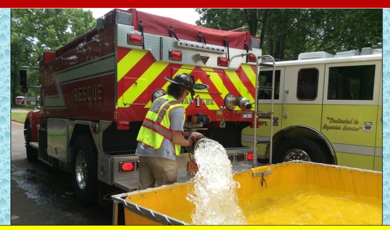
Additional tankers begin to arrive and off-load their water as the operation transitions to a dump tank operation. Flow was moved to 500 gpm around the 15-minute mark.
