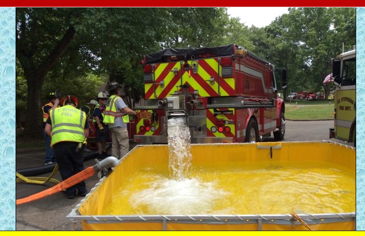
At the 5-minute mark, water flow was started at 250 gpm. At the 8-minute mark, the 1<sup>st</sup> dump tank is in operation.
