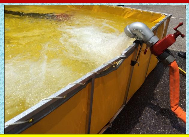
The use of a gate valve on the supply line holder allowed the folks at the dump site to control water flow into the primary dump if needed. It was never needed.
