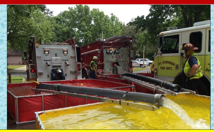
Around the 58-minute mark flow was moved to 600 gpm and then again to 850 gpm at the 69-minute mark. A three-dump tank arrangement was used to support those flow increases...as was the continued operation of Marine 13.
