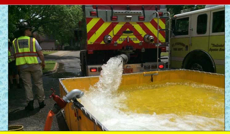
A supply line holder is placed on the primary dump tank in anticipation of Marine 13 supplying water from Lake Hickory to the dump site. Even though Marine 13 was limited in pump capacity, its contribution really made a difference in sustained water flow in between the arrival of tankers.
