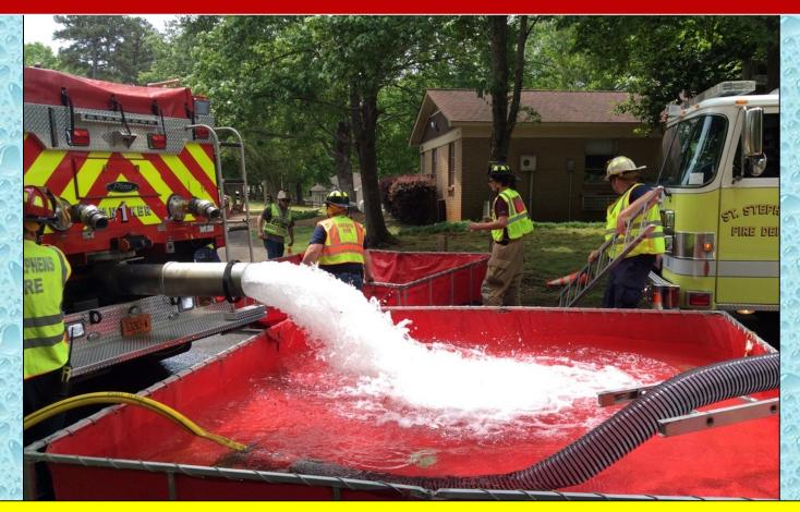
Around the 38-minute mark two dump tanks were in use and a third was being set up..
