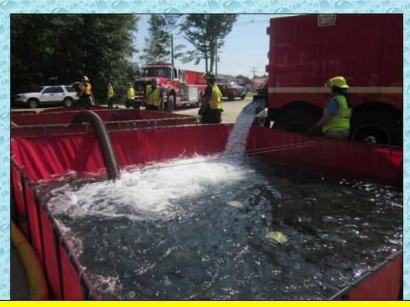
More resources arrive to offload water and crews continue to work to plan for the eventual expansion of dump site operations. Harrison Tank 6 offloads here at the 13:30 minute mark.
