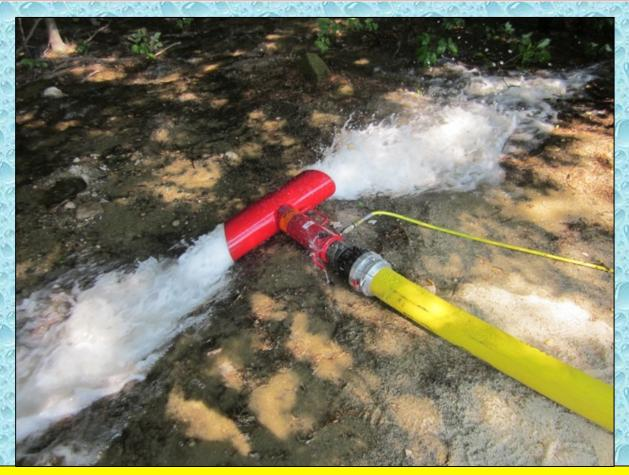
Flow was increased to 750 gpm at the 51:00-minute- mark.
