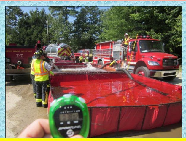
Around the 38:00 minute mark, all of the dumps tanks were pretty much full and tankers were waiting to dump their water. The decision was made to increase flow.
