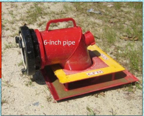
As it turns out, there were two types of low level strainers available. The one shown on the right (above) is the "high-flow" model. It was NOT used.
