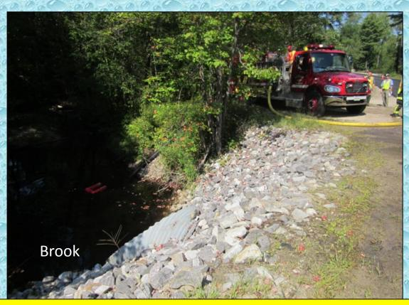
The crew was supposed to use a dry fire hydrant but it was out of service so they had to resort to drafting directly out of the brook. This required an additional length of suction hose – which the pumper did not initially have.
