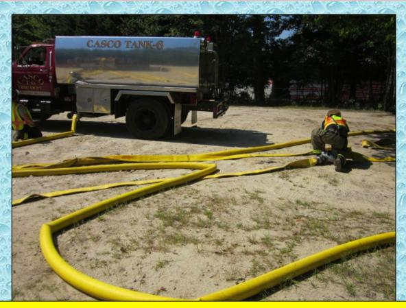
At the 5:30-minute mark, Casco Tank 6 (1,800 gallons) takes a position to operate as a nurse tanker if needed. The tanker crew sets up to supply the dump site pumper through 4-inch LDH and a double-clappered siamese.
