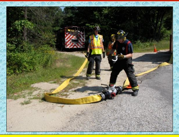
The Casco crew used a 5-inch LDH manifold to load the tankers coming to this fill site. The manifold allowed the loading to be controlled away from the pump panel.
