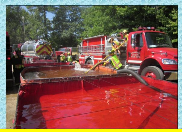
The low-level drafting strainer on the dump site pumper's suction line got flipped over when a tanker dumped its water in the primary tank. Fortunately, the crew was able to fix the problem without interrupting the water flow.
