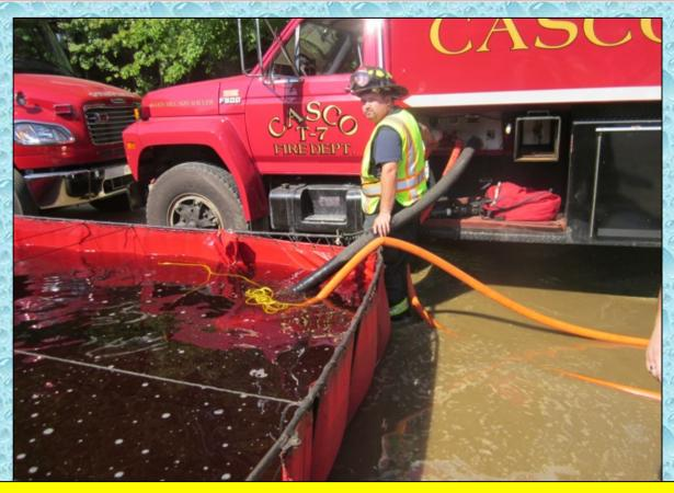
The goal was to try and increase the flow to 1,000 gpm. The dump site pumper was struggling to go above 800 gpm. The decision was made to take Tank 7 out of the water hauling loop and have them draft and run jet siphons.
