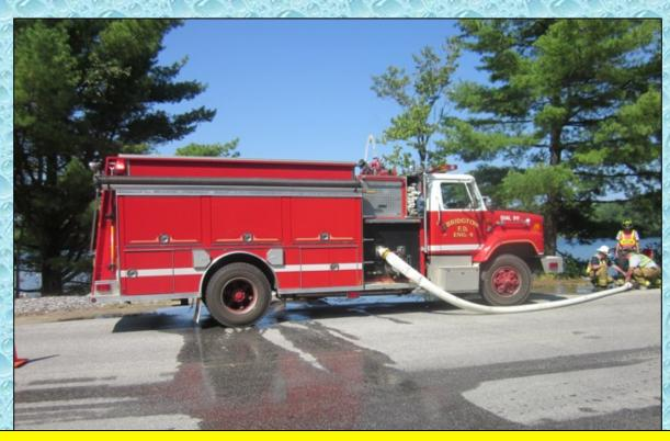
Bridgeton Engine 4 (1,500 gpm) operated the second fill site which was located on a large lake that had plenty of water access. The pumper had good positioning and there was ample room to load tankers.
