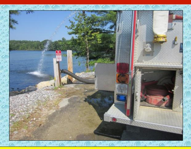
The fill site was established at a dry fire hydrant which provided plenty of water for meeting tanker filling rate requirements.
