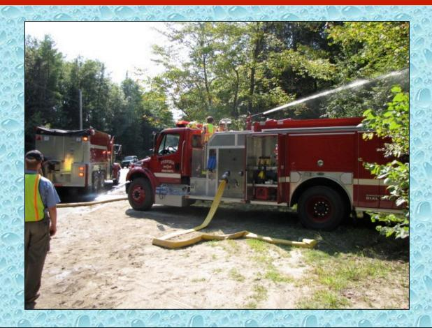
Otisfield Engine 3 (1,250 gpm) operated the third fill site and also filled tankers using 4-inch LDH.
