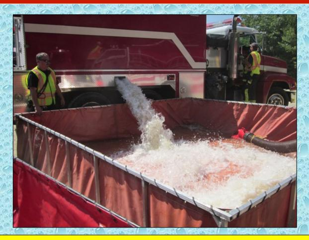
Raymond Tank 2 dumps its 3,000 gallons of water into the first dump tank at the 4:00-minute mark and drafting operations are about to begin.
