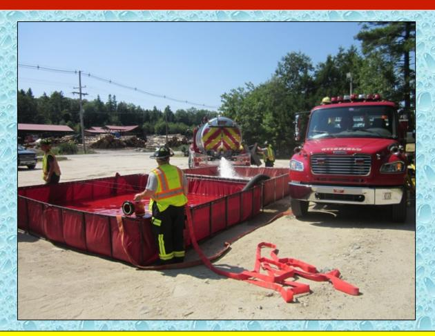
At the 12:00-minute mark, Bridgeton Tank 4 – a 3,000 gallon vacuum tanker – arrives on the scene an offloads its water into the primary dump tank.
