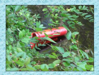
Engine 14's front suction inlet was used as the drafting inlet for the operation and a floating strainer was needed to access the pond water. The disadvantage of using a front suction inlet is that these inlets are not used in the rating of the fire pump and thus – they normally have restrictive flow – often times in the neighborhood of just 60% capacity. A better choice would be to use an extra length of suction hose and draft from a side suction inlet.
