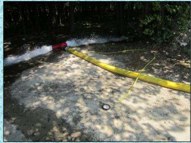
At the 5:00-minute mark, water flow was started at 280 gpm. A Hose Monster flow diffuser with fixed pitot was used to provide an accurate flow measurement.
