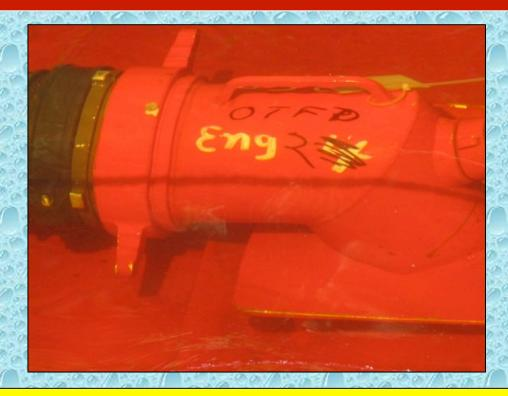
A problem occurred at the dump site pumper. Otisfield Engine 2 could not attain a 1,000 gpm flow. Several attempts were made to change the operation but nothing made a difference. The pumper could not get above 800 gpm. The problem? It was the low-level strainer that was being used on the pumper's suction line.
