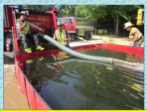
Casco Tank 7 offloads its 1,800 gallons of water using a little bit of a different approach before it was relocated to run jet siphons.
