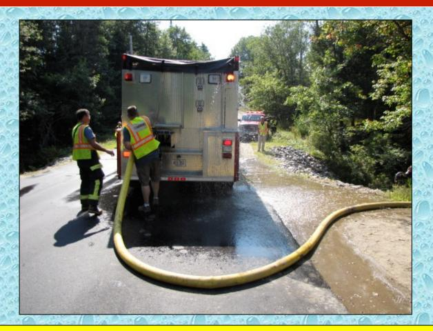
The loading crew did not have an LDH manifold to use so the pump operator had to be involved in the loading process.
