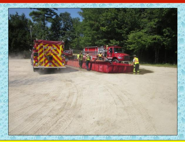
With the arrival of the additional tankers, the third dump tank was placed into service and flow was moved to 504 gpm at the 15-minute mark.
