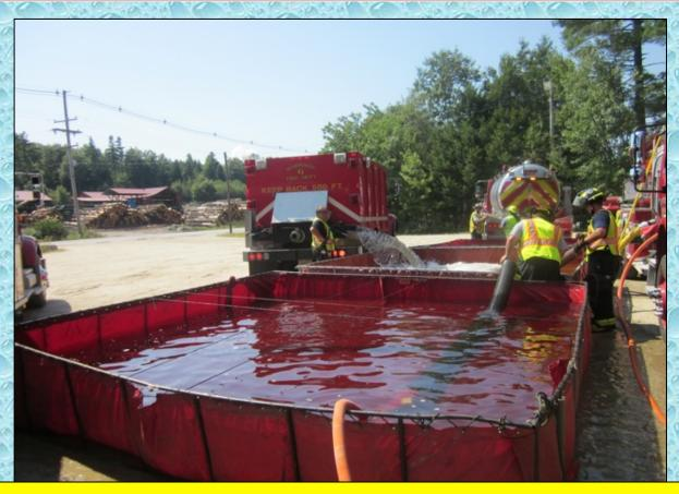
With the flow now at 750 gpm, crews had to hustle to keep the primary dump tank full and water transfer operations in sync with the demand. Harrison Tank 6 is shown here dumping its 3,000 gallons of water.
