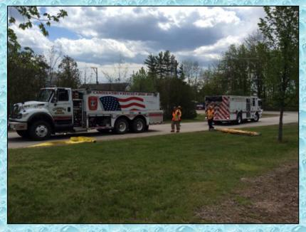
The drill began with Candia Engine 1 (left) arriving on the scene and laying a400-ft 4-inch supply line. Candia Engine 1 and Tanker 1 arrived soon thereafter and crews worked to establish a nurse tanker operation using a "rural hitch" set-up.
