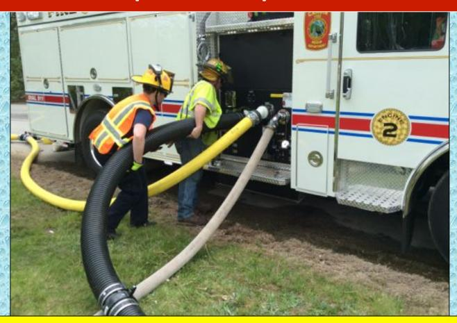
Around the 90-minute mark, a third suction line was added at Engine 2 which helped gain extra water for supplying Engine 1 while not working as hard to also supply the three jet siphons.
