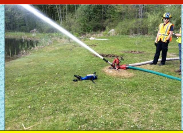
At the 62-minute mark flow was increased to 1000 gpm and three dump tanks were now in operation.
