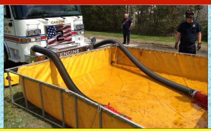
Engine 2's crew set-up to draft using twin, 6-inch suction lines; one from the front suction inlet and one from the driver side suction inlet. All of the new pumper's suction inlets were equipped with control valves which made this maneuver quite easy.
