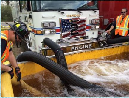
In the end, Engine 1 (1500 gpm) was able to draft through three, 6-inch suction lines, operate three jet siphons, and supply 1,000 gpm to the Engine 1 (attack engine).
