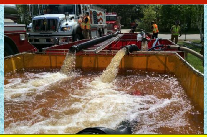
Water transfer operations were critical to the success of the operation. Three jet siphons were used to moved water to the primary drafting tank.
