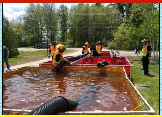
At the 20-minute mark, three dump tanks were down and one was in operation. Water flow was 500 gpm.
