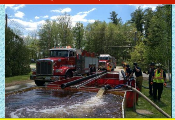
At the 60-minute mark, flow was moved to 920 gpm and all tankers were now hauling water in the shuttle.
