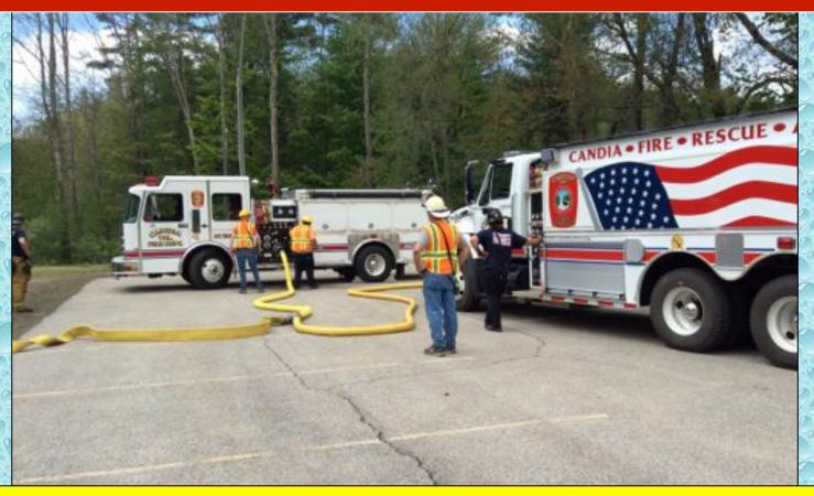
Tanker 1 co-located near the attack engine and supplied water via another double-clappered siamese until such time that Engine 2 switched over to a dump tank operation.
