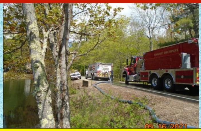
Candia Tanker 1 is shown being loaded at the pond fill site. Tankers at this site were loaded at 1000+ gpm using 4-inch LDH.
