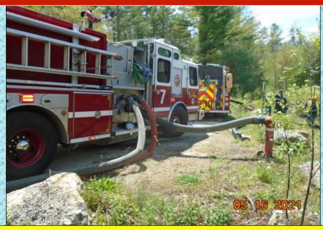
Manchester Engine 7 (2000 gpm) and Manchester Engine 10 (2000 gpm) worked to load tankers at the pond fill site.
