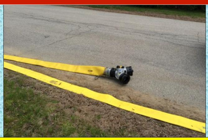
A double-clappered siamese was used on the end of the attack engine's 4-inch supply line.
