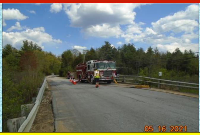
Auburn Engine 2 (1500 gpm) drafted off a bridge to access the stream. The crew loaded tankers using 4-inch LDH and at a rate in excess of 1000 gpm.
