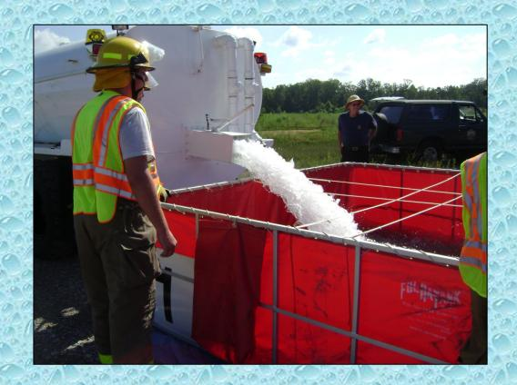
Water flow was backed down to 250 gpm at the 25:00 minute mark because of some issue with water transfer operations at the dump site. When those were fixed, flow was moved back to 500 gpm.
