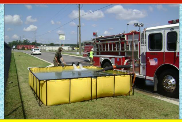
When a tanker arrived for filling, Engine 241 drafted out of the dump tank and filled the tanker. The rate at which the engine could draft and fill was faster than what the hydrant could have provided by itself. This "open" relay is very useful when faced with low flow hydrants.
