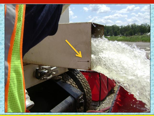
When the water hits the black line – the valve is closed and the tanker takes off for another load.
