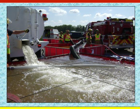
Around the 31:00 minute mark, the first tanker was back and ready to dump. Three dump tanks were also in operation by that time.
