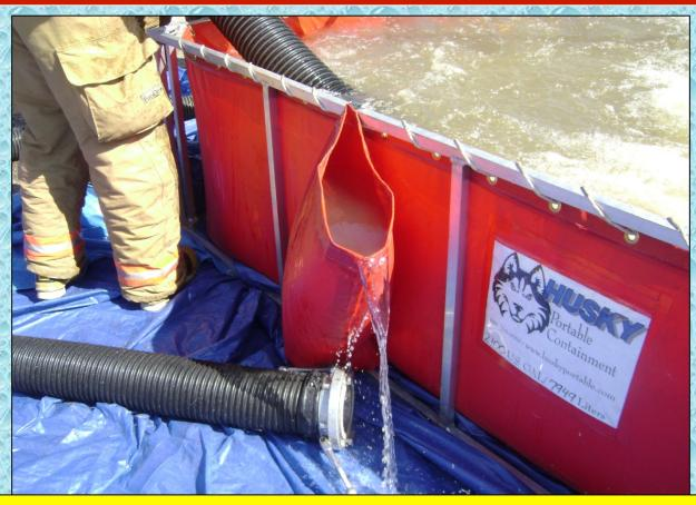
A common problem seen at many drills is the dump tank drain not secured. While it is unlikely to lose the contents of your tank, it does make a big mess which can cause problems during long term operations.
