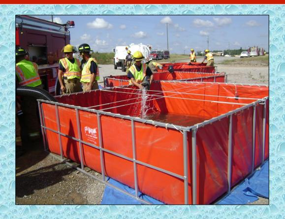
With three dump tanks now in operation, the water transfer process became important.
