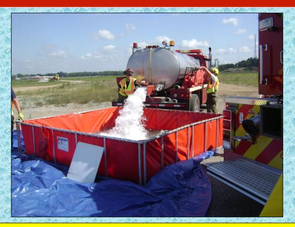
About a minute later, Pea Ridge Tanker 101 arrived and dumped its water and the operation transitioned to a tanker shuttle operation as opposed to a nurse-pumper-tanker operation.
