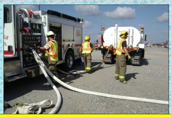
With the arrival of the first tanker, a decision was made to gravity nurse from the 2,200-gallon unit. This probably was not the best decision, because the rear 2-1/2-inch outlet could not support the 250 gpm flow being attempted. The tanker did have a 300 gpm pump, which most likely would have proven more useful – but it was not used.
