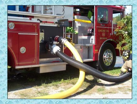
Engine 203 set up dual suctions so that its capacity would be improved. This once again illustrates the importance of carrying more than 20-feet of hard suction hose on rural pumpers.
