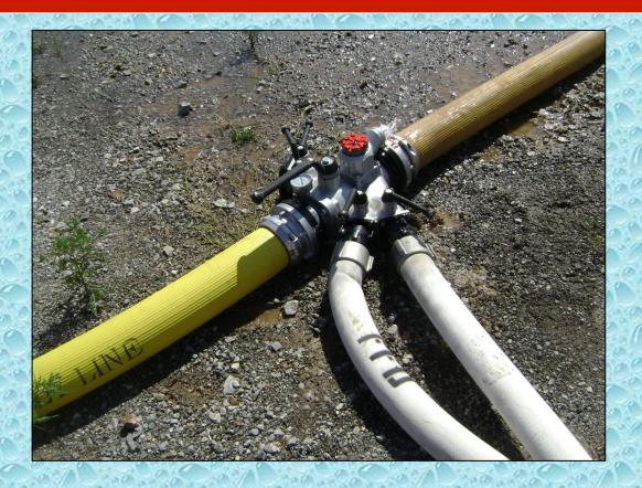
While not as efficient as a clappered device, this LDH manifold served its purpose quite well.
