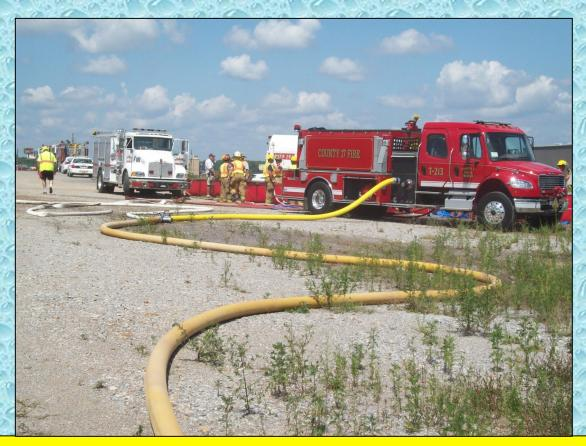
At the 108:00 minute mark, the flow was moved to 558 gpm where it stayed for the remainder of the drill.
