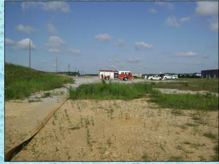
Meanwhile, Calera Engine 21 arrives and prepares to give its water to Engine 22 via the manifold on the 5-inch supply line. While this technically is not a nurse tanker operation – it uses the same principle. This is the advantage of having a control valve or manifold at the end of your LDH supply line.
