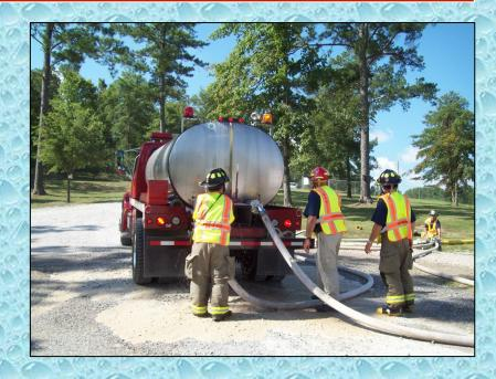
Use of an LDH manifold makes the "loader's" job so much easier. The valve allows for close control of filling operations with minimal impact on the pump operator.
