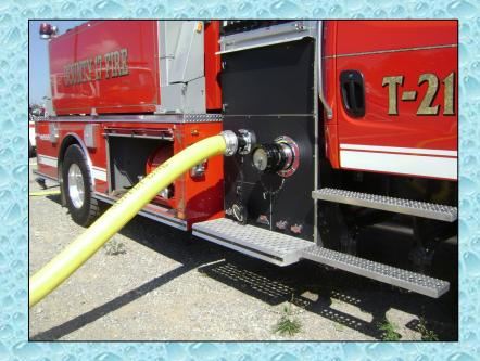
The LDH manifold that was originally laid out by the first arriving engine made a huge difference in sustaining flow. The pumpers shown on the left above, were able to pump off their water into the manifold without interfering with tankers trying to dump. County 17 Tanker 213 (right) used its hi-flow discharge to support the LDH manifold while drafting from the dump tanks.
