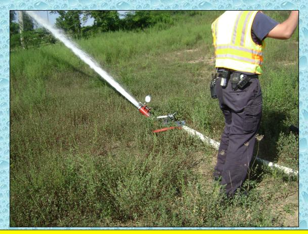
At the 3:59-minute mark (a bit early), water flow is started at 250 gpm using a fixed-pitot on the monitor for accuracy in flow measurement.
