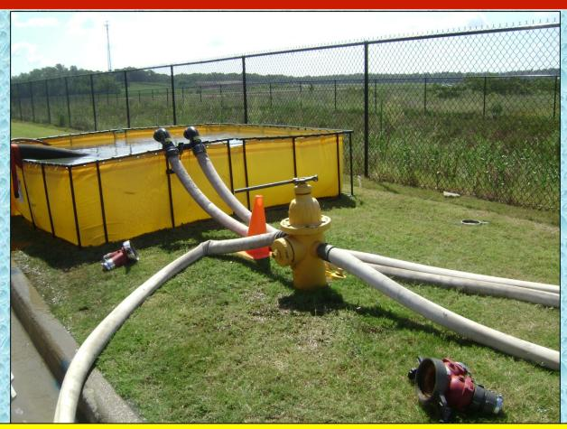
The site was set-up to simulate a low-flow hydrant (<1,000 gpm). The crew used a dump tank which was kept full via the fire hydrant.
