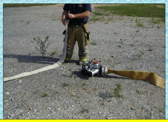
The use of the manifold at this drill made a big difference in sustaining the water flow. It allowed pumpers to pump off their water in lieu of blocking out tankers trying to dump at the dump site.
