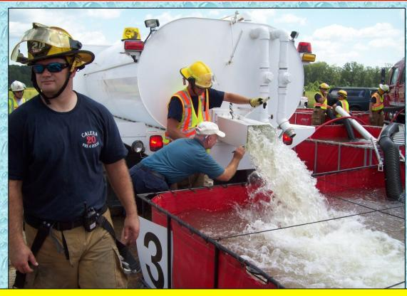
So at this drill, we marked a line on the dump chute to show folks when to stop dumping and get back on the road for another load of water. On a square dump and level ground, this normally occurs around the 1/4 –height mark on the chute.
