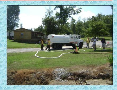
This tanker has dual fill lines each equipped with a check valve and camlock fittings. This arrangement allows for quick connect and disconnect operations.
