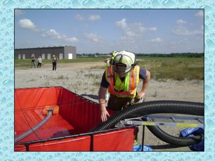
In order to support jet siphon operations, a brush truck was brought in to run a jet siphon. The problem that occurred was that the pump could not generate quite enough pressure to make the jet siphon work properly. So the brush truck was eventually removed from the operation.
