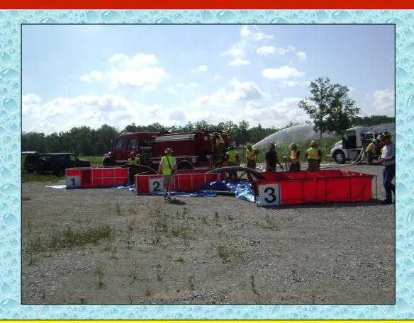
A third dump tank was placed into operation as additional tankers arrived and provided dump tanks. Note the use of the portable signs – they help the tanker drivers to identify what tank to dump into.
