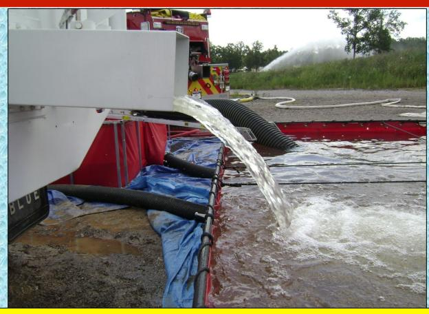
One question that often arises is, how long do you dump water? There is a point where the cost of waiting to finish off-loading outweighs the benefit of being on the road to get more water. In the photo above, that tanker needs to be on the road!
