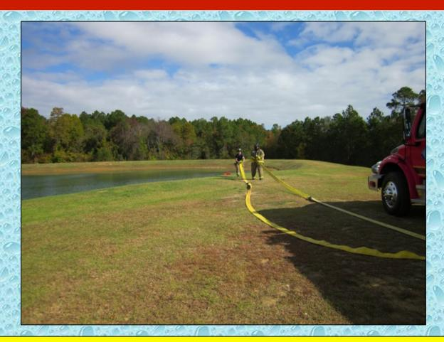
In preparation for water flow, Engine 34's crew stretched a 100-ft, 3-inch hose line to a Hose Monster flow measuring device.
