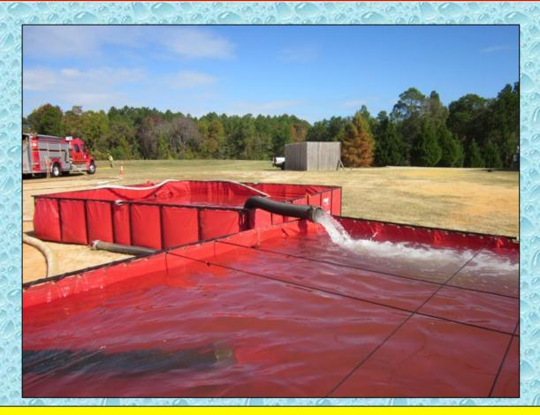
A jet siphon is the most common type of water transfer device used today and when properly pumped – its output should look like the output shown above.
