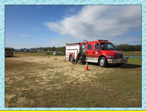
Engine 34's crew works to get ready to receive water from the dump site via a 4-inch supply line.
