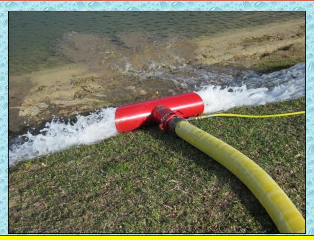
At the 5:00-minute mark, water flow begins at 280 gpm using a Hose Monster flow diffuser with a built-in pitot tube for accurate flow measurement.,
