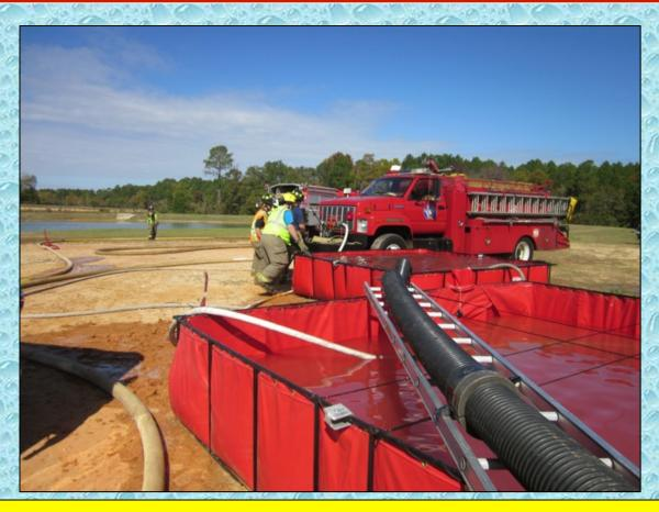
With the flow now at 750 gpm, Engine 31 was pulled from hauling water at around 104:00 minutes and put into operation helping to pump jet siphons.
