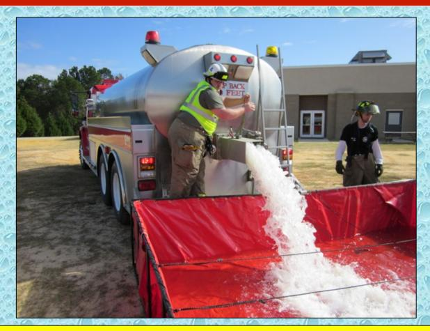
With the dump site all set-up, the first tanker dumps its water and operations transition from a nurse operation to a tanker shuttle operation.
