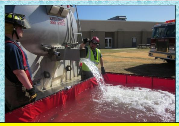
When the water level drops to this point in a tanker, it is time to stop dumping and go get more water. In fact, this tanker could have left about a minute or so sooner. Waiting for every last drop to come out actually reduces the tanker's efficiency.
