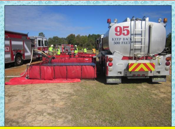
With four dump tanks now in operation, the flow is moved to 750 gpm at the 72:00-minute mark.
