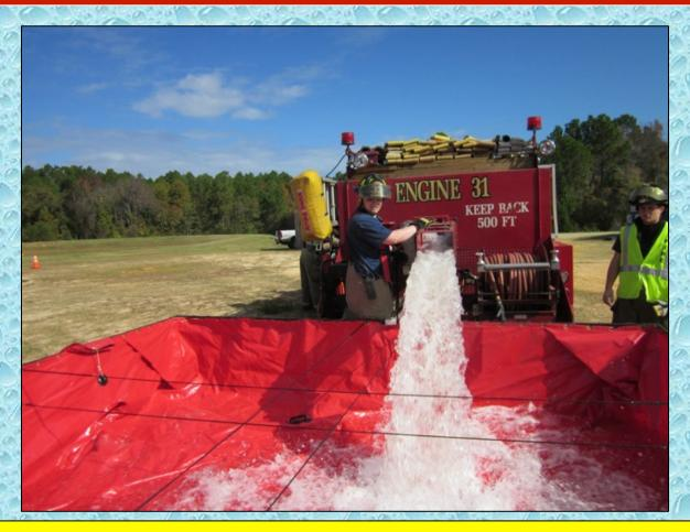
Around the 28:00-minute mark, the first tanker has returned from the fill site and dumps its second load of water.
