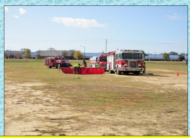
Additional units arrive and around the 2:54-minute mark, crews begin setting up the first dump tank – a 3,000-gallon tank.
