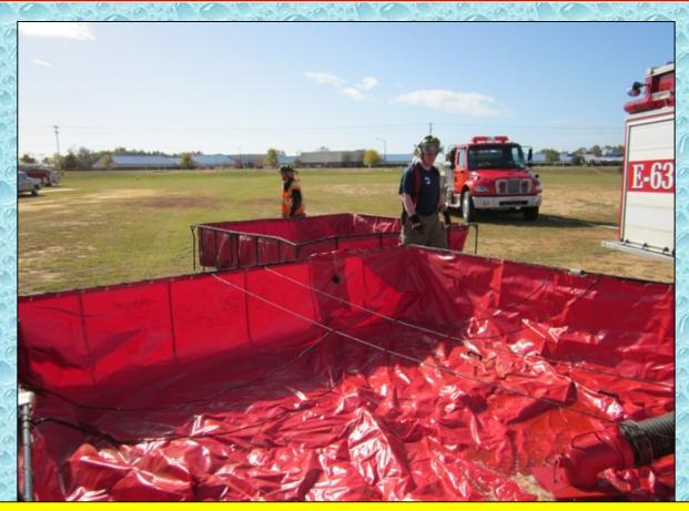
With the arrival of additional units, a second, 3,000-gallon dump tank was set up in preparation for moving to a higher flow at some point in the drill.
