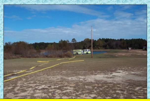
The fill site was set up and operating in just under 11:00 minutes after the arrival of Engine 83. Given the distance between the pond and the tanker loading area, some 4 or 5-inch LDH would have improved fill capabilities – however, this set-up still provided respectable fill times.
