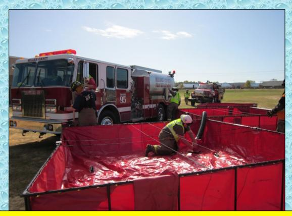
As units from the Tanker Task Force arrive, a third dump tank (2,100 gallons) is set up in order to further expand the operation. Water flow is also moved to 504 gpm around the 21:00-minute mark.
