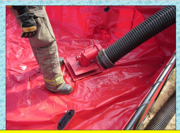
While working to set up water transfer operations so that the second dump tank could be placed into operation, a small problem arose – two different size fittings. This was resolved fairly quick.
