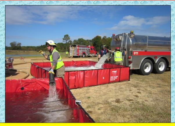
When using multiple dump tanks, water transfer operations become very important. Without a means by which to transfer water, water becomes "trapped."
