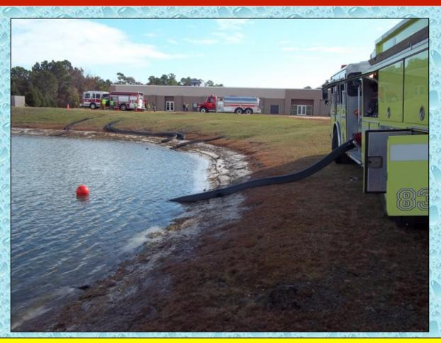
Two lengths of hard suction were needed to reach an adequate depth in the pond.
