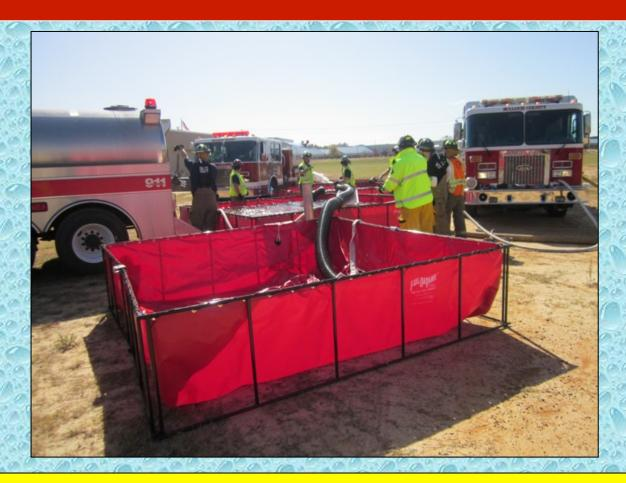
Around the 55:00-minute mark, a fourth dump tank (1,500 gallons) is put into position so that flow can be increased once again.
