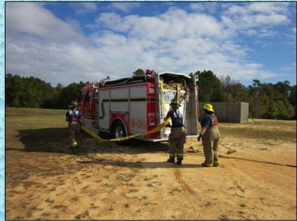
Engine 34 was the first unit to arrive. The pumper stopped and laid out 100-ft of 4-inch LDH. The timer was started when the pumper came to a stop.
