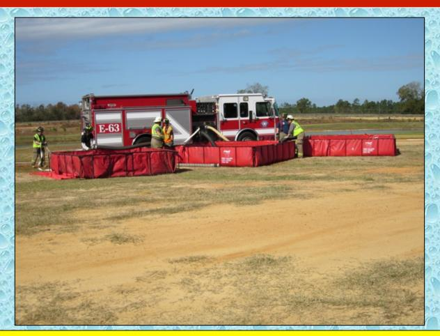
The dump site now has 8,100 gallons of storage capacity in the three dump tanks and water hauling operations have stabilized some.
