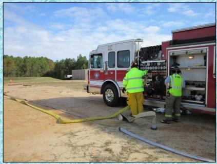
With water now flowing, the dump site pumper gets ready to supply the attack pumper using a "nurse" operation until the dump site can be made ready.
