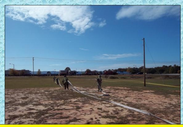
With the Turbo Draft in place, Engine 93's crew hand stretches two more fill hoses for tanker loading. One item to consider is that it may have been easier to "lay in" from the road when the pumper arrived rather than hand stretching back.
