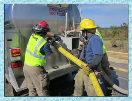
Dual fill lines were used to load the tankers – this helped to improve loading times since LDH was not available for use.
