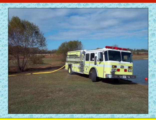
Engine 83 arrives at the fill site and immediately goes to work setting up for a drafting operation.
