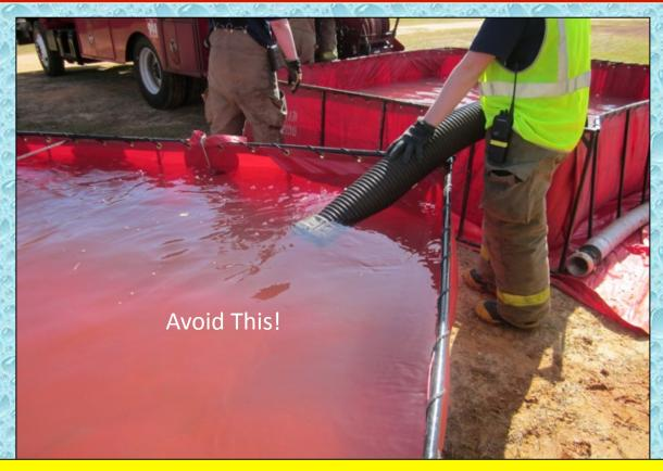
When using a jet siphon, avoid submersing the outlet end because the device will then act as a siphon when the tank is full and the device is no longer pumped. In other words – water will go back to where it came from!
