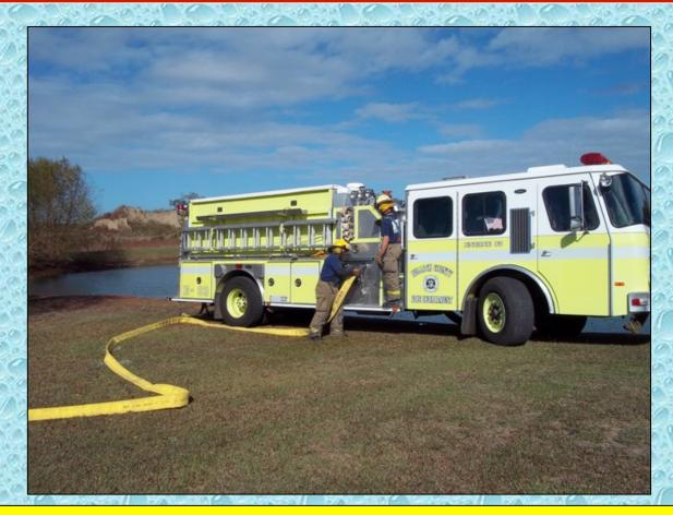
Crews switch the location of the fill hose from a rear discharge to a side discharge.
