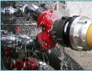
Also to improve capability, a clappered siamese was used because the pumper had no high-flow, LDH discharge. While no test data was gathered, the improvised set up seemed to work okay – short of some leakage.
