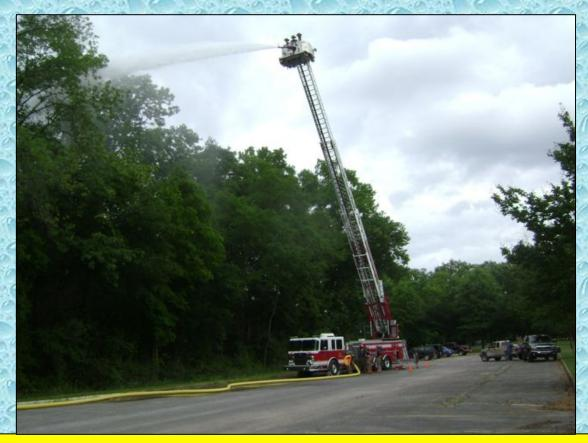
At the 24:30-minute mark, the flow was increased to 500 gpm and the tower's flow meter was used to monitor the flow rate of the water being discharged.
