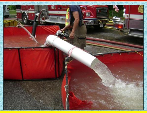
The pumper shown above was put into operation to run the jet siphons and supply a third, 3-inch line to the LDH manifold as a flow increase to 800 gpm was attempted.
