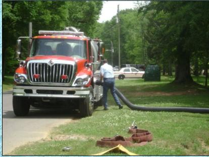
The 3,500 –gallon vacuum tanker arrives at the fill site and the driver – BY HIMSELF – makes the connection and fills the tanker at over 1,000 gpm! No fill site crew needed, which one of the key benefits of a vacuum tanker.
