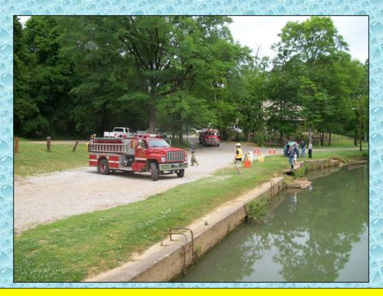
This creek provided plenty of water and plenty of access for drafting. Pea Ridge Engine 101 (1,000 gpm) is shown above arriving on scene and positioning to set-up to draft.
