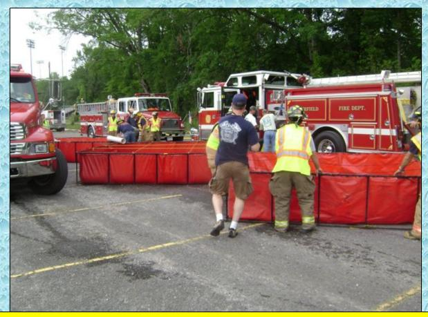
At the 14:11-minute mark, a third dump tank (2,100 gallons) is set into position and more units begin to arrive on scene.
