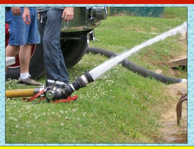
A portable monitor is used as a recirculation line – thus insuring a prime is not lost.
