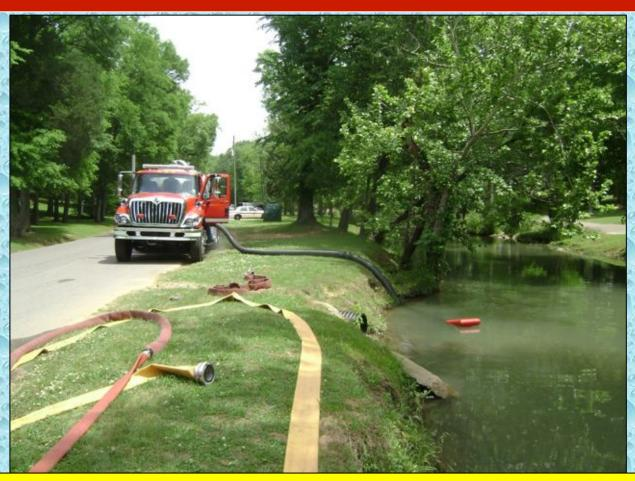
The vacuum tanker carried 30 feet of hard suction and it was used along with a floating strainer to access the creek.
