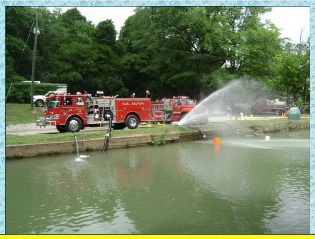
Both pumpers are shown in operation – each supporting a tanker fill station.
