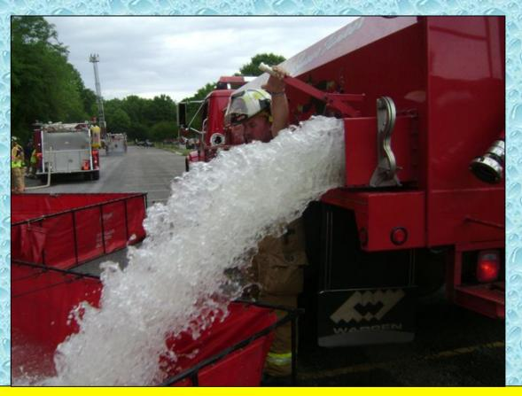
At the 21:00-minute mark, Tanker 200 returns from the fill site – the first tanker to return. The tanker is shown above dumping its water into the primary drafting tank because water levels are running low.
