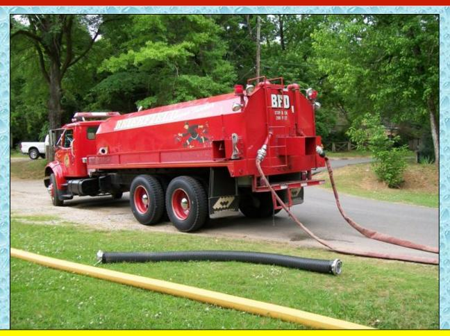
The fill site was ready when Tanker 200 arrived —which was the first tanker empty. Tanker 200 was filled using dual, 3-inch fill lines.
