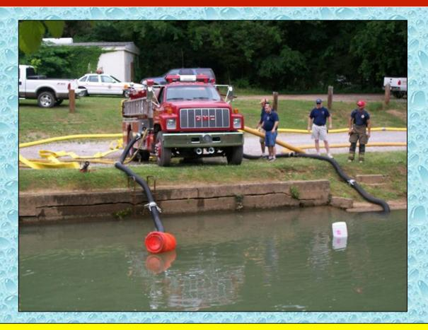
Pea Ridge Engine 101 is set up to maximize its ability to draft and supply water for filling tankers. Great Job!
