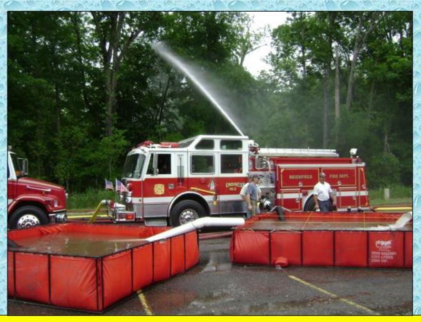
Around the 51:00-minute mark, a small snafu occurred at the tower and water flow was diverted to Engine 202's deck gun at 500 gpm.
