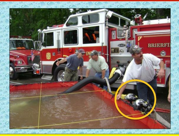
A couple of pumpers were used to haul water and they pumped off their water to the "gooseneck" fittings attached to the primary dump tank.
