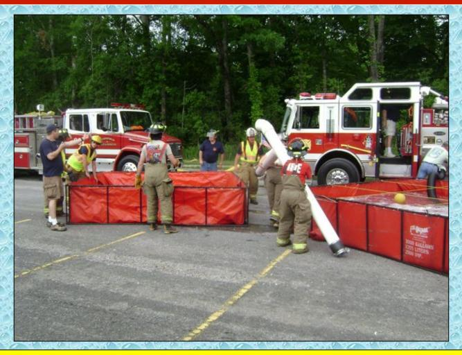
A second tank (2,100 gallons) is set-up as the dump site continues to expand.
