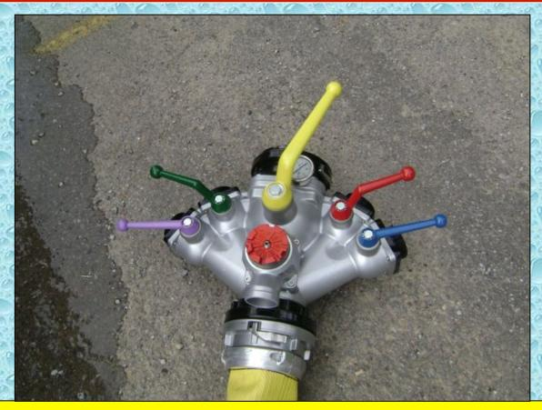
"Hey Johnny, go shut down this 2-1/2 at the manifold." Hey Johnny, go shut down the blue line at the manifold." Which one is easier for the new guy to do? That is why color coding can really simplify operations.
