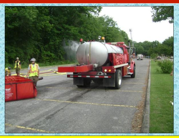
At the 9:51 minute mark, Pea Ridge Tanker 101 arrives at the dump site and positions to offload its 1,850 gallons of water.
