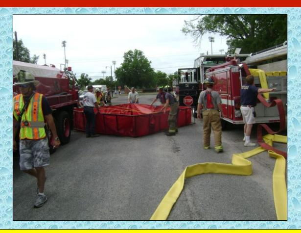
The first tank down was a 3,000 gallon one and crews work quickly to get the dump site set-up.
