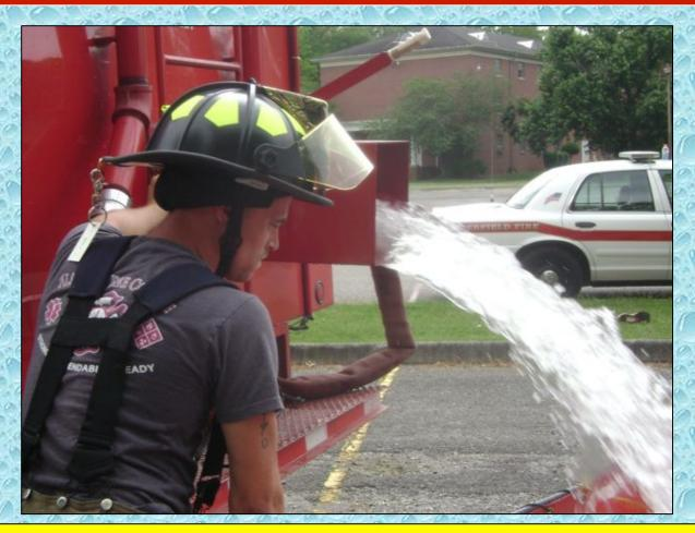
Tanker 200 dumps its load as Engine 202 works to get a prime. Timing is everything during the first 15 minutes of the ISO drill.
