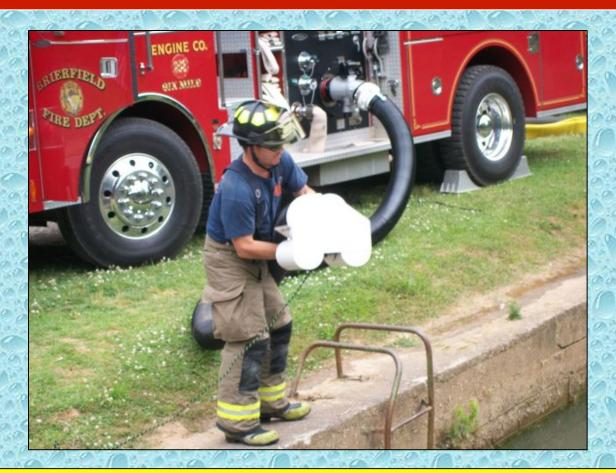
Brierfield Engine 203 (1,500 gpm) sets up to support the operation of a second fill station. Above, a high-flow, floating strainer is shown being deployed.
