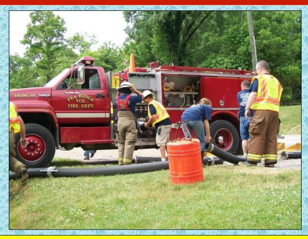
To improve the capability of this 1,000 gpm pumper, both the driver and officer side suctions were used.
