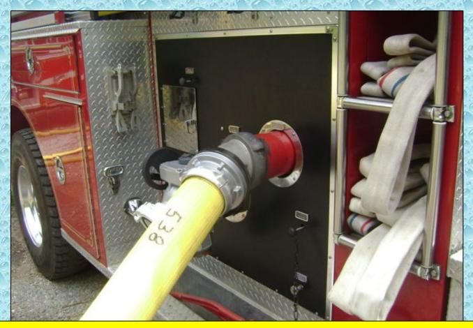
A good example of a high-flow discharge in use. When designing or rehabbing a pumper, a high-flow discharge is an item that should always be included.
