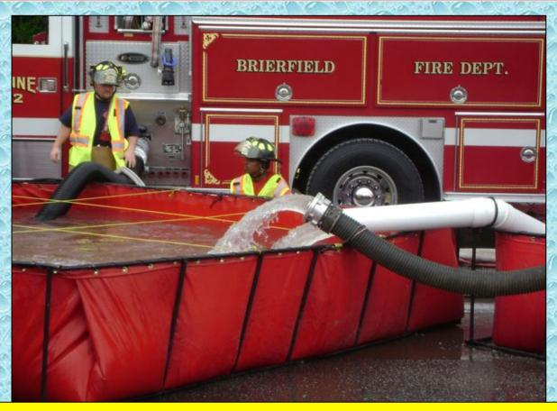
Of course, as flows increase – so does the need for transferring water from tank to tank. Therefore, additional jet siphons - and perhaps an additional pumper might be needed.
