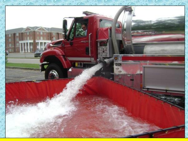
One of the features of the drill was a 3,500-gallon Water Master vacuum tanker provided by the folks from E-One. The tanker is shown above offloading its water under pressure.
