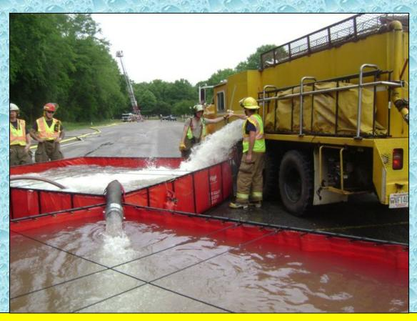
The photo above is a good depiction of transferring water. The jet siphon shows a solid stream of water - which should be in the neighborhood of an 800 to 1000 gpm flow.
