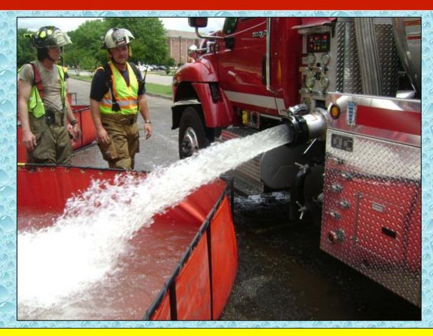
The Water Master vacuum tanker is shown above with its powerful offload capability. Its 6-inch dump can dump at a rate of 1,750 gpm when the tank is pressurized.
