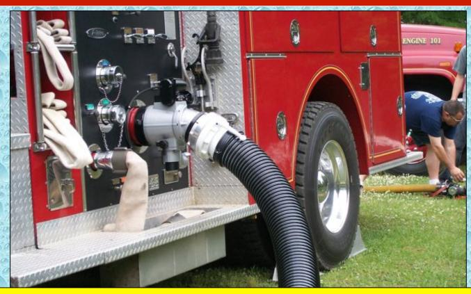
This TFT intake valve is rated for suction operations and is controlled by an electric motor. In addition, the use of the long-handled, Storz suction fittings makes it easier for the driver/operator to make and break suction hose connections.
