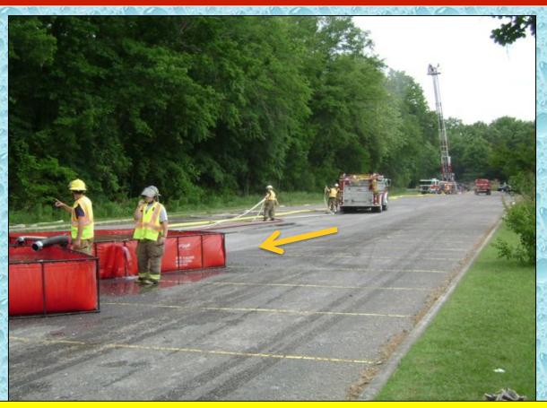
The pumpers hauling water pulled past the dump tanks and pumped their water back to the site via dual, 3-inch lines. This prevented the pumpers from blocking out the tankers who were trying to dump their water.
