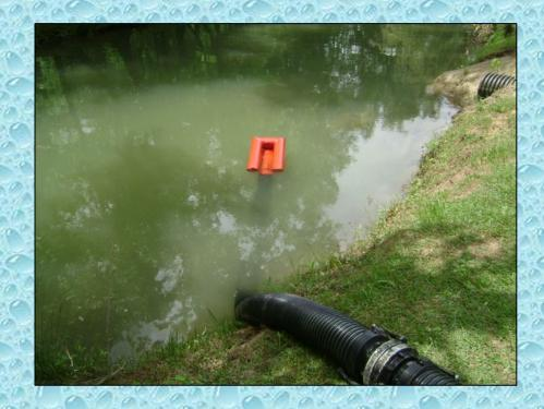
At first glance, it appears as just some extra suction hose laying around. It actually is the fill site for the vacuum tanker. Once deployed – the equipment is left in place for each return trip.
