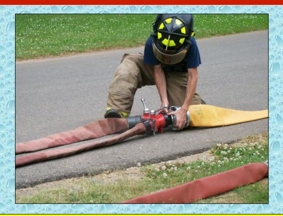
If a manifold is not available – then traditional devices can be used – assuming the correct adaptors are present.
