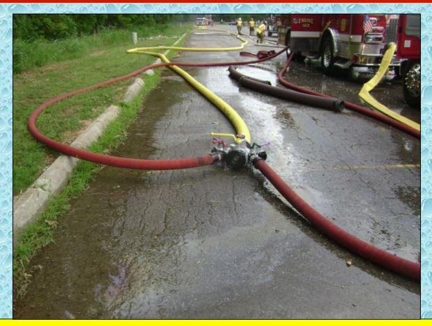
After troubleshooting a couple of items, water is finally sent to Montevallo's tower. Two, 3-inch lines from Engine 202 were used to supply the LDH manifold.
