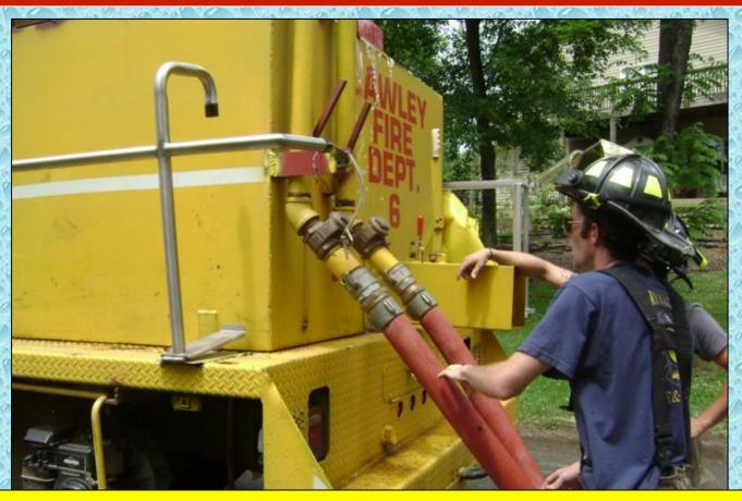
Lawley's 3,250-gallon tanker has dual fill lines, each with a check valve as the control point. The tanker is shown above being filled at the tanker fill site.
