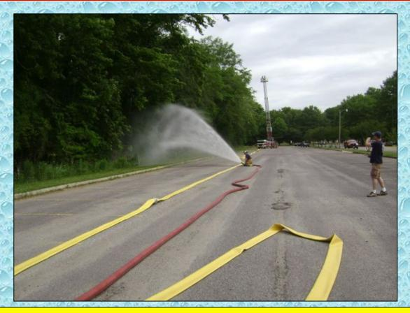
At the 6:45 minute mark, water flow is started to the rapid attack monitor using the tank water from the two engines.
