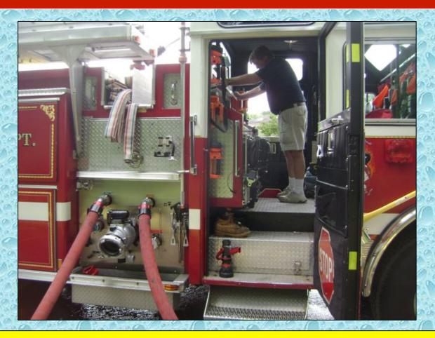
The pump control panel for Engine 202 is located inside the cab – a feature not often seen in Alabama. As usual, the dump site pump operator got a workout!
