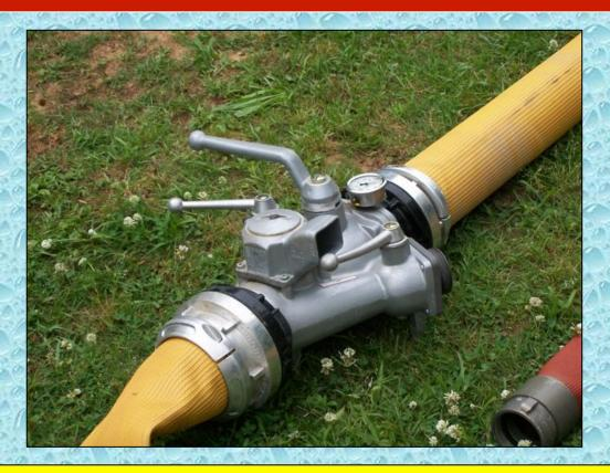
When using LDH for tanker fill operations, a manifold is always helpful – it provides control over the water flow, a pressure gauge for accurate supply pressure settings, and a relief valve.
