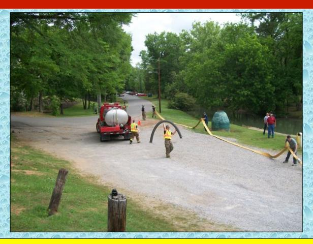
Folks are shown deploying a 5-inch line to use as a tanker fill station. Others are shown bringing equipment to the draft pumper.
