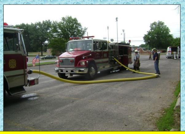
Engine 201 sets up to supply Engine 202 with its 1,000 gallons of water. When combined with E202's 500 gallons, this should provide about 5 to 6 minutes of a 250 gpm flow once the 5-minute start point arrives.
