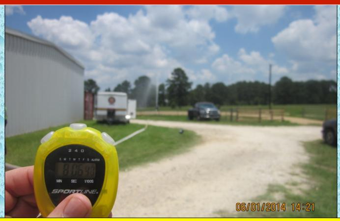
Water flow got started a little bit late because of a primer issue with the dump site pumper. Once the primer was able to be activated, flow was started at 250 gpm using a TFT Blitzfire.
