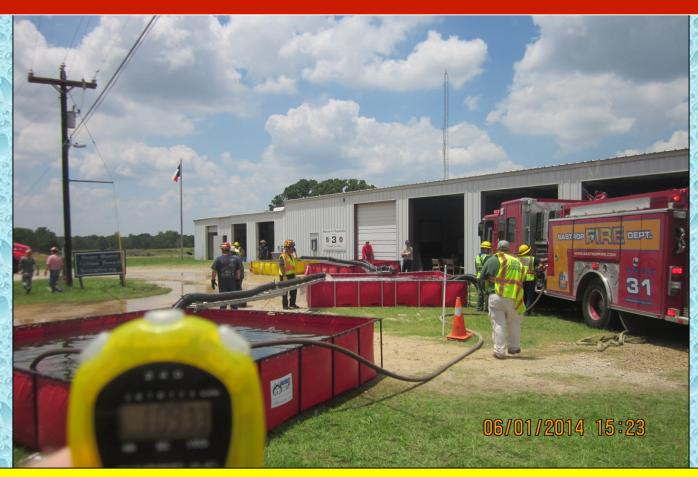
The operation is in "full-swing" at 1,000 gpm and once again, no tenders dumping. Crews at the fill sites had to "step it up" a bit – which they did.
