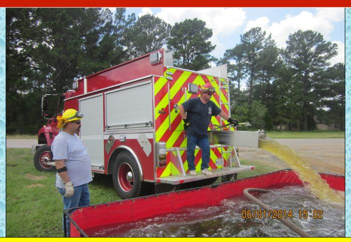
Ferrara Fire Apparatus provided a 2,000 gallon tender for the drill and folks took turns driving and operating the rig during the shuttle.
