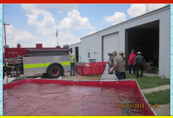
At the 15:00-minute mark, flow was moved to 500 gpm and a third dump tank was placed into operation.
