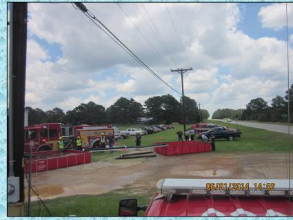
At the 46:00 minute mark, all four dump tanks were now in operation and plans to move to a 1,000 gpm flow were underway.
