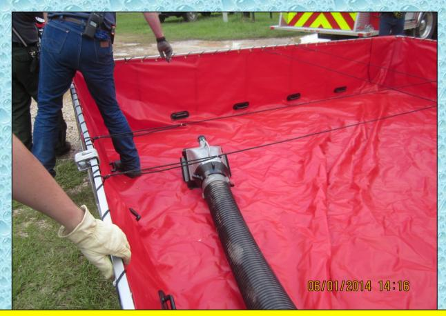
The crew worked quickly to get the first dump tank set up and ready for water. The goal was to conduct the operation without the use of a nurse tender.
