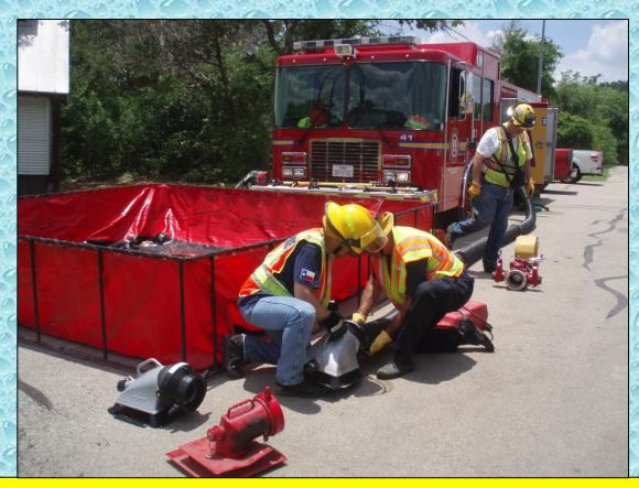
During the set-up process for this fill-site, crews used the side suction inlet to ensure maximum flow. They also used a TFT low level strainer as their suction strainer of choice.
