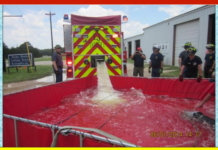
Lake Jackson Tanker 1 dumps its first load of 3,000 gallons and the dump site pumper begins drafting operations.
