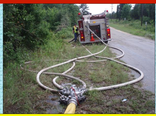
The Smithville engine did not have a high-flow discharge, so they pumped four, 2-1/2-inch lines into a reversed LDH manifold and filled tenders at a 1,000 gpm rate.
