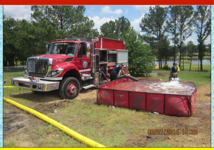
District 5's Tender 119 (1,000 gpm) was used as an engine instead of a water hauler. This fill site also used an open relay set-up to provide water for drafting.
