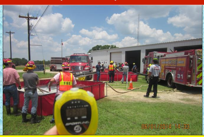
Three dump tanks are in operation and plans are underway to expand to a fourth tank in expectation of flowing 1,000 gpm. The dump tanks are nicely spaced out to accommodate multiple tenders at the same time.
