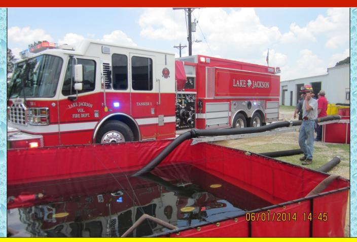
Lake Jackson Tanker 1 positions to dump its third load of 3,000 gallons. The tanker was brand new and the crew brought it to class to practice using it.
