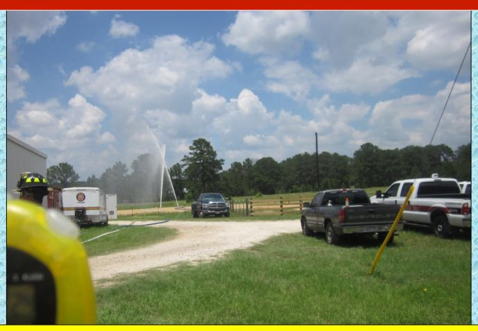
At the 91-minute mark, flow was moved to 1,575 gpm using both the portable deck gun and the Blitzfire.
