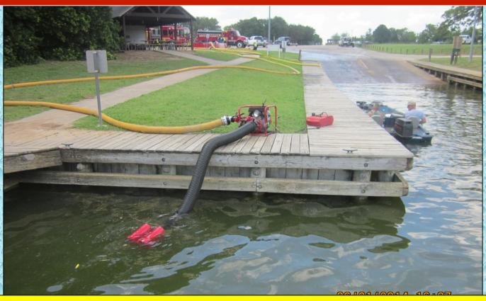
This fill site used a 500 gpm portable pump and a TurboDraft to support its tender filling operation. Both devices pumped water into a 3,000 gallon dump tank from which a 1,750 gpm drafted and filled tenders. This "open relay" is a great tool for using lower flow devices to support a 1,000 gpm fill rate.
