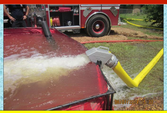
The two supply lines were then fed into a jumbo siamese and then into a single-5-inch line that supplied the dump tank.
