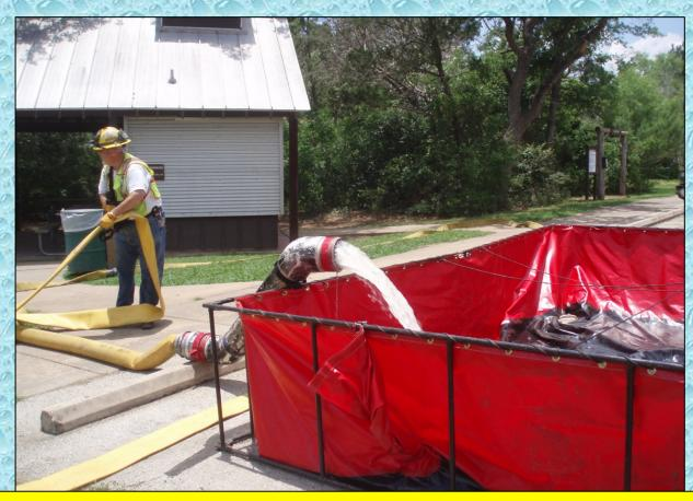
The discharge flow from the TurboDraft was directed via 5-inch LDH into this homemade tube which allowed water to be pumped into the dump tank.
