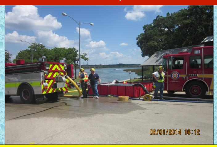
Bastrop Engine 241 operated as the fill site pumper and drafted from the 3,000 gallon dump tank. Tenders were filled at rates over 1,000 gpm using LDH.
