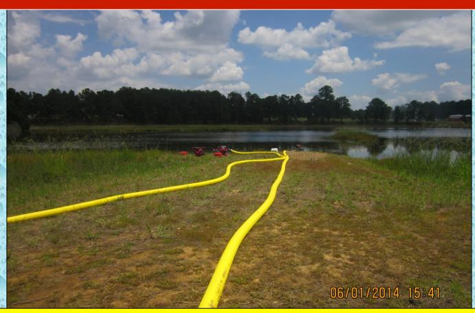
A 250 gpm and a 500 gpm portable pump were used to draft out of the lake and pump water back to the dump tank via 5-inch LDH.
