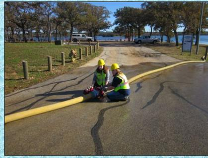
A 5-inch LDH line outfitted with a manifold was used to fill tenders at this site. The tenders were filled at rates over 1,000 gpm.
