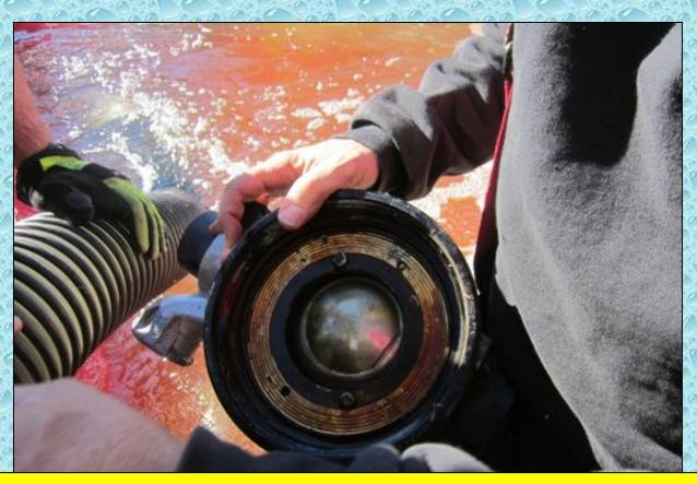
The inside of the external control valve shows why flow was limited. The valve fits on the 6-inch threaded suction inlet but the ball opening is only about 4-inches – thus flow was limited.
