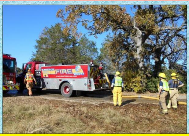
The fill sites used 5-inch LDH to load the tenders. One of Bastrop FD's 2,000-gallon tenders is shown here being filled at over 1,000 gpm.
