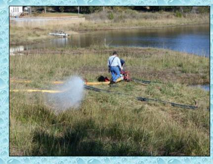
This fill site was perhaps the most interesting because it required the use of two portable pumps in order to meet the 1,000 gpm fill rate goal. Crews used two, 500 gpm CET portable pumps to feed water to a 3,000-gallon dump tank from which a 1,750 gpm pumper drafted and loaded tenders.
