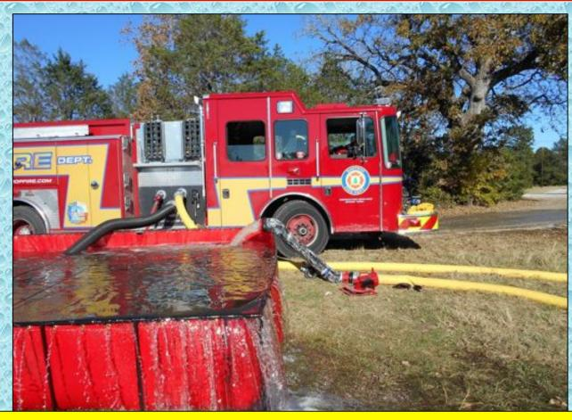
Bastrop Engine 241 (1,750 gpm) drafted from the 3,000-gallon dump tanker and filled tenders at a rate over 1,000 gpm. This type of set-up is often called an "open" relay.
