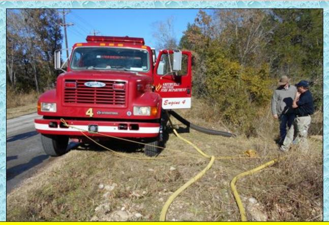
Smithville Engine 4 (1,250 gpm) established a draft where water passed under the road through a culvert. The lift was less than 10-feet and the water was clean and plentiful.
