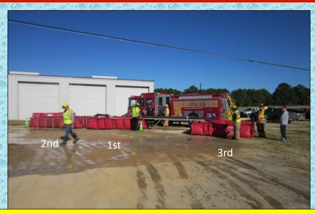
With three dump tanks set-up, the operation was ready to increase flow as needed. The third tank was positioned a bit farther away in order to permit two tenders to offload at the same time.
