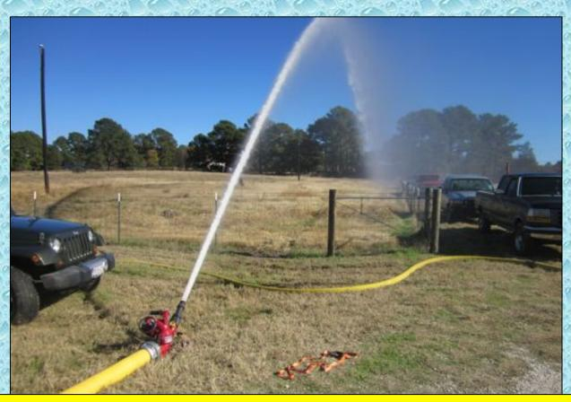
At the 60:00 minute mark, flow was moved to 1,067 gpm using a portable ground monitor fed by 5-inch hose from the pumper's high-flow discharge. The flow to the Blitzfire was stopped.
