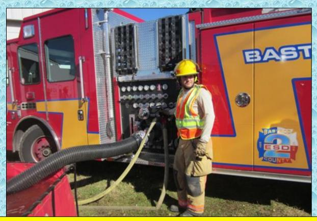
Engine 231's 1,750 gpm pump had plenty of capacity to support the fire flow and to run two jet siphons. A gated wye was used on a 2-1/2-inch discharge to supply the two jet siphons.
