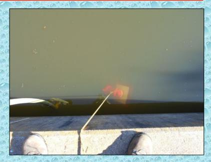
No barrel strainer was available, so a low-level strainer was used. However, the strainer restricted flow to under 1,000 gpm.
