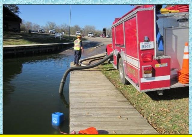
The lake water was clean and deep and the lift was minimal. Had this been a real incident, the pumper would have positioned on the boat ramp.
