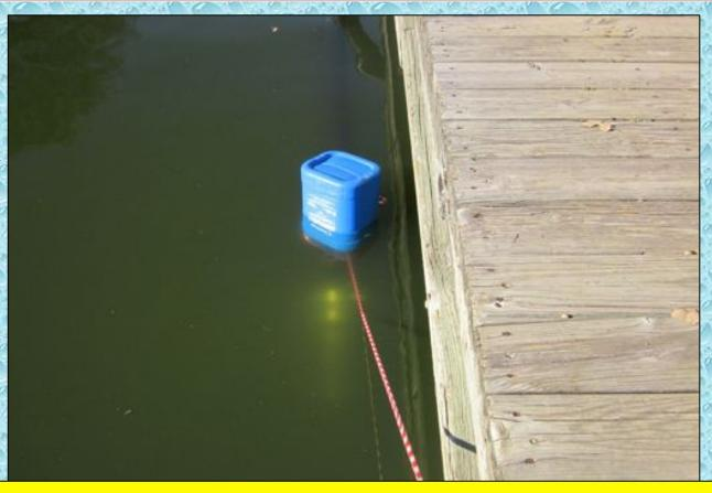
An improvised float was made using an empty 5-gallon foam container. The float helped keep the barrel strainer from resting on the lake bed.
