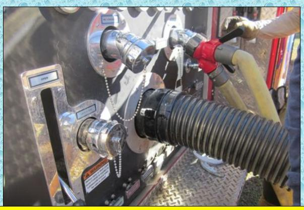
While trying to increase flow, crews found that the external control valve was limiting intake capabilities. So the valve was removed and the suction hose was connected directly to the steamer inlet. This made a huge increase in flow!
