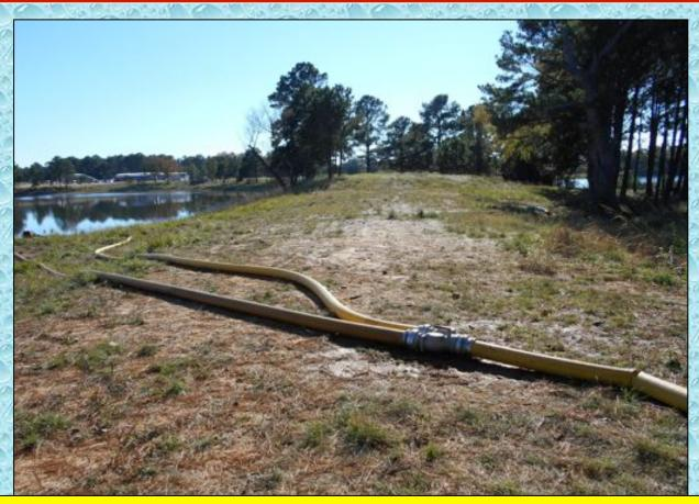
The two pumps fed this 5"x5"x 5" double-clappered siamese which in turn supplied a single-5-inch line to the portable dump tank.
