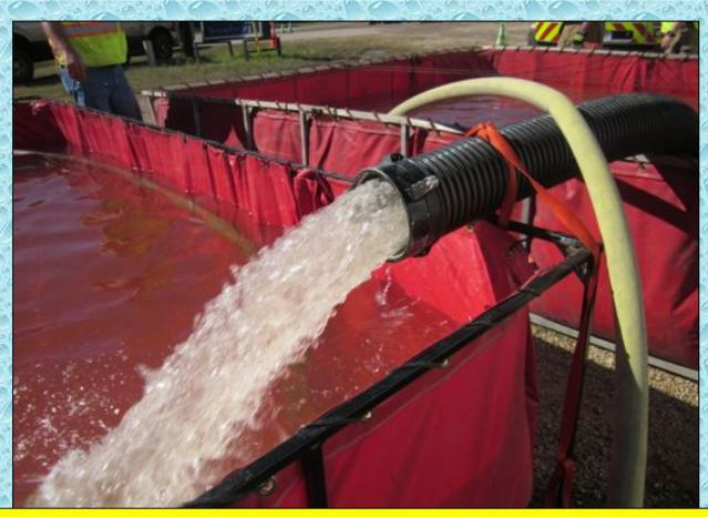
A good looking jet siphon stream! At the 15:00 minute mark, flow was moved to 500 gpm and then again to 720 gpm at the 17:00 minute mark.
