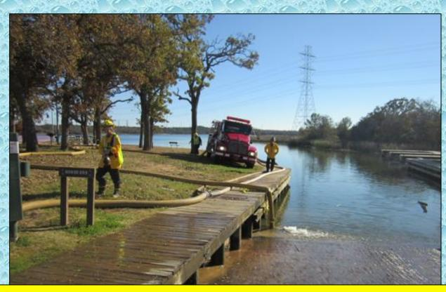
Heart of Pines Engine 871 (1,250 gpm) backed into position along this boat launch area and took draft from the lake. The 5-inch line going into the water is a circulating line. The line had previously been set-up for a different use; however, its use was changed to circulation.
