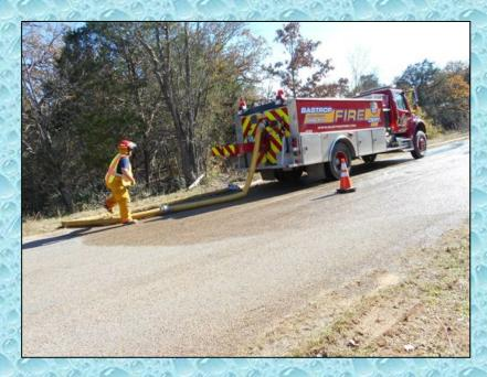
Tenders were filled using 5-inch LDH supplied by a single, 2-1/2-inch discharge – which also restricted the available flow. The best fill rate for tenders at this site was about 850 gpm – which is still respectable.
