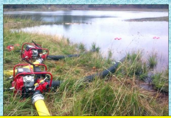
The pumps were gasoline powered and equipped with 6-inch suction hose. The pumps discharged their water into 5-inch LDH which supplied a siamese.
