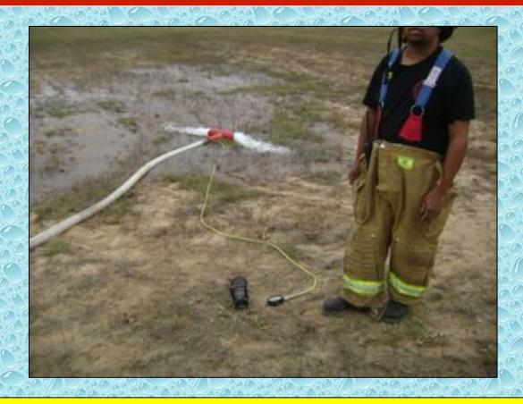
At the 5-minute mark, water flow begins at 282 gpm through the fixed pitot device.
