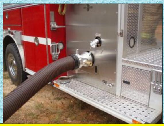
Because the dry hydrant was finished out with a female swivel, a double female adaptor was needed back at the suction intake to complete the hook-up.
