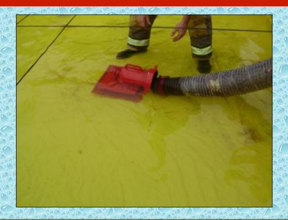
Another issue that arose at the dump site was the lack of a low level strainer. One was quickly found, but a delay occurred. The use of a low level strainer allows access to more water in a dump tank than using a traditional strainer.
