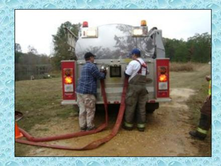
Crew members used dual, 3-inch lines for tanker fill operations. However, the lines were not equipped with any type of quick connect couplings – so the couplings had to be threaded and unthreaded each time.
