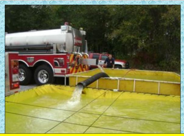
A 6" low level strainer equipped with a built-in jet siphon was used to transfer water from the second tank into the primary drafting tank.
