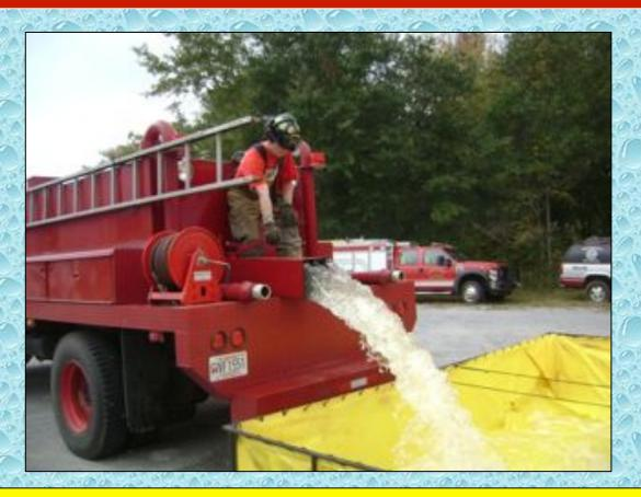
Booth's tanker dumped the first load of water so that Independence's engine could obtain a draft and begin the dump site operation.
