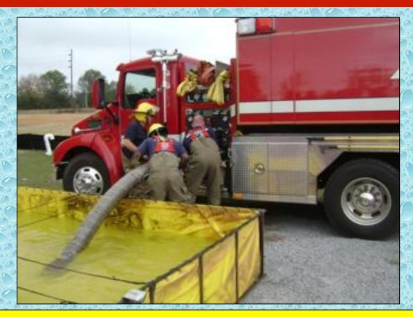
One problem that occurred was that Engine 901 did not have a control valve on either of its suction intakes and since it was being used as a nurse tanker for Engine 902, flow had to be interrupted in order to connect the suction hose.
