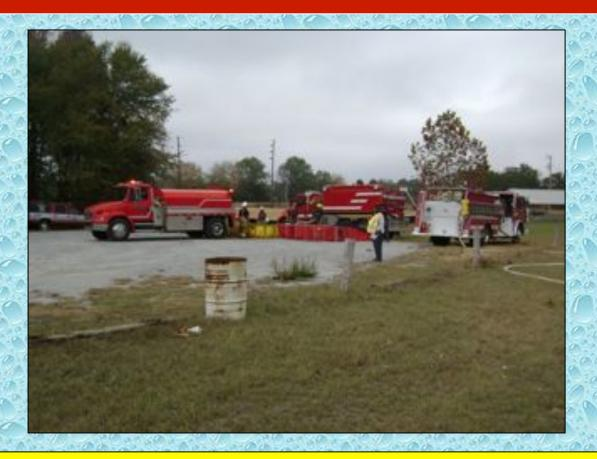
With the dump site now fully operational, the flow was moved to 470 gpm around the 35-minute mark.
