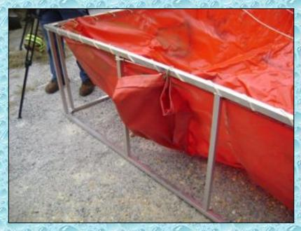
While there is no "written rule" for how to secure dump tank drains, it seems that the better practice is to tie the drains up on the inside of the tank. Doing this allows the weight of the water to hold the drain closed. Tying the drains up on the outside of tank often leads to leakage – and an eventual mess at the dump site.
