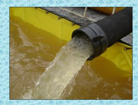
Of course, the key to any multiple, dump tank operation is the ability to transfer water to the primary drafting tank. Jet siphons seem to be the best practice for this transfer of water. Many pump operators ask about the pressures needed to run a jet siphon – the answer is simple – pump the jet siphon line until the flow looks like the flow in the photos above.
