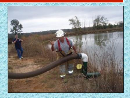
A temporary dry hydrant was used at this fill site and the crew needed one section of 6-inch suction hose to make the connection.
