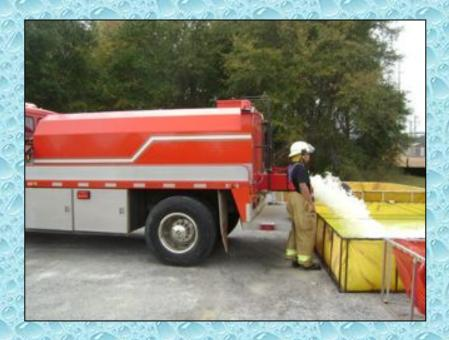
Pine Level's tanker arrived next and dumped its water. This 2,000-gallon tanker has a short wheelbase which makes it quite maneuverable on the back country roads of Autauga County.
