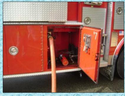
Another adaptor issue arose – this time a tanker had a 5-inch direct fill but no way of connecting to it. Instead, a 3-inch line has to be connected to an auxiliary suction intake. Another good reminder to equip engines and tankers with plenty of adaptors – especially when they serve duty in the rural arena.
