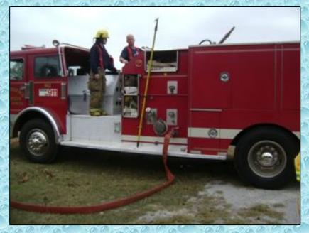
With the clock running, the two engines switched positions in order to improve the dump tank set-up choices. E901 with its 3,000 gallons of water began nurse tanker operations and supplied E902 via dual, 3-inch lines.
