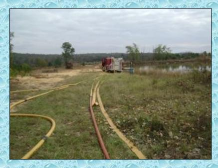
Once a draft was obtained – the South Fill Site was quite functional. Two additional 3-inch lines were stretched so that a tanker could be connected while another one was being filled.
