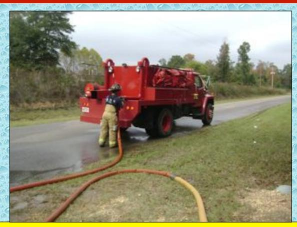
The Booth tanker was unique in that it did not have a control valve on its fill lines – but it worked just fine. The use of camlock connections made filling this tanker a quick operation.
