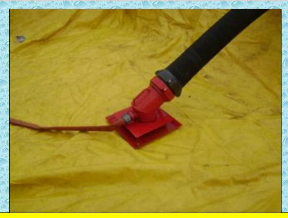
As more units arrived at the dump site, a second low level strainer (with jet siphon capability) was located and placed in the second dump tank to begin water transfer operations.
