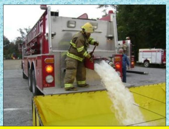
Independence's Tanker 982 (3,000 gallons) was the second tanker to arrive on the scene. The crew dumped their water into the primary dump tank in support of maintaining the fire flow.
