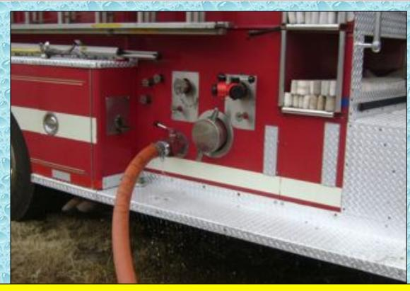
E902 also had no control valve on either of its steamer intakes – therefore, the 3-inch supply lines had to be connected to the auxiliary intakes. While this worked out okay for this drill, direct connection to the steamer intakes will provide much more flow capability to the pumper.
