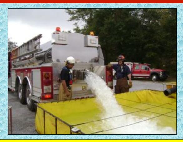
Now with additional tankers arriving, the focus was turned to making the second dump tank operational.
