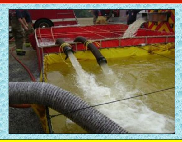
Dual, 4-inch jet siphons were needed to provide adequate water transfer from the third dump tank.
