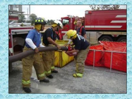
When Pentecost's tanker arrived at the dump site, an additional low level strainer/jet siphon became available – it however, was 4-inches in diameter and therefore required the use of 4-inch suction hose.
