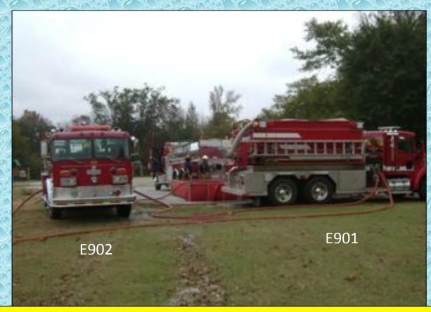
Although E901 never hauled a load of water in the shuttle, its use as a nurse tanker helped provide an uninterrupted flow for most of the 2-hr drill.
