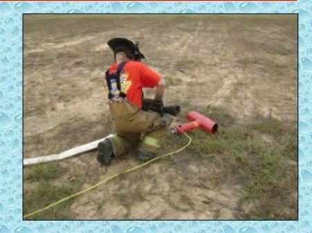
A 150-ft, 3-inch line was stretched to a Hose Monster device which was outfitted with a fixed pitot for accurate flow measurement.
