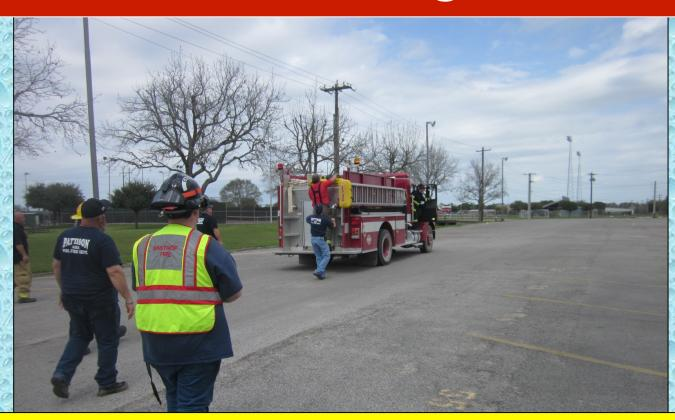
New Ulm Engine 1106 was the first-arriving unit and assumed the role as the attack pumper. The crew stopped to lay a 400-ft, 3-inch supply line before setting up to operate an attack line. The stopwatch was started when the New Ulm engine driver applied the air brakes.
