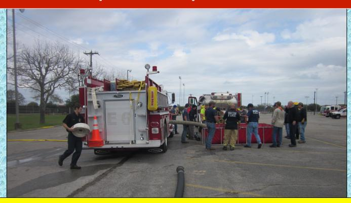
As additional units arrived on the scene, folks helped set up dump tanks. In the meantime, Bellville Engine took position as the dump site pumper and was prepared to supply tank water to Engine 1106 through the 400 ft of supply if needed. Pattison Tanker 2 (2000 gal) was the first tanker to dump a load of water.
