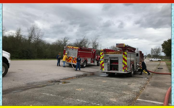
Eventually, a pumper arrived at the fire hydrant and was able to support the loading operation. Cat Spring Engine 803 (1500 gpm) was able to take water from the fire hydrant and load tankers at a rate of 1000+ gpm.
