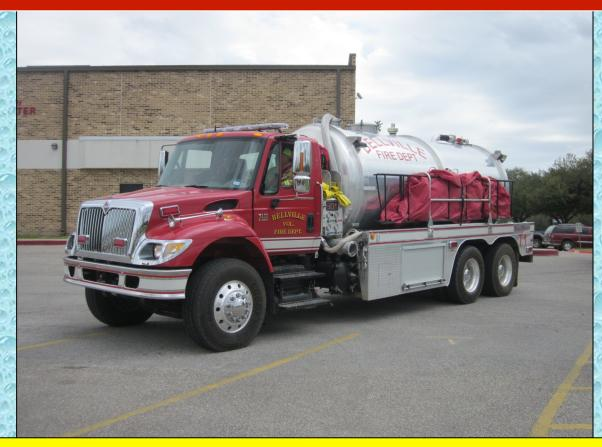
Bellville Tanker 1 (3500-gal) was the only vacuum tanker in the drill. As expected, the vacuum tanker proved quite effective in hauling water, especially when it came to self-loading at the fill site.
