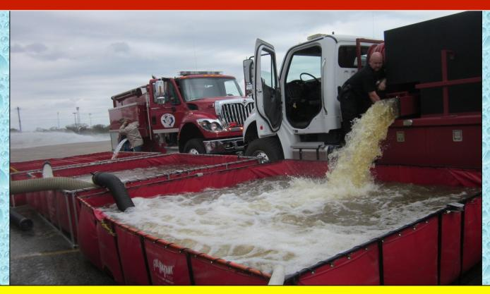
Knowing when to "cut and run" is important in tanker shuttle work. A typical 2,000-gal gravity dump tanker dumps most of its water in the first 60 to 90 seconds. Waiting 3 minutes to dump all water actually reduces the efficiency of the tanker.
