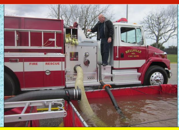
To help gain more output capacity, Engine 6 added a 3-inch suction line which helped to support the jet siphons and thus increase output to the attack pumper.
