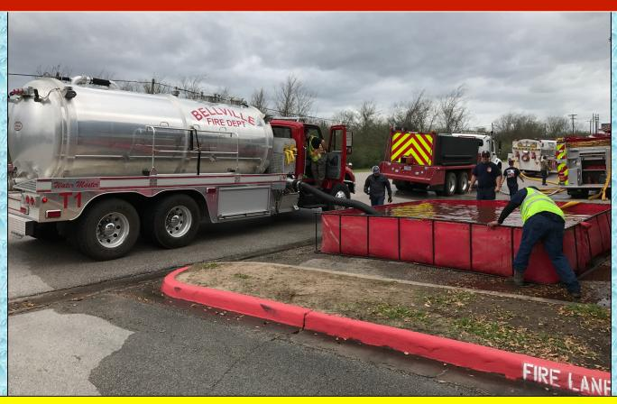
The hydrant was also used in an "open relay" manner to fill a 3500-gal dump tank from which the vacuum tanker filled each time. The self-loading feature of the vacuum tanker is the key to its success in a water hauling operation.
