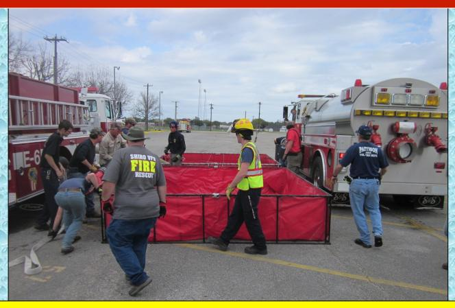
Cat Spring Tanker 804 (2100 gal) was the second tanker to arrive. Crews grabbed the tanker's dump tank while the tanker prepared to dump its water.
