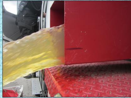
The black line on this dump chute indicates to the driver/operator when to "cut and run" for another load of water.
