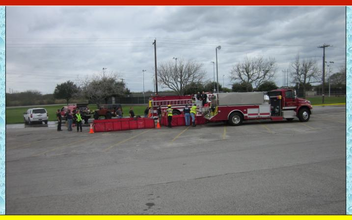
At the 92-minute mark, flow was moved to 1180 gpm at the attack engine and the arrival time of tankers at the dump site grew further and further apart.
