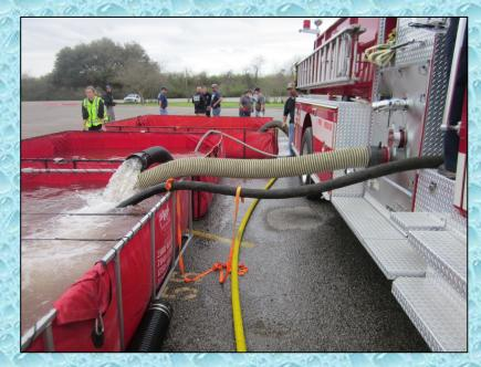
In order to reach the 1180 gpm flow at the attack engine, the supply engine went to a third suction line – a 6-inch line from the other side of the pumper.
