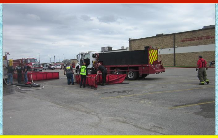
Units on the second Tanker Task Force arrived. The 4,000 gallon dump tank from the Blieberville tanker was grabbed and set-up. Flow was moved to 560 gpm at the 20-minute mark and then to 800 gpm at the 80-minute mark.
