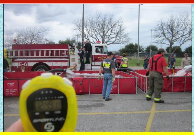
At around the 13-minute mark, three dump tanks we down and in operation. Water flow was increased to 400 gpm at the 15:00 minute mark.
