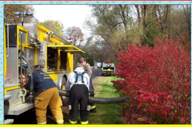
The crew used a 6-inch dry fire hydrant to access the pond. The pumper was unable to achieve 1,000 gpm from the dry hydrant – most likely due to sediment build-up around the suction strainer in the pond. A flow of around 850 gpm was the most achieved.
