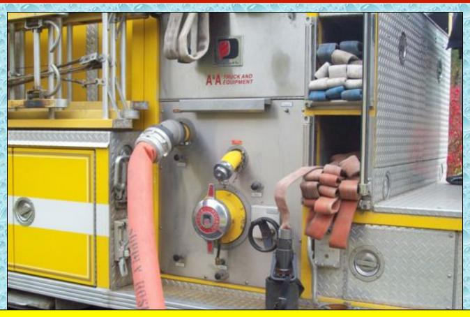
The Panama pumper was a 1,250 gpm pumper de-rated to 1,000 gpm. However, it was equipped with a 3-inch high-flow discharge and was able to support a good flow (850 gpm) to the 4-inch LDH fill line.
