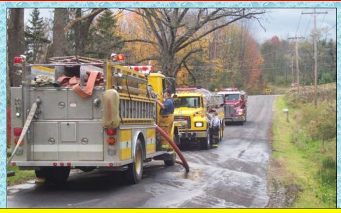
The Victoria Road fill-site was a good example of operating on narrow roads and the need to have a traffic management plan. Once the site was operational, all tankers were directed to travel in the same direction because of the limited space available for passing.
