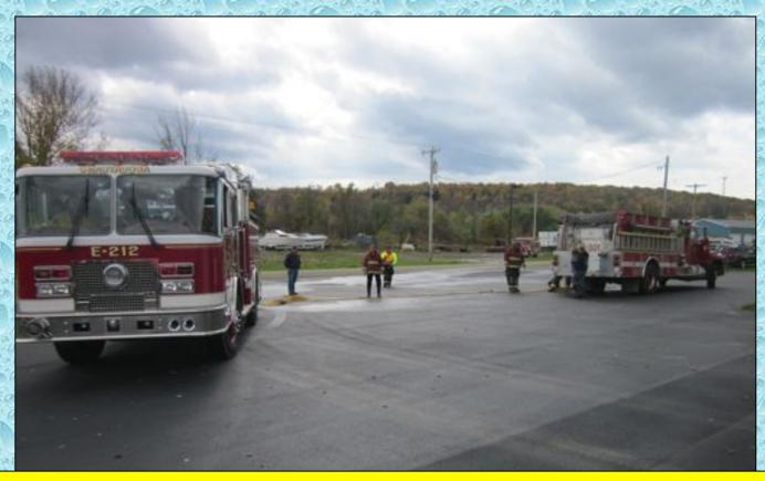
Chautauqua Engine 212 was the first-arriving engine and stopped to lay out a 4-inch supply from the front of the station. Ashville Engine 301 arrived next, "picked up" the line and began getting ready for a dump tank operation.
