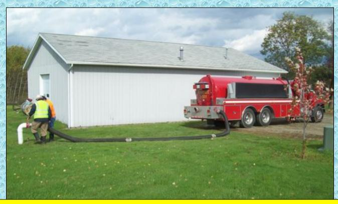
Ashville's 4,200 gallon vacuum tanker (T-301) is shown here self-loading through 30-feet of 6-inch suction hose connected to a 6-inch dry fire hydrant. The vacuum tanker's 500 cfm vacuum pump allows the tanker to load at over 1,000 gpm without the need for an engine crew.
