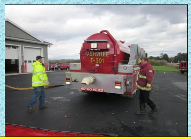
Ashville Tanker 301 arrived with its 4,200 gallons of water and a 4,000 gallon dump tank.
