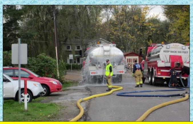
Two loading operations were established – one used 4-inch LDH for those tankers so equipped and the other used dual 3-inch lines supplied by an LDH manifold.
