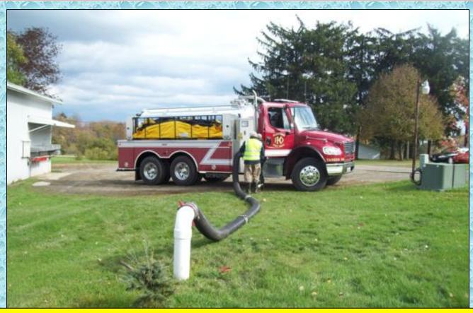
Kiantone's new Firovac 2,700-gallon vacuum tanker also did a fine job of loading using the same suction set-up.
