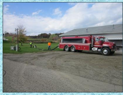
More impressive was the fact that the pond was about 200-feet away from the dry fire hydrant – which meant that the 500 cfm vacuum pump had to pull water through 230 feet of 6-inch conduit.
