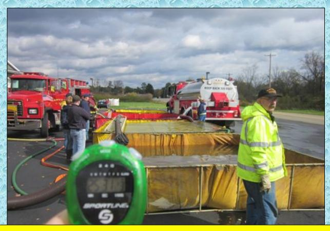
With the flow at 500 gpm and four dump tanks fully in operation at the 25:00 minute mark, things were a "little sparse," in that only one tanker was present at the dump site.
