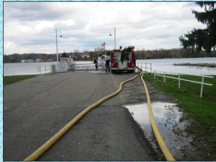
Lake Chautauqua provided an endless source of water at this fill site. Busti Engine 311 (1,500 gpm) took a position at the ferry launch and supported tanker loading operations using 4-inch LDH. One problem that occurred was excessive aquatic debris and vegetation blocking strainers. The pumper crew had to work hard to keep the suction lines free.
