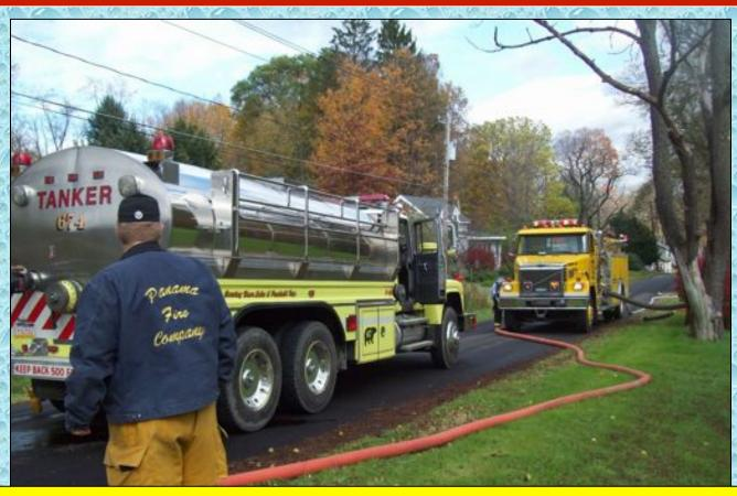
The fill site crew set up to load using a 4-inch LDH line for those tankers equipped to handle such: they also set up to fill using a single, 3-inch line for those tankers that had smaller fill connections.
