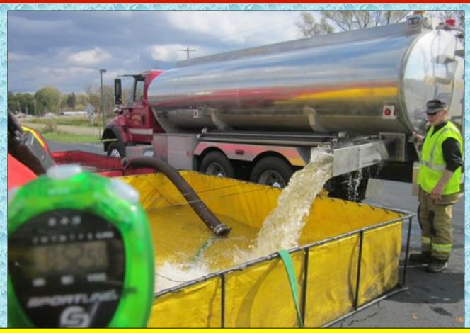
At around the 9:00 minute mark, a second dump tank was placed into service. Chautauqua Tanker 211 is shown here dumping its 4,200 gallons of water.
