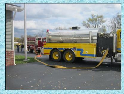
Panama's 3,000-gallon tanker (1,500 gpm pump) was set-up to support the operation as a nurse tanker – however, it was never needed because crews did a really great job of getting the dump site up and running in under 5:00 minutes.
