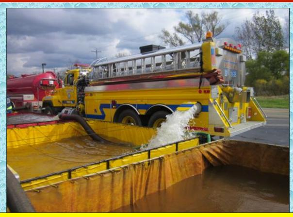
The Water Supply Officer directed Panama's tanker to break from the nurse tanker set-up and move into the shuttle. This move occurred just at the right time and water flow was never interrupted.
