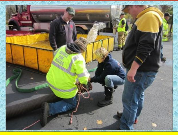
With two dump tanks already in operation, crews work to build another jet siphon in order to move to a three-dump tank operation.
