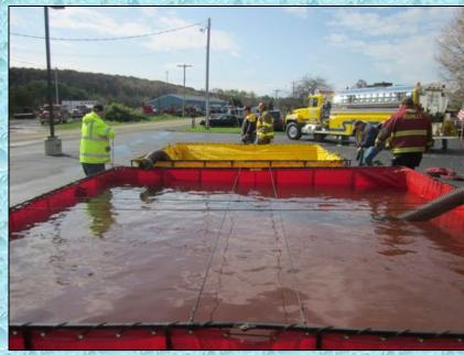
Meanwhile, back at the dump site, Engine 301 was already drafting from the first dump tank! Panama's tanker (yellow) was positioned to serve as a nurse tanker if needed.
