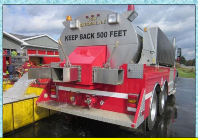
Stanley Hose Tanker 281 arrived as part of the first, tanker task force and is shown here off-loading its 3,000 gallons of water.
