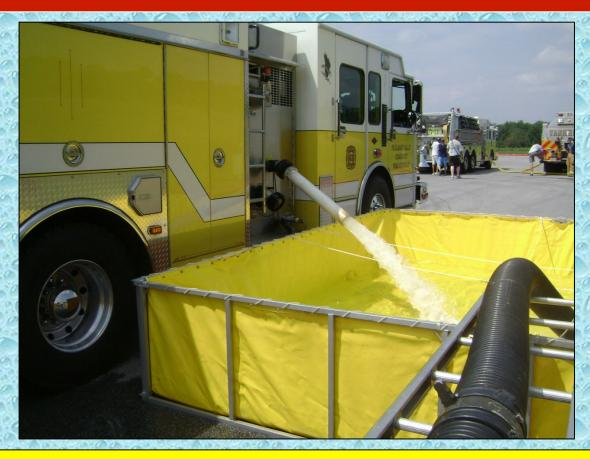
While not ideal for a tanker shuttle operation – water is water. Pleasant Valley Engine 6-3 pumps off its water while awaiting the arrival of more tankers.
