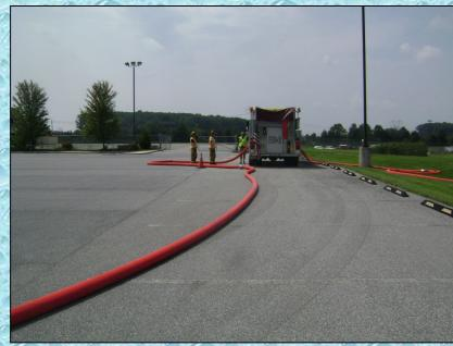
At the 5:00 minute mark, water flow is started at 250 gpm from Engine 6-2 while ET19 supports the flow through nurse tanker operations.
