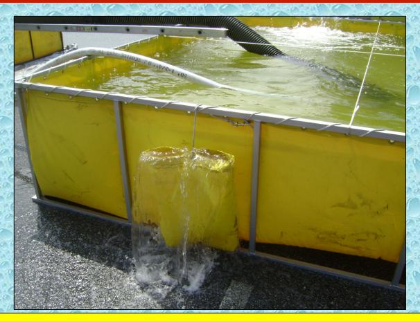
It is important to secure the drains on dump tanks. While it is unlikely that the entire contents will be lost, this does make a huge mess in bad weather. When possible, tie the drains up on the inside of the tank.
