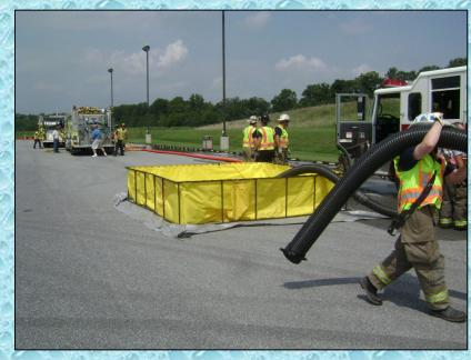
Gettysburg Engine 1-2 arrives and also supports the fire attack using the LDH manifold while the dump site awaits the arrival of a tanker.
