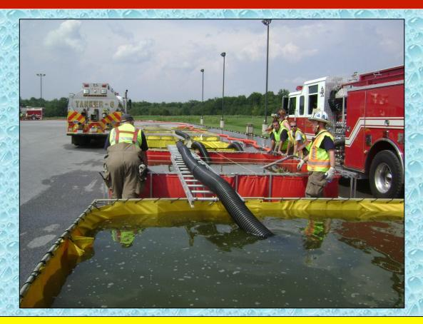
With the flow now at 1,000 gpm, the four-tank, dump site operation provides adequate support.
