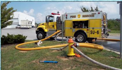
Pleasant Valley Special Unit 6 (1500 gpm) was used to establish the second fill station at a fire hydrant. The crew did a nice job of accessing the available water from the hydrant.
