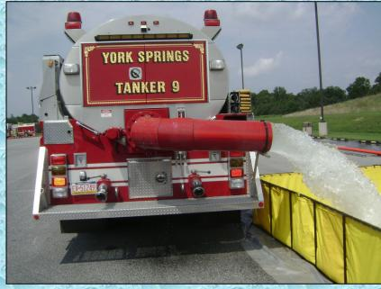
Tanker 9 dumps its water and the transition to a dump site operation begins at 16:58 minutes.
