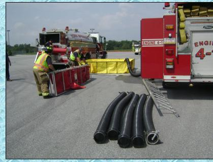
At the 13:30-minute mark, York Springs Tanker 9 arrives as the first tanker on the Tanker Task Force and prepares to offload its water. The dump site crews also grab extra equipment and begin setting up a second dump tank.
