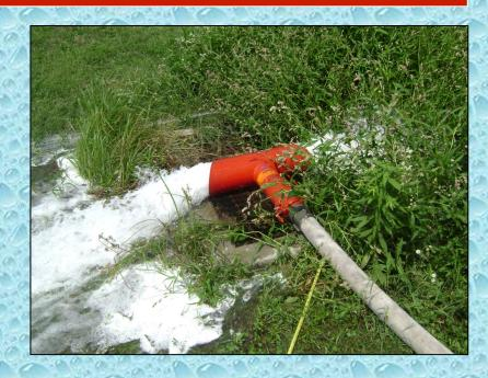
A Hose Monster equipped with a fixed pitot tube was used to measure the flow during the drill.
