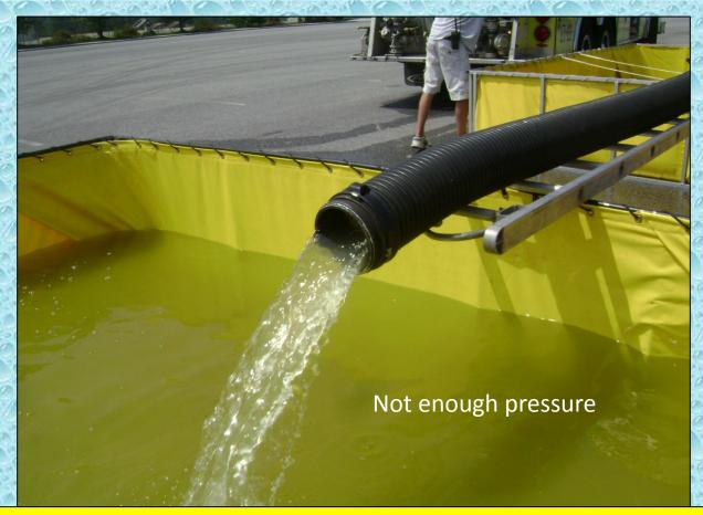
When pumping a jet siphon, pump enough pressure so that a solid stream of water is discharged from the end of the suction hose.
