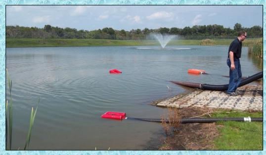
The Jarrettsville crew sets up three suction lines so that they can maximize their pumper's flow capacity.
