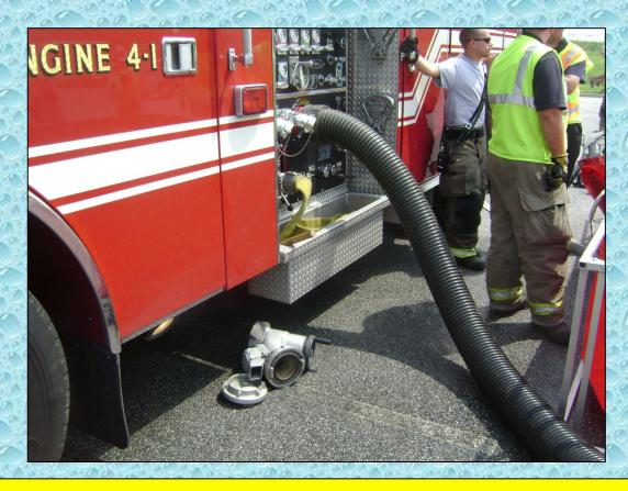
One problem that arose at the dump site was that Cashtown Engine 4-1 was not equipped with a control valve on its suction inlet which meant that is could not pump its 1,000 gallons of water to the attack engine.
