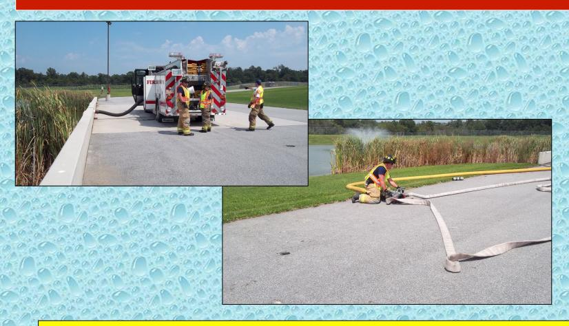
Fairfield Engine/Rescue 2 sets up a second fill site at the same pond thus allowing two tankers to be filled independently.
