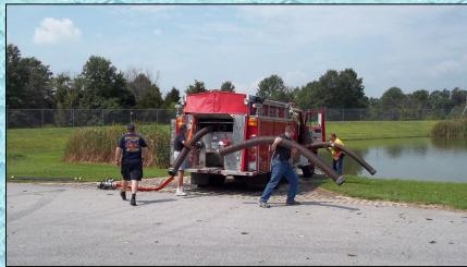
Jarrettsville Special Unit 781 (1500 gpm) arrives at the pond and begins work on setting up a tanker fill site. The pond was located on the grounds of the training center – so the travel route for tankers was adjusted to add some distance.
