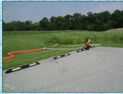
In hopes of delivering 1,000 gpm, a 5-inch line is stretched to the flow measuring device.
