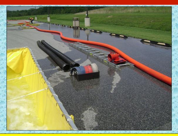
At the 19:00-minute mark, flow was increased to 504 gpm as more equipment is brought in to expand the dump site.
