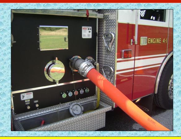
Choosing the right discharge is critical when moving to larger flow volumes. The high-flow discharge shown in use above is able to easily support the 1,000-gpm flow at this drill.
