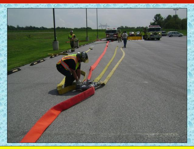
Meanwhile, an LDH manifold is placed in-line in order to facilitate nurse tanker operations if needed.
