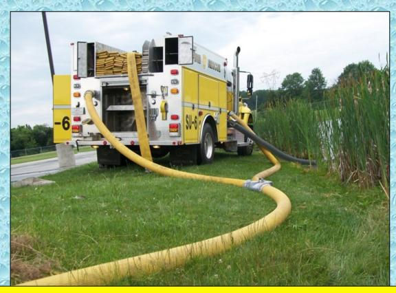
Special Unit 6 maximizes its output by using dual suctions and dual, 5-inch discharges. The 1500 gpm unit easily flowed more than 2,000 gpm using this configuration.
