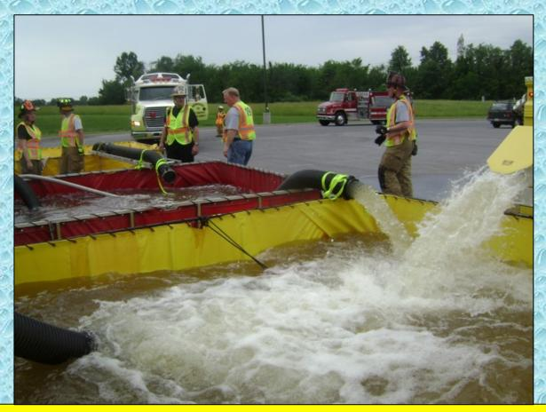
With three dump tanks in use, the transfer of water between the tanks becomes critical to the success of the operation.
