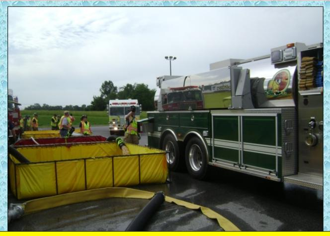
A third dump tank is placed and flow is moved to 524 gpm at the 19:00-minute mark.
