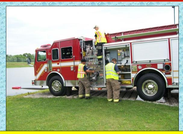
With the suction hose now in place, the crew works on deploying a hose line for running the fill station.
