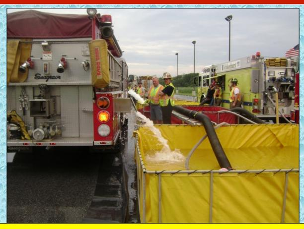
SAVES Engine Tanker 29 is shown here just starting to offload its water. Note the ladder used to help space out the dump tanks – this allows more room for larger tankers to offload simultaneously.
