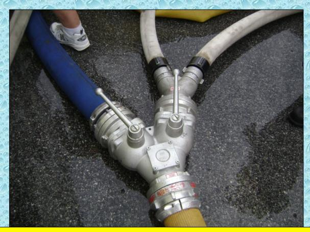
In an effort to improve again, three discharges were used to feed the jumbo wye – however, two had to be reduced to 3-inch lines. This allowed the pumper to produce the same flow with less effort.
