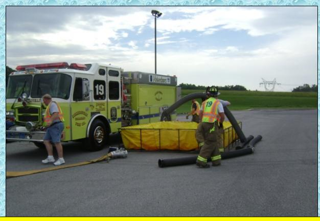
Meanwhile, at the dump site, ET19's crew hustles to get the first dump tank (2100 gallons) set-up and ready for the arrival of tankers. This feat is accomplished at the 4:00-minute mark.
