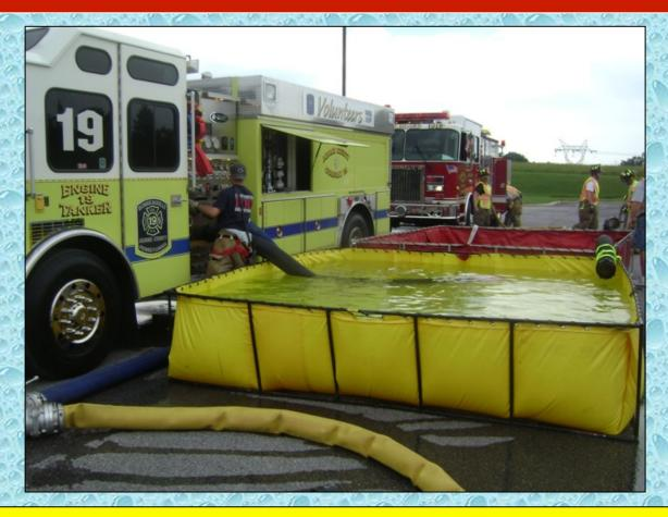
With the primary dump tank now full, the operation begins transitioning from a nurse tanker operation to a dump tank operation.
