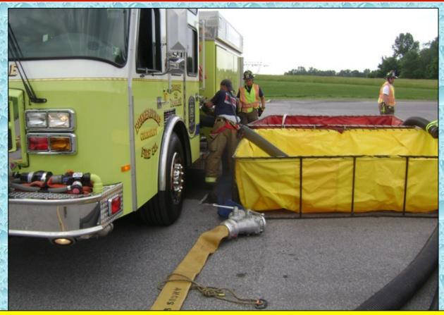
The dump site engine works to set-up for a drafting operation. The 1750 gpm pumper intends to use 5-inch hose to feed one side of a 5"x5"x5" "jumbo" gated wye.
