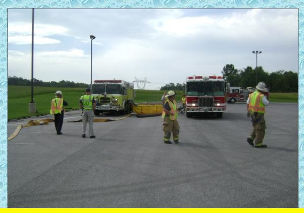
Fountaindale ET3 (1800 gallons) is the first tanker to arrive on the scene. With the 5-minute mark not yet reached, a decision must be made whether to dump the tanker or use the tanker in a nurse tanker mode.
