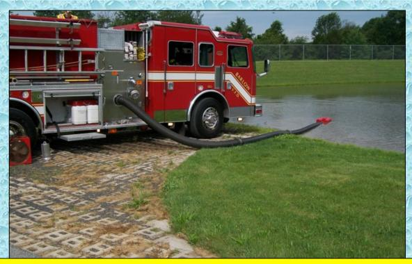
30-feet of suction hose was used to access a deeper part of the pond. This again reinforces the importance of carrying more than the traditional 20-ft of suction hose on a pumper. Rural pumpers should carry 30 or 40-ft of suction hose so that then can have better access to draft sites in their response districts.
