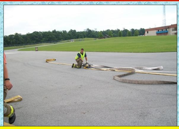
A 5-inch hose line is stretched and an LDH manifold is connected so that the filling operations can be controlled near the tankers – not at the pump panel of the fill site engine.
