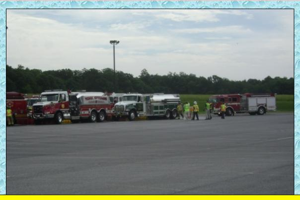
Tankers line up to offload water. One issue that did arise was that the larger tankers could not dump their load into just one dump tank because all four dump tanks were either 2,500 gallons or smaller. This was not a major issue at this drill, but is certainly something to consider when using large tankers.
