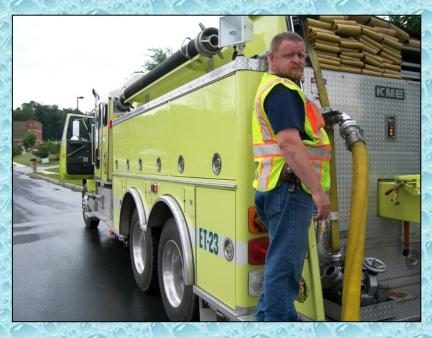
Greenmount's Engine Tanker 23 (1500 gallons) is shown above being filled by the Cashtown pumper at the hydrant fill site.
