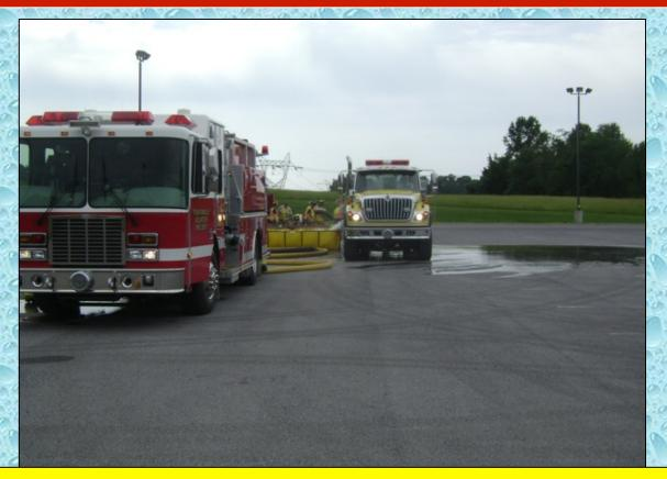
Pleasant Valley Tanker 6 (3200 gallons) was one of the first, large tankers to arrive. The tanker is shown above offloading its water into the primary dump tank.
