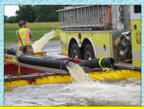
Once again – an excellent photo showing what the stream from a jet siphon should look like. In terms of operating pressure – there is no exact number – just pump the siphon until the flow looks like the photo above.
