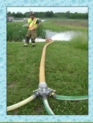
At the 71:00 minute mark, operations had stabilized and the flow was moved to 750 gpm and then again to 794 gpm at 80:00 minutes - where it was sustained for the remainder of the drill.
