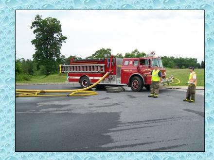
One note for improvement would be to have used some type of siamese or manifold instead of connecting the 5-inch hose to a single, 2-1/2-inch discharge. Because E43 is an older pumper, it did not have a high-flow discharge — to correct that problem, simply pump from two discharges into one 5-inch line. In this case, dual 3-inch lines into a 5-inch line would most likely have improved their output ability.
