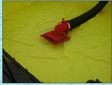
ET19 does not have a control valve on its driver's side suction inlet. Thus, when trying to pump to the attack engine using onboard water, much of the water back feeds through the suction hose into the dump tank. Without some type of control valve on your suction inlet, it is difficult to use onboard tank water and set up for drafting at the same time.
