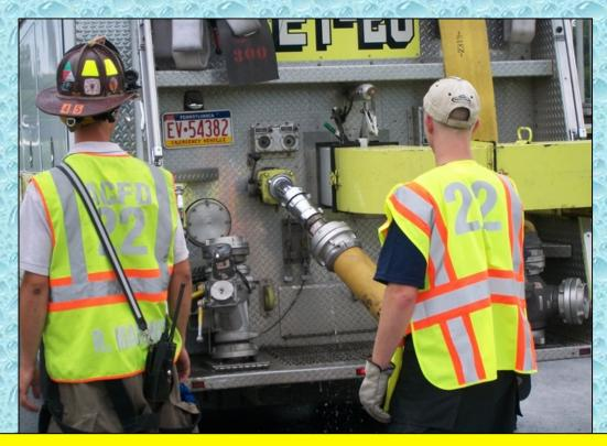
Even though a tanker may have a smaller fill line, LDH can still be used. The advantage in using LDH is that friction loss is minimized between the pumper and the tanker fill valve. Littlestown ET20 is shown above being filled using 5-inch hose.
