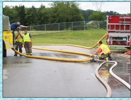
Pleasant Valley Tanker 6 (3200 gallons) is filled using a 5-inch fill hose – a much faster operation than the dual, 3-inch line scenarios.
