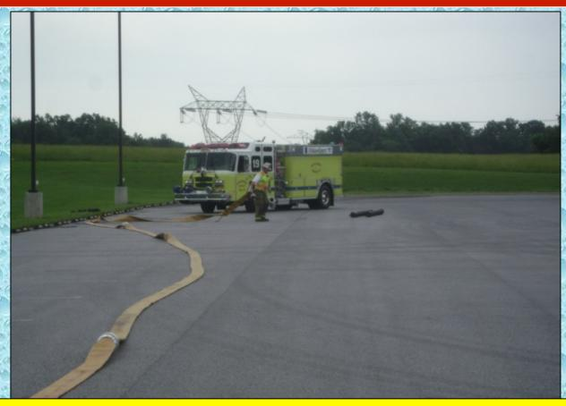
ET19 positions and begins setting up for a dump tank operation. The intent is to be ready to support the attack engine as soon as possible.
