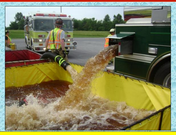
Water transfer operations are begun – the jet siphon above is a good example of what the flow should look like when the device is properly pressurized.
