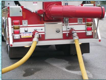
York Springs' tanker (2600 gallons) is shown above being filled using two different fill arrangements. As proven before, the use of LDH can shave valuable seconds/minutes off of a tanker's fill time – which translates to possibly one or two more loads of water that can be hauled in the 2-hour ISO test.
