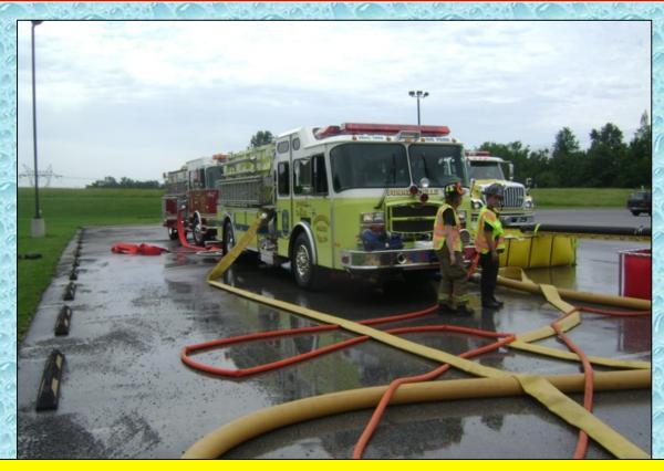
In hopes of increasing the operation to 1000 gpm, the decision is made to feed the jumbo wye with two, 5-inch lines so that the flow can be fed using two discharges on the pumper instead of just one.
