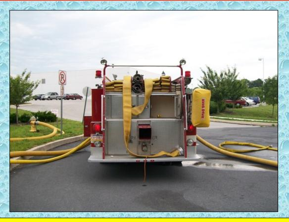
Engine 43's use of LDH allowed it to operate as a fill site pumper with little difficulty.
