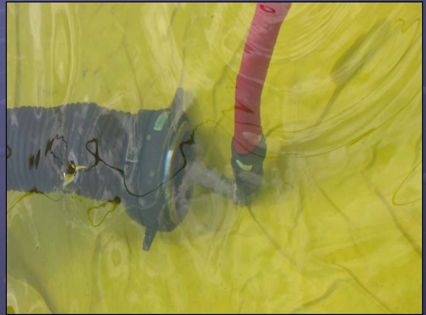
A "home made" jet siphon.
