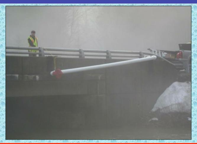
When ready to deploy, one person can lower the arm using a mechanical advantage raising/lowering system.
