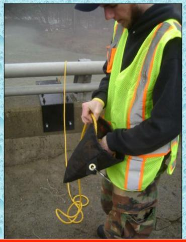
The retrieval system uses polypropylene rope for weather resistance and the rope is stored in a small, mesh stuff sack.
