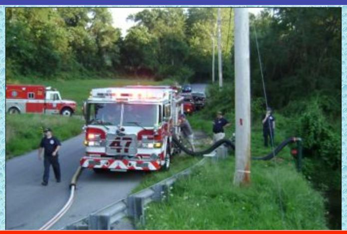
Once deployed by a two-person crew, the standpipe flowed 1,000 gpm+ when connected to this 1,500 gpm pumper.
