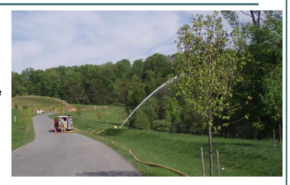
The most flow that was obtained from RE709B in the first evolution was around 830 gpm (50 psi out of a 2" tip).
