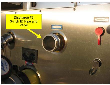
Rear Discharge Specifications (Labeled as "Rear Discharge" on pump panel)
